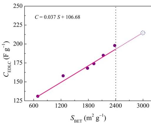
**Fig. S7** The relationship between surface areas and  $C_{\text{EDLC}}$  of HPC electrodes.
