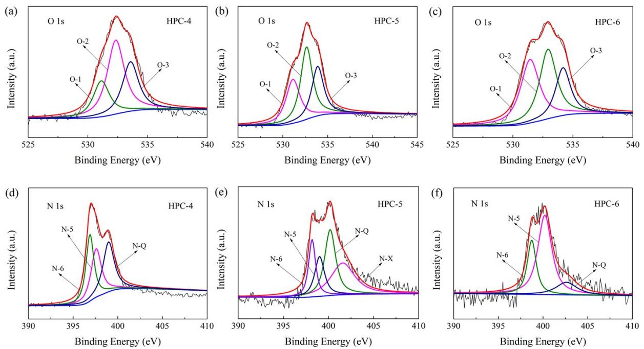
**Fig. S2** High-resolution XPS spectra of O 1s (a–c) and N 1s (d–f) for HPC-4 (a, d), HPC-5 (b, e) and HPC-6 (c, f) prepared at different activation temperatures.
