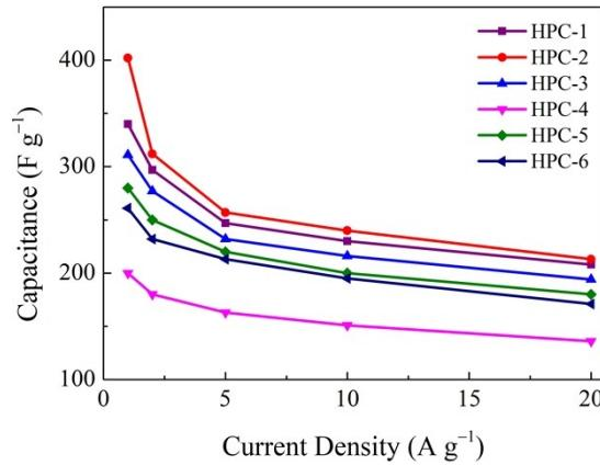
**Fig. S6** Specific capacitances of HPC electrodes at different current densities.
