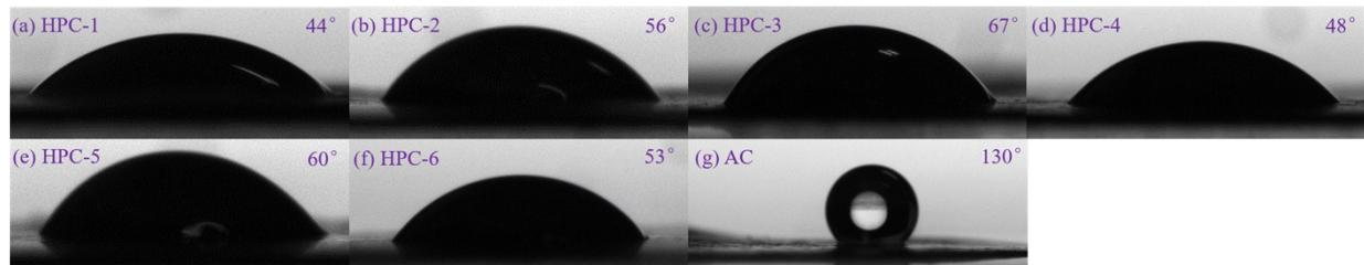
**Fig. S3** The water contact angles of HPC (a–f) and commercial activated carbon (AC, g).
