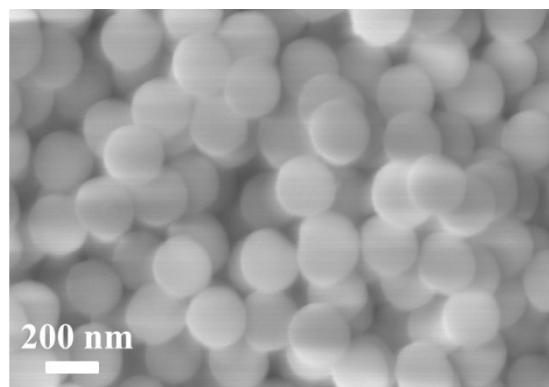
**Fig. S1** SEM image of  $\text{SiO}_2$ .
