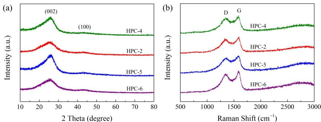
**Fig. S4** XRD patterns (a) and Raman spectra (b) of HPC.
