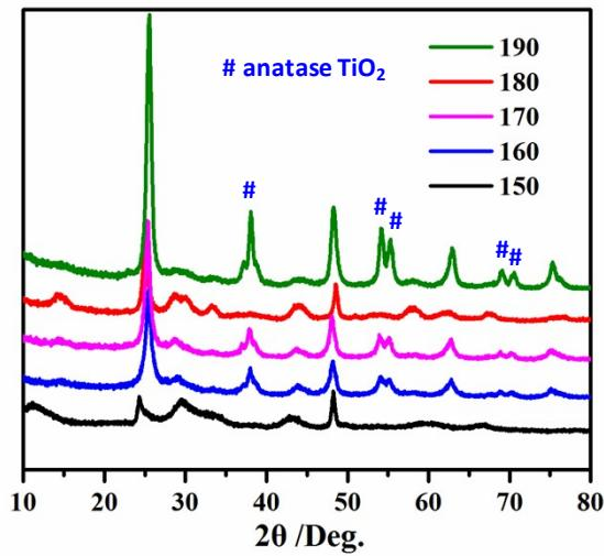
Fig. S3 XRD pattern of  $\text{TiO}_2$  derived from titanate with different reaction times.
