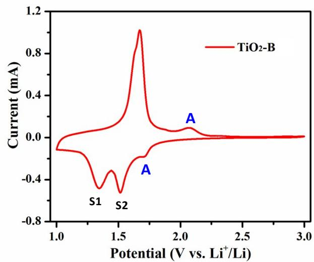
Fig. S4 CV curve of  $\text{TiO}_2\text{-B}$ .
