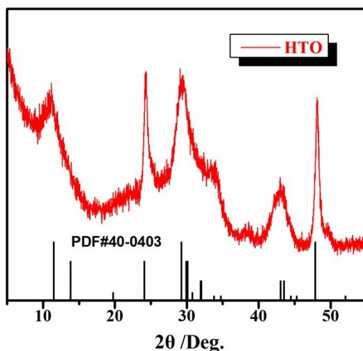
Fig. S1 XRD pattern of HTO nanowires precursor.
