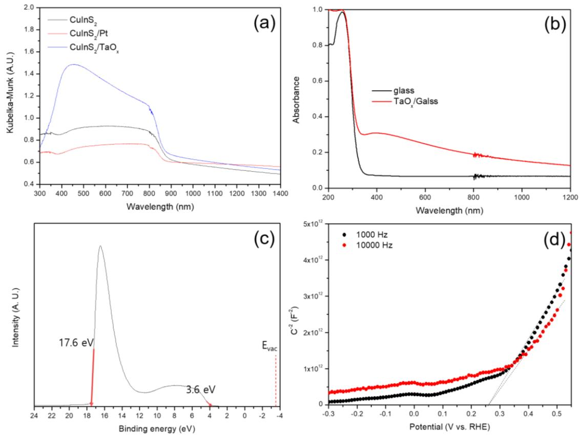
**Fig. S8.** (a) Kubelka-Munk absorption spectra of photocathodes (b) absorbance of TaO<sub>x</sub> deposited on glass (c) UPS result of TaO<sub>x</sub> deposited on CuInS<sub>2</sub> (d) Mott-Schottky plot of TaO<sub>x</sub>
