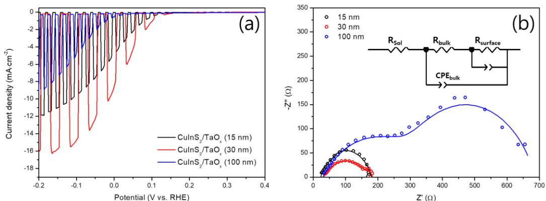
**Fig. S7.** LSV (a) and Nyquist plots (b) of CuInS<sub>2</sub>/TaO<sub>x</sub> films depending on the thickness at -0.2 V vs. Ag/AgCl.
