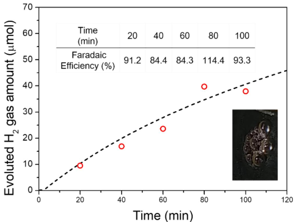
**Fig. S10.** Evolved H<sub>2</sub> gas measurement for a CuInS<sub>2</sub>/TaO<sub>x</sub> photocathode during chronoamperometry. Inset photograph shows the bubble coalescence of H<sub>2</sub> gas during the photoelectrochemical reaction.
