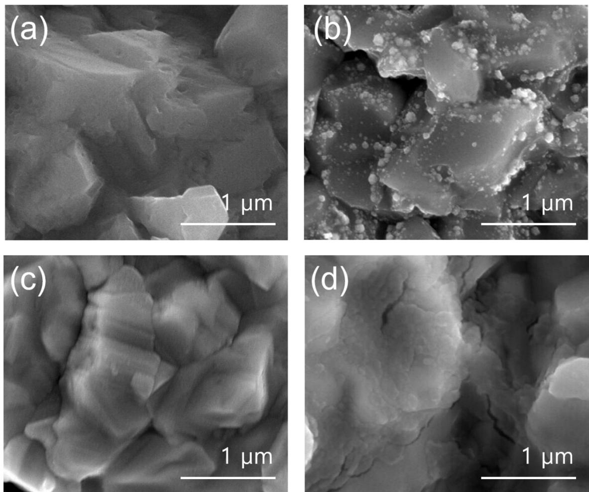
**Fig. S3.** SEM images of (a) CuInS<sub>2</sub>. (b) CuInS<sub>2</sub>/Pt (c) CuInS<sub>2</sub>/TaO<sub>x</sub> (as prepared) (d) CuInS<sub>2</sub>/TaO<sub>x</sub> (activated)
