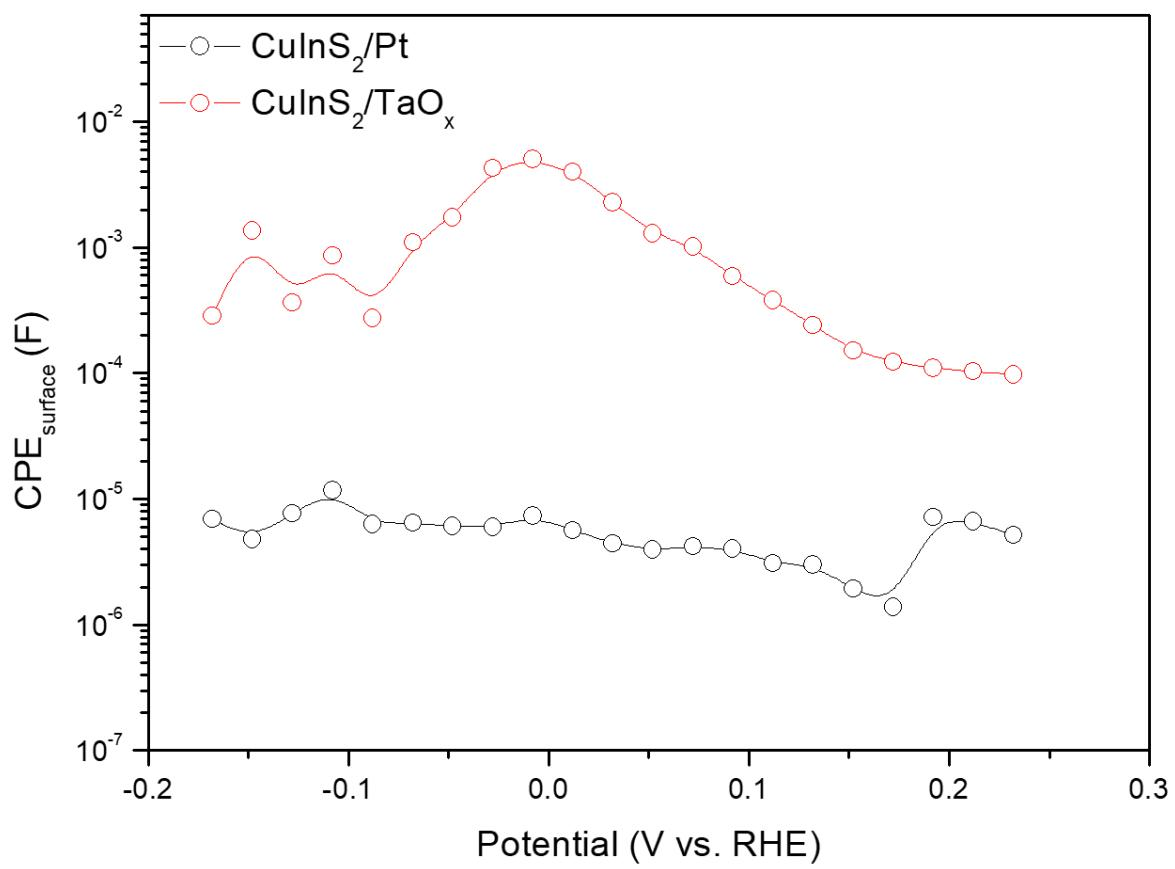
**Fig. S6.** Capacitance of surfaces for CuInS<sub>2</sub>/Pt and CuInS<sub>2</sub>/TaO<sub>x</sub>
