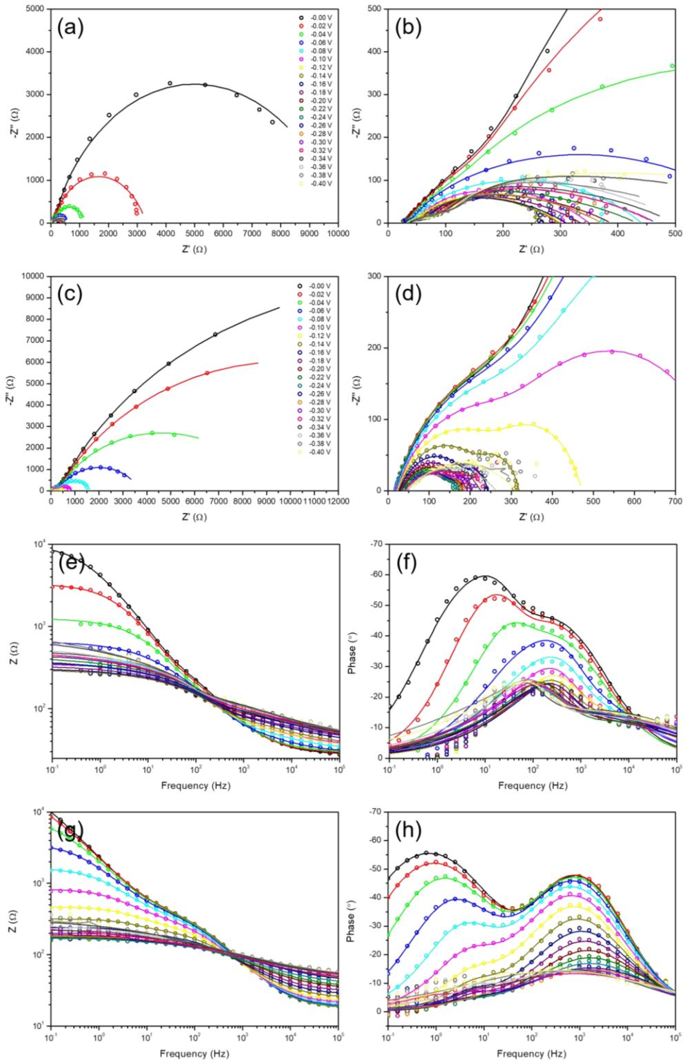
**Fig. S5.** Nyquist plots of electrochemical impedance spectroscopy results for CuInS<sub>2</sub>/Pt ((a), (b)) and CuInS<sub>2</sub>/TaO<sub>x</sub> ((c), (d)) on a different scale. Bode plots of electrochemical impedance spectroscopy for CuInS<sub>2</sub>/Pt ((e), (f)) and CuInS<sub>2</sub>/TaO<sub>x</sub> ((g), (h)) on a different scale. The dotted data is obtained from experiments and the solid lines indicate the fitted results.
