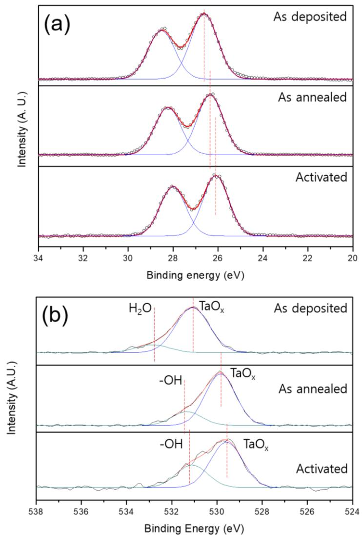
**Fig. S1.** XPS spectra of  $\text{CuInS}_2/\text{TaO}_x$  with different conditions (a) Ta 4f and (b) O 1 s
