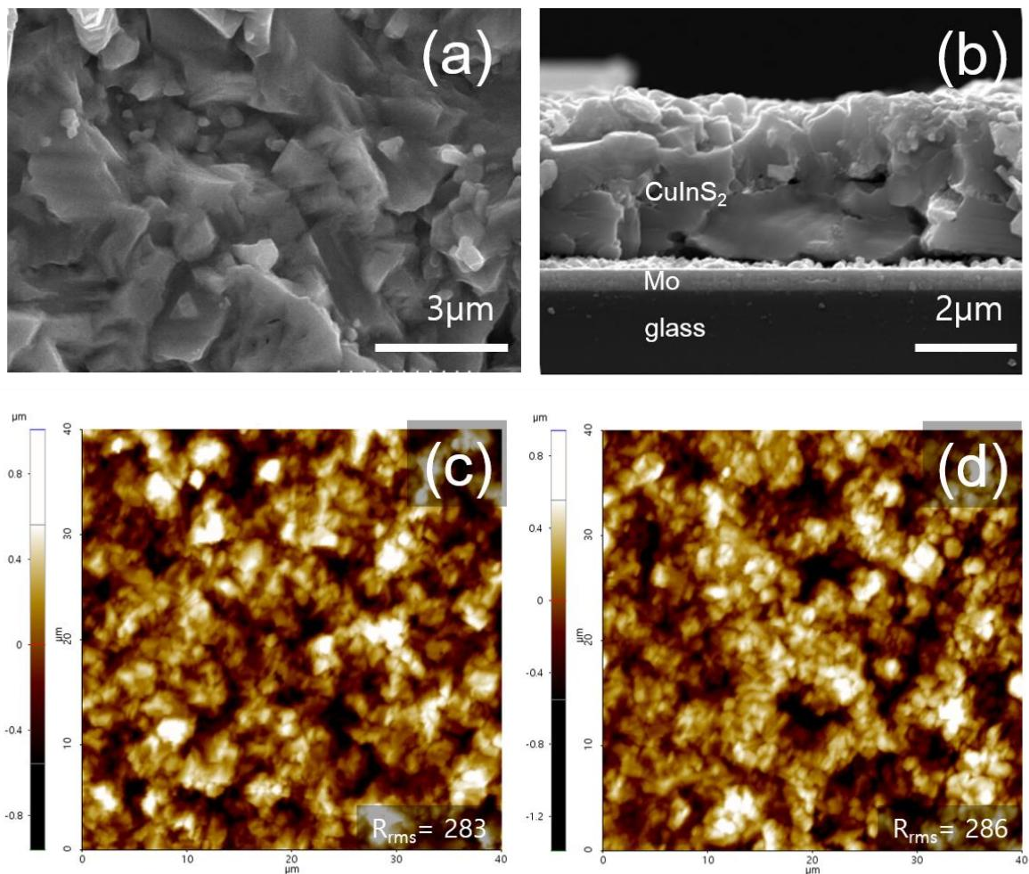
**Fig. S2.** SEM images of (a) top view and (b) cross-section of CuInS<sub>2</sub>. AFM topography images of CuInS<sub>2</sub>/TaO<sub>x</sub> (c) as deposited and (d) activated samples.
