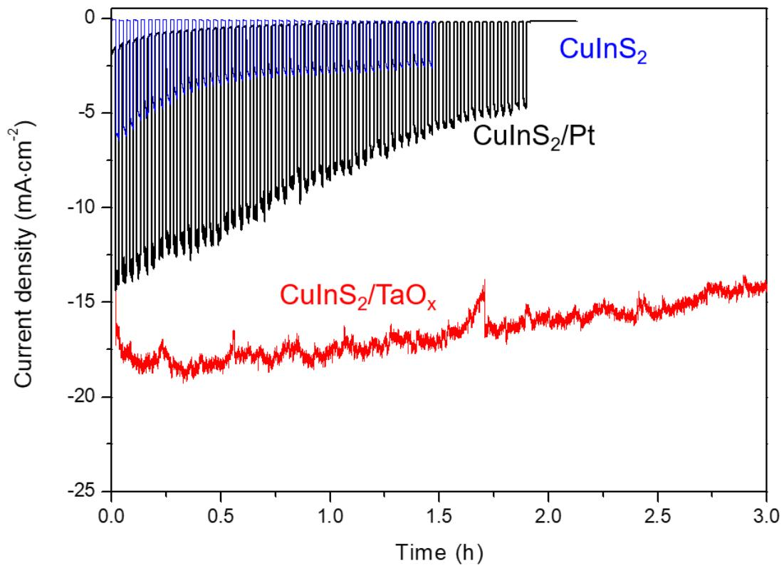
**Fig. S9.** Chronoamperometry results of  $\text{CuInS}_2$ ,  $\text{CuInS}_2/\text{Pt}$ , and  $\text{CuInS}_2/\text{TaO}_x$  photocathodes under light illumination.
