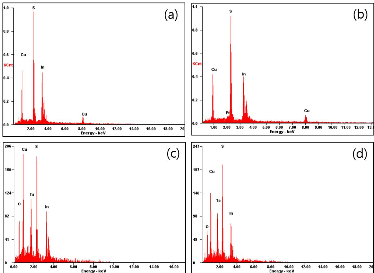
**Fig. S4.** EDS spectra of (a) CuInS<sub>2</sub>. (b) CuInS<sub>2</sub>/Pt (c) CuInS<sub>2</sub>/TaO<sub>x</sub> (as prepared) (d) CuInS<sub>2</sub>/TaO<sub>x</sub> (activated)
