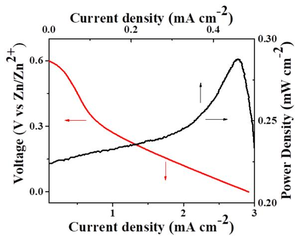
**Figure S13.** The Polarization and power density curves of rechargeable Zn-CO<sub>2</sub> batteries with NiPG as cathode.
