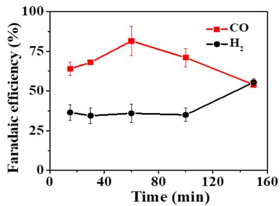
**Figure S15.** CO and H<sub>2</sub> FEs of Zn-CO<sub>2</sub> batteries at discharge current of 0.5 mA.
