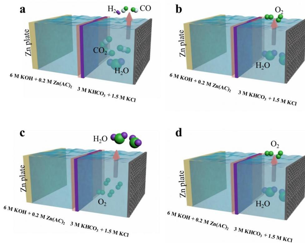
**Figure S12.** The scheme of aqueous rechargeable dual-model battery device. Zn CO<sub>2</sub> battery mode of (a) discharge and (b) charge process. Zn O<sub>2</sub> battery model of (c) discharge and (d) charge process.
