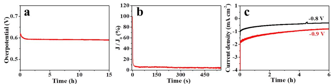
**Figure S11.** Electrocatalytic durability on NiPG in neutral solution. (a) OER and (b) ORR in 3 M  $\text{KHCO}_3$  including 1.5 M KCl solution, and (c) CDRR in 0.1 M  $\text{KHCO}_3$  solution, respectively.
