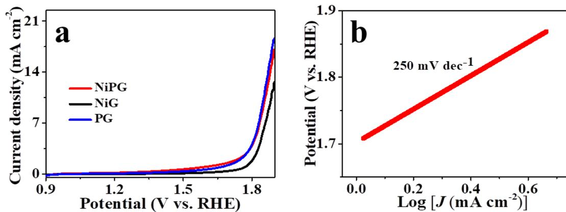
**Figure S5.** Neutral OER performance on NiPG, NiG and PG. (a) Neutral OER LSV curve and (b) Tafel slope of NiPG. Electrolyte: 3 M KHCO<sub>3</sub> solution including 1.5 M KCl.
