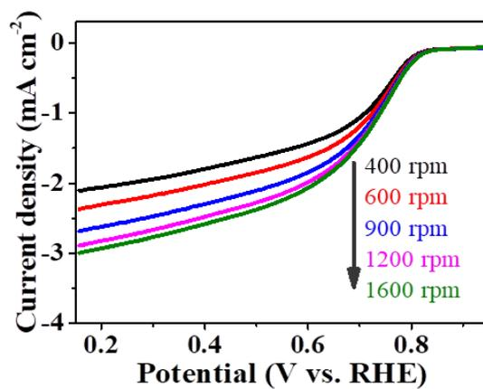
**Figure S6.** ORR LSV curves on NiPG at a series of rotating speeds. Electrolyte: 0.1 M KOH solution.
