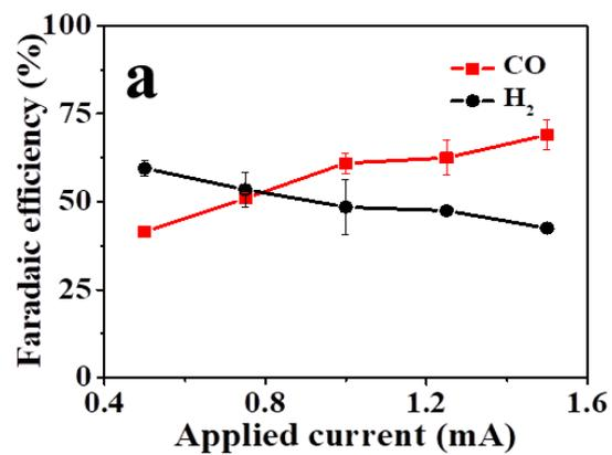
**Figure S14.** CO and H<sub>2</sub> FEs of Zn-CO<sub>2</sub> batteries with error bar at a series of discharge currents.
