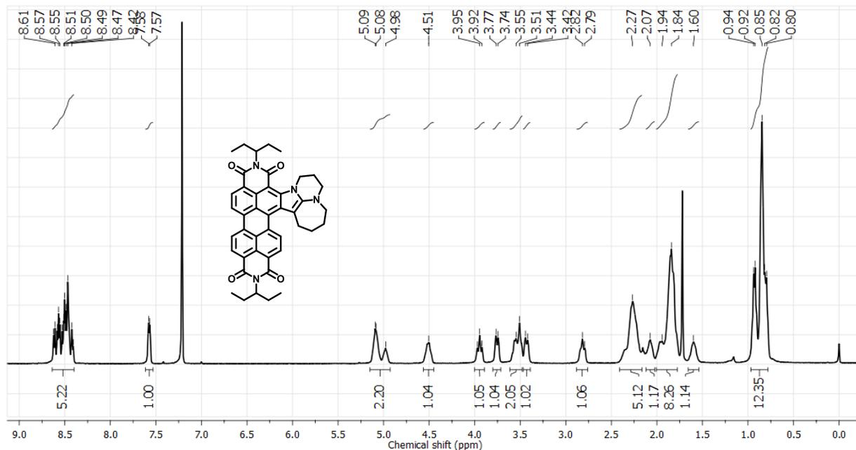
Figure S3:  $^1\text{H}$  NMR spectrum of PDIDBU in  $\text{CDCl}_3$  (500 MHz).
