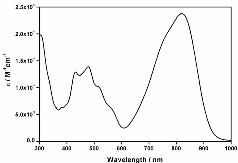
Figure S1. Absorption spectra of PDIDBU in chloroform ( $10^{-6}$  M) solution.
