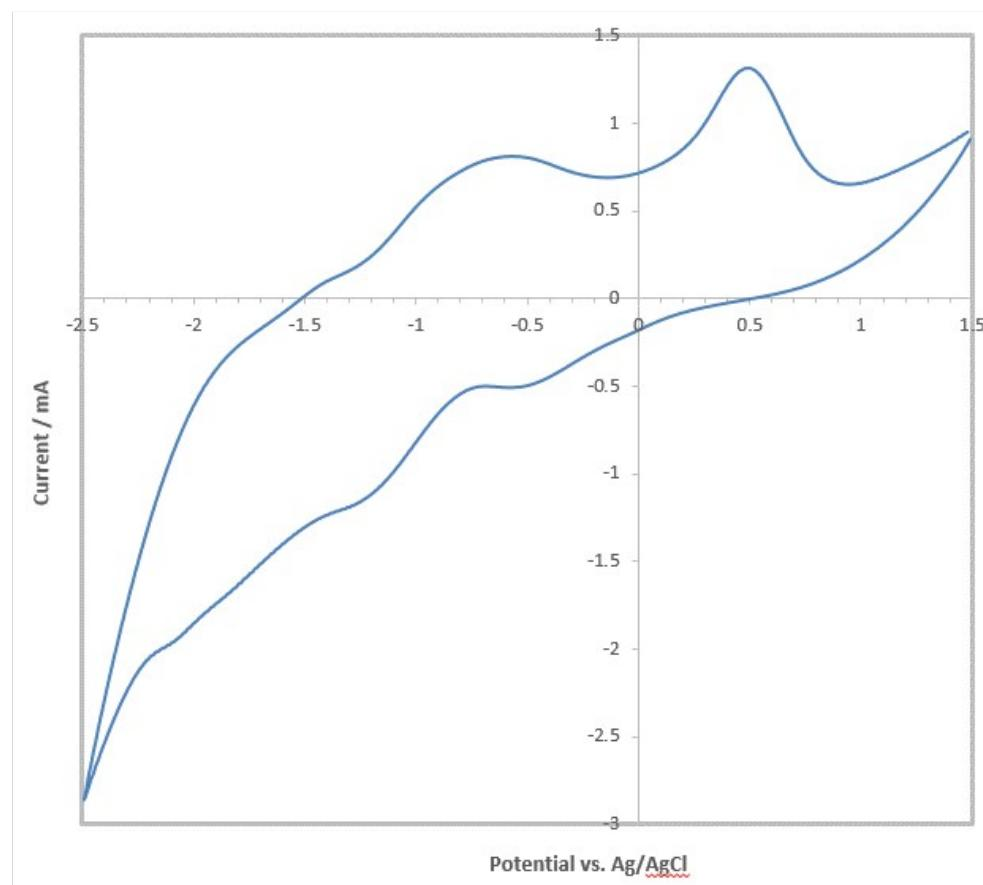
**Figure S4.** Cyclic voltammogram for  $\text{Bi}_{13}\text{S}_{18}\text{I}_2$  thin film sample on mesoporous titania at scan rate of 0.1 V/s
