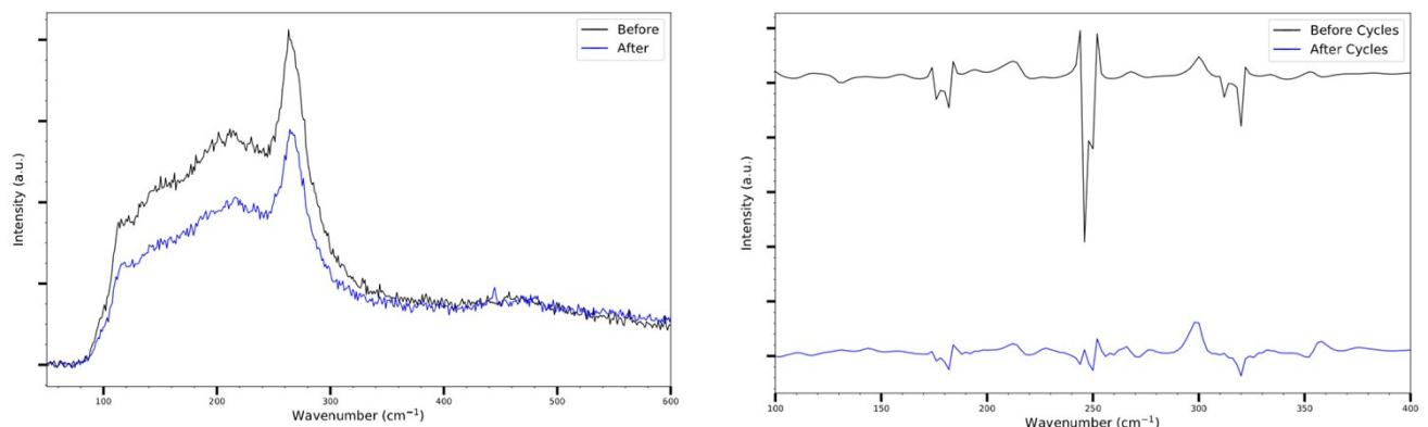
**Figure S9.** Raman (a) and IR (b) spectra (shifted vertically for clarity) of  $\text{Bi}_{13}\text{S}_{18}\text{I}_2$  as electrode material deposited on carbon cloth, compared before and after conducting 5000 cycles of stability test.
