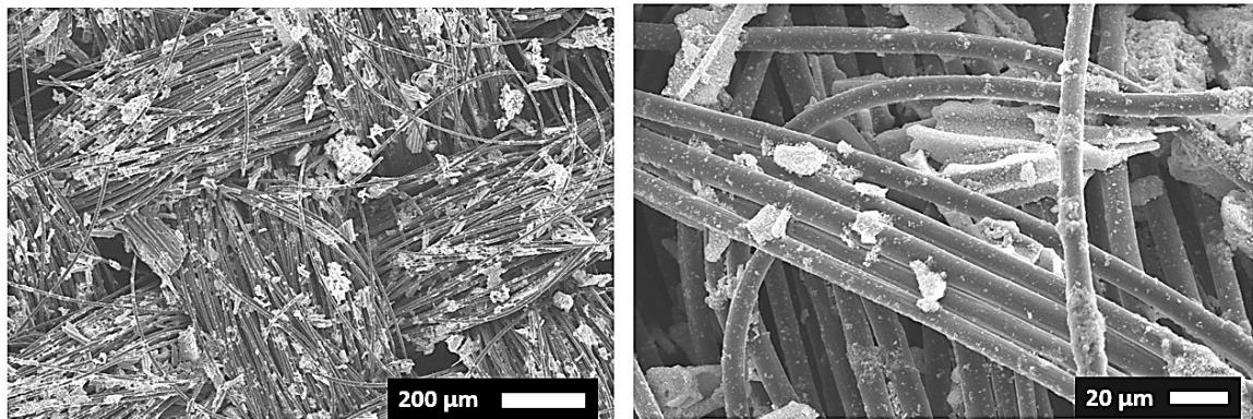
**Figure S7.** SEM images of  $\text{Bi}_{13}\text{S}_{18}\text{I}_2$  electrode prepared from suspension-deposited method
