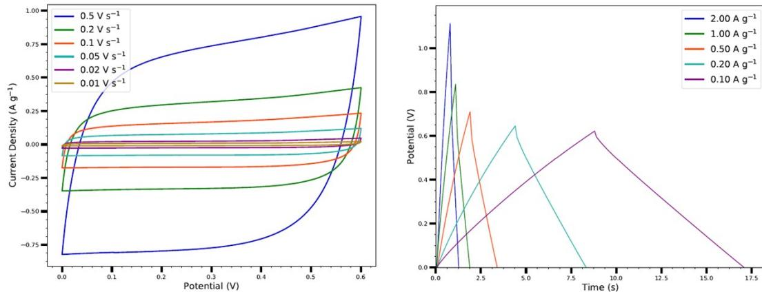
**Figure S6** Cyclic voltammograms at varying scan rates (a) and Galvanostatic charge–discharge curves at different constant current (b) of the controlled suspension-deposited Bi<sub>13</sub>S<sub>18</sub>I<sub>2</sub>-based EDLC.
