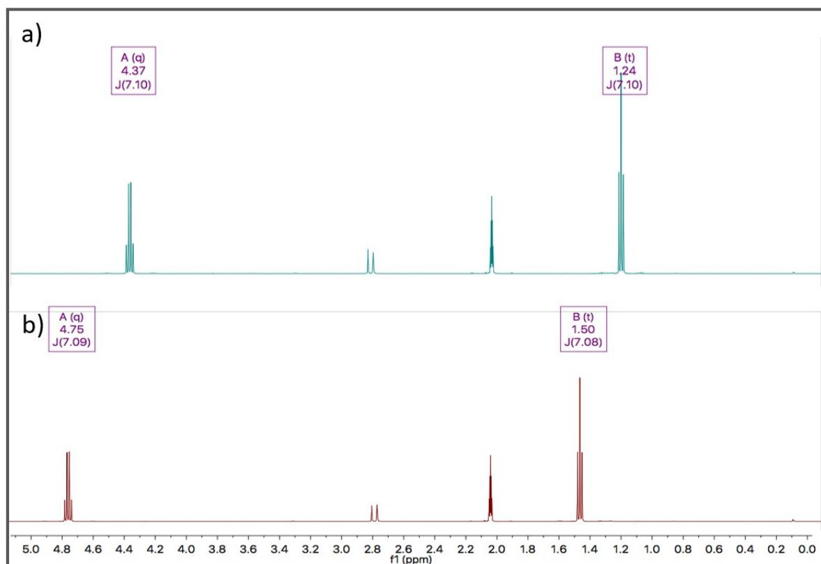
**Figure S1.** <sup>1</sup>H NMR spectra for (a)  $\text{KS}_2\text{COC}_2\text{H}_3$  and (b)  $\text{Bi}(\text{S}_2\text{COC}_2\text{H}_5)_3$  in deuterated acetone. The additional peaks at 2.0 and 2.8 ppm were identified in literature as  $\text{H}_2\text{O}$  and acetone impurities.<sup>42</sup>
