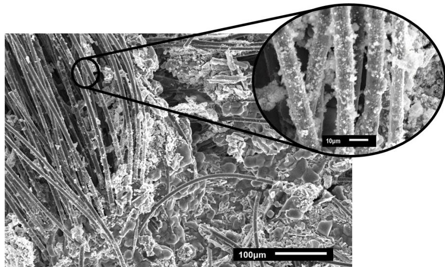
**Figure S8.** SEM images of  $\text{Bi}_{13}\text{S}_{18}\text{I}_2$  electrode after 5000 cycles, with spread-out coverage of active material on carbon fibres. The area with smooth surface coverage indicated the coating from  $\text{NaClO}_4$  electrolyte.
