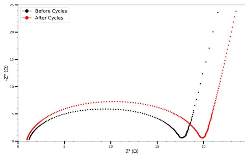
**Figure S11.** Nyquist plot of  $\text{Bi}_{13}\text{S}_{18}\text{I}_2$  EDLC before (black) and after (red) 5000 cycles.
