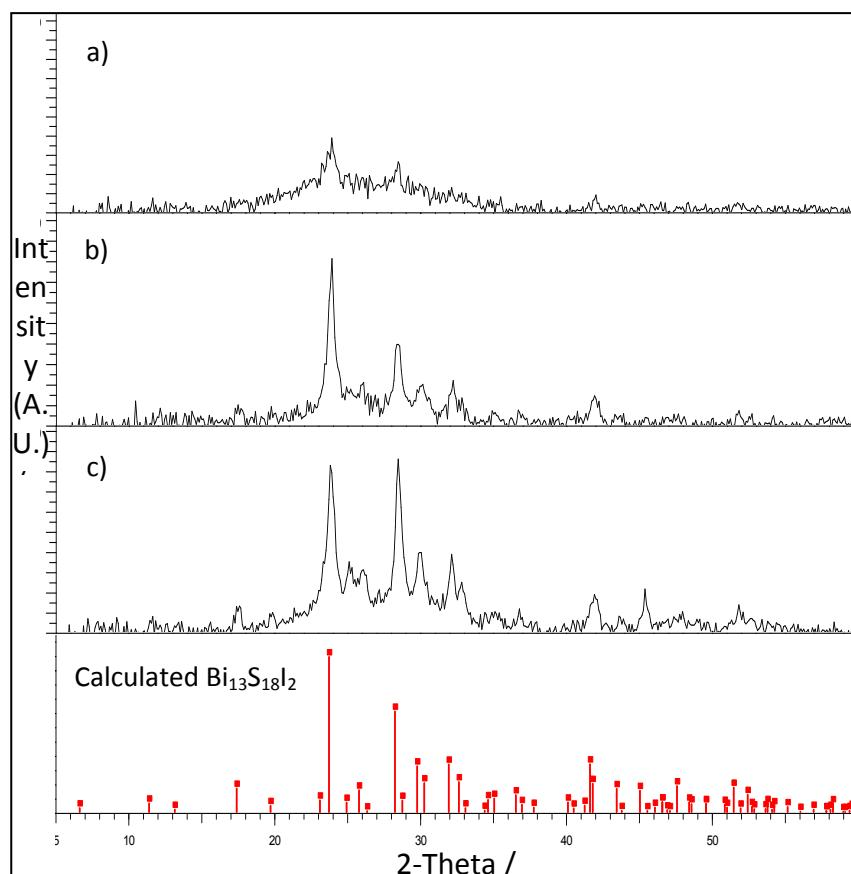
**Figure S3.** XRD spectra for a thin film comprised of (a) 1 layer, (b) 3 layers, and (c) 5 layers
