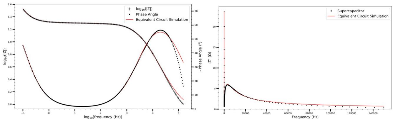
**Figure S10.** Bode plot (a) and frequency versus out of phase component plot (b) showing both experimental (black) and simulated from equivalent circuit (red).
