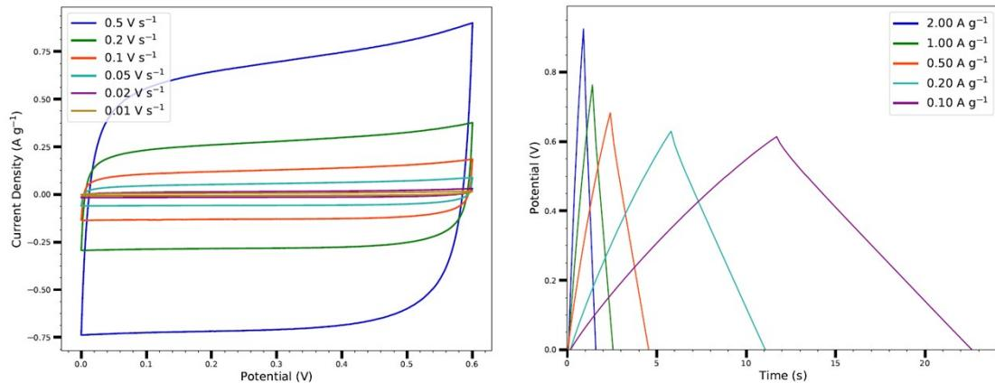
**Figure S5.** Cyclic voltammograms of the control blank EDLC without active material at varying scan rates. d) Galvanostatic charge–discharge curves of a control blank EDLC device.
