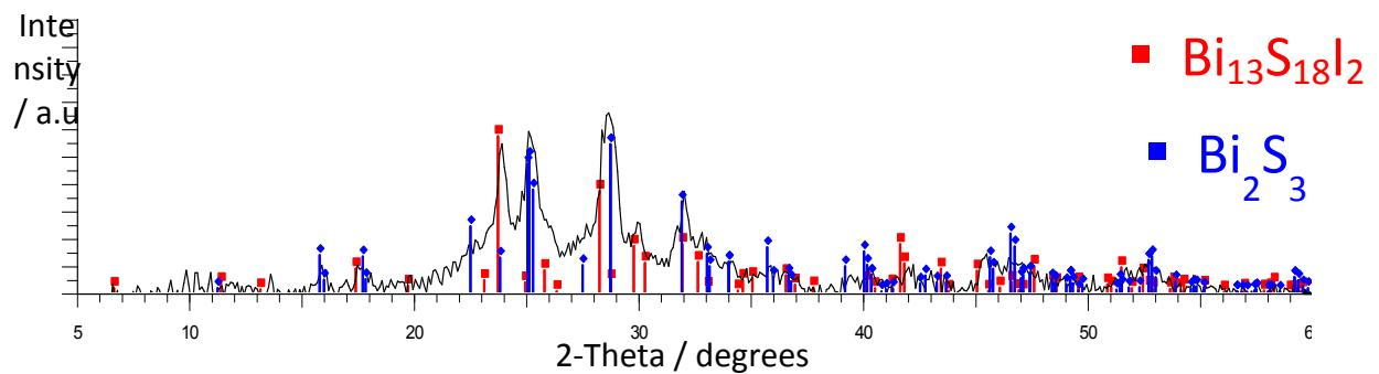
**Figure S2.** XRD spectra for a thin film synthesized from a precursor solution with a 26:1  $\text{Bi}(\text{xt})_3:\text{BiI}_3$  ratio, showing patterns corresponding to a mixture of  $\text{Bi}_{13}\text{S}_{18}\text{I}_2$  and  $\text{Bi}_2\text{S}_3$ .
