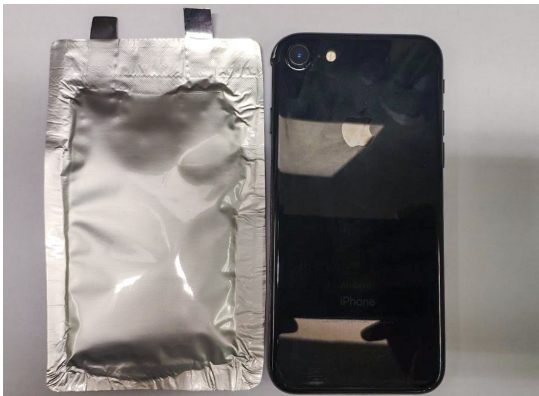
Figure S4 Assembled 3D printed graphene/nickel supercapacitor in punch cell style, with size comparing to an iPhone 7.
