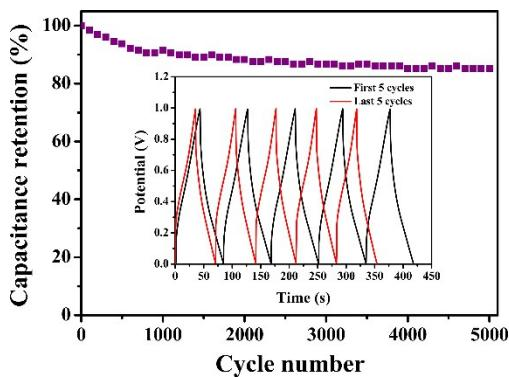
**Fig. S19.** Cycling stability of Lig/PANI/FGH/FCC-based all-solid-state supercapacitor at a current density of  $20\text{ mA cm}^{-2}$ . The inset shows the GCD curves of first 5 cycles
