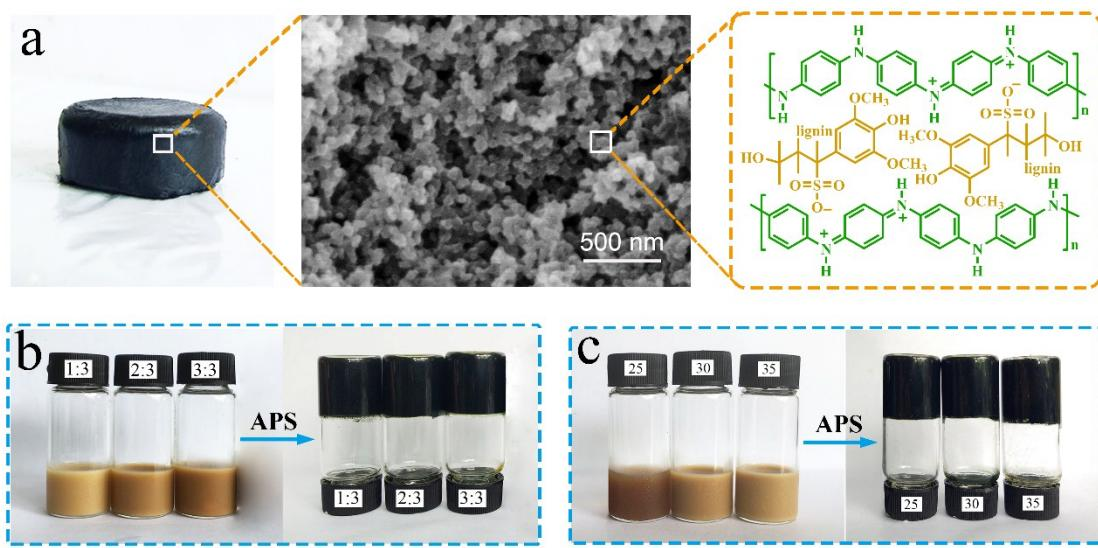
**Fig. S2.** (a) Lig/PANI at three length-scales. Left: photograph of Lig/PANI hydrogel; middle: a SEM image of Lig/PANI; right: a schematic molecular structure of Lig/PANI. (b) Photographs of the Lig/Ani aqueous dispersion with different mass ratio of Lig to Ani before and after adding APS oxides. (c) Photographs of the Lig/Ani aqueous dispersion with different concentration of Ani ( $\text{mg mL}^{-1}$ ) before and after adding APS.
