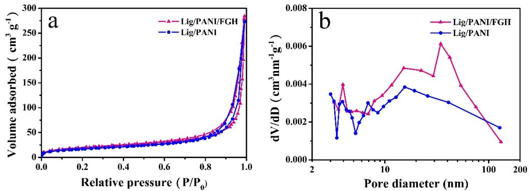
**Fig. S4.** (a) Adsorption–desorption isotherm curves and (b) the pore size distribution of the Lig/PANI/FGH and Lig/PANI determined by the Barrett-Joyner-Halenda method.
