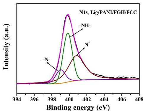
**Fig. S11.** N1s core-level spectrum of Lig/PANI/FGH/FCC.
