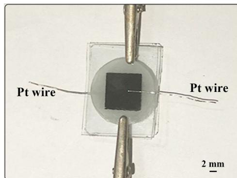
**Fig. S12.** Photograph of the conventional supercapacitor configuration using 1M H<sub>2</sub>SO<sub>4</sub> as electrolyte.
