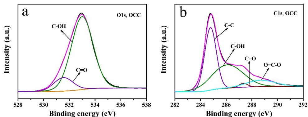
**Fig. S9.** (a) O1s and (b) C1s core-level spectra of OCC.
