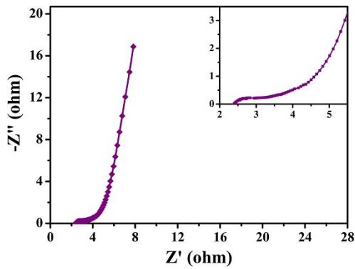
**Fig. S17.** Nyquist plots (the inset shows a magnified view of the high-frequency region) of Lig/PANI/FGH/FCC-based supercapacitor with PVA-H<sub>2</sub>SO<sub>4</sub> as electrolyte.
