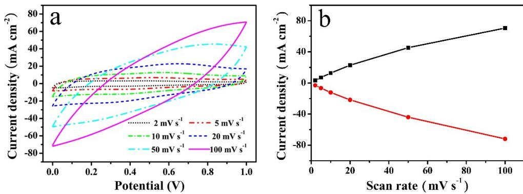
**Fig. S18.** (a) CV curves at different scan rates ( $2\text{--}100\text{ mV s}^{-1}$ ), and (b) the relationship between the maximum current density and scan rate from CV curves for Lig/PANI/FGH/FCC-based supercapacitor with PVA-H<sub>2</sub>SO<sub>4</sub> as electrolyte.
