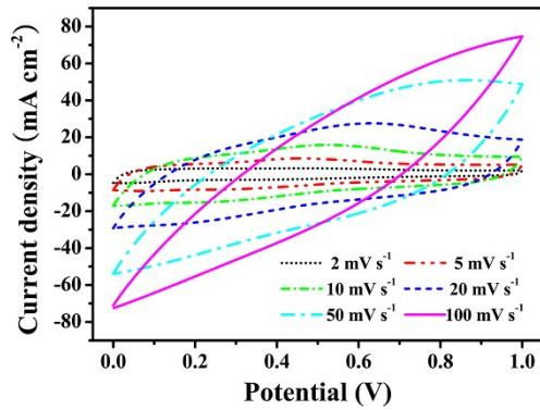
**Fig. S13.** CV curves of Lig/PANI/FGH/FCC based supercapacitor measured at different scan rates ( $2\text{--}100\text{ mV s}^{-1}$ ).
