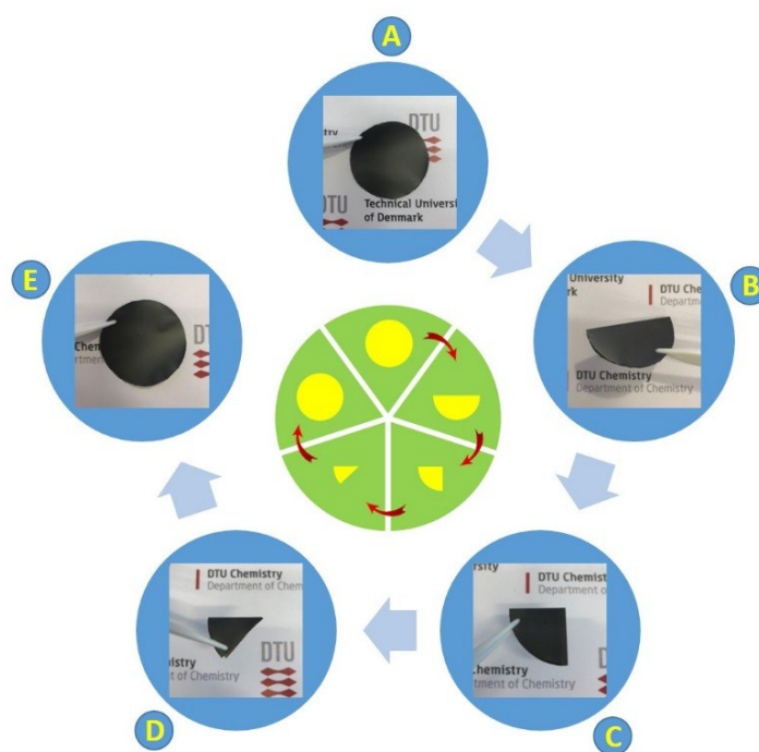
Fig. S7. Photos of an N-RGO-CNT-CBNP-P showing its flexibility: (A) initial state; (B) folded once; (C) folded twice; (D) folded thrice; (E) unfolded completely.
