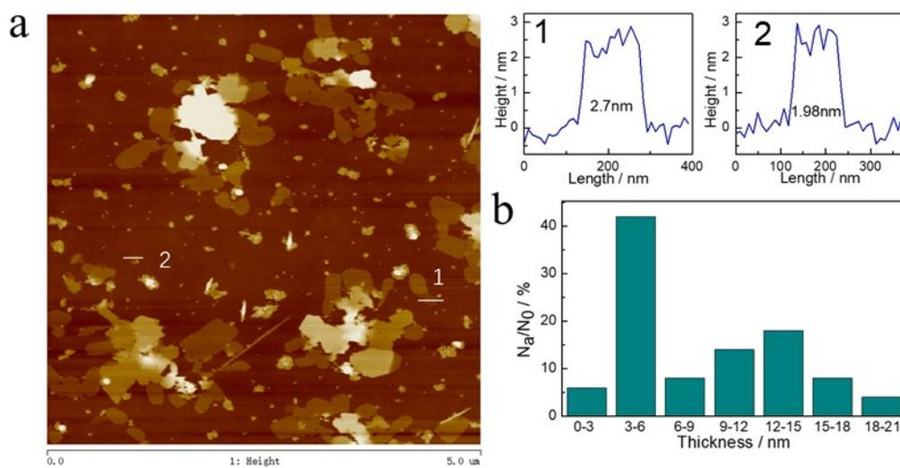
Figure S3. (a) AFM image of deposited few layer antimonene on SiO<sub>2</sub>/Si substrate and the height analysis of typical samples. (b) Statistical histogram of the thickness on 100 nanosheets.
