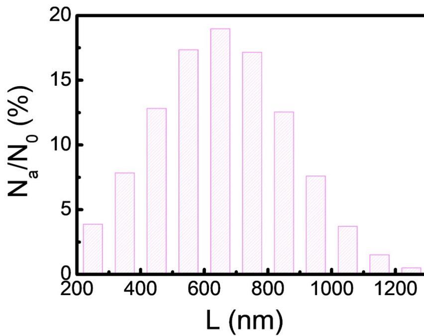
Figure S2. The statistical diagram of nanosheets lateral size on 100 flakes.
