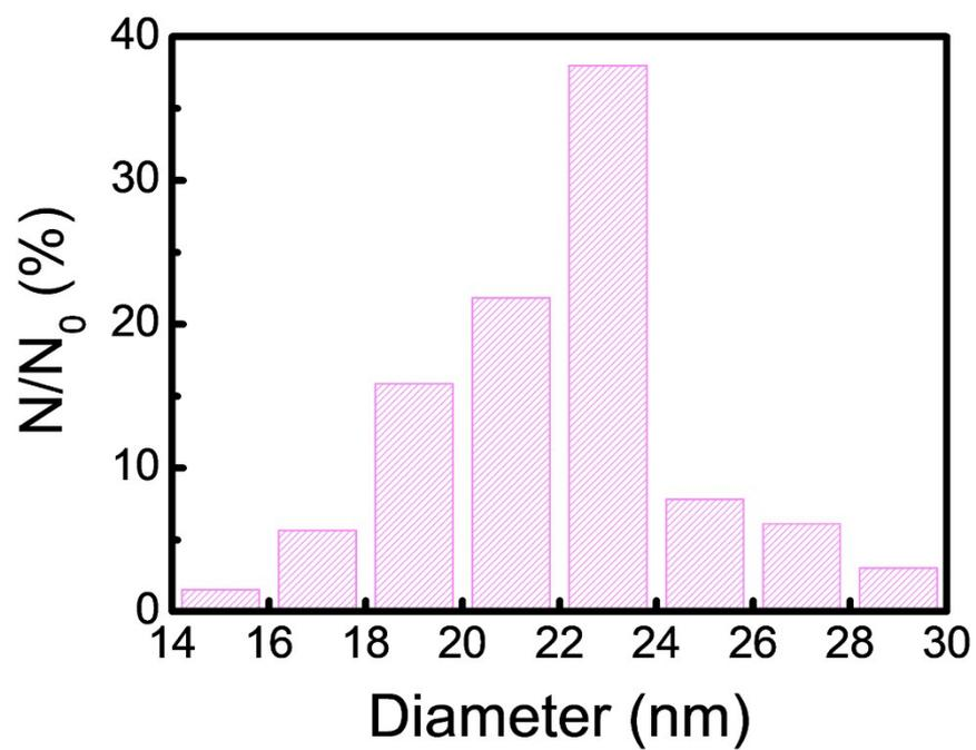
Figure S4. The statistical diagram of Sb QDs lateral size on 100 flakes.
