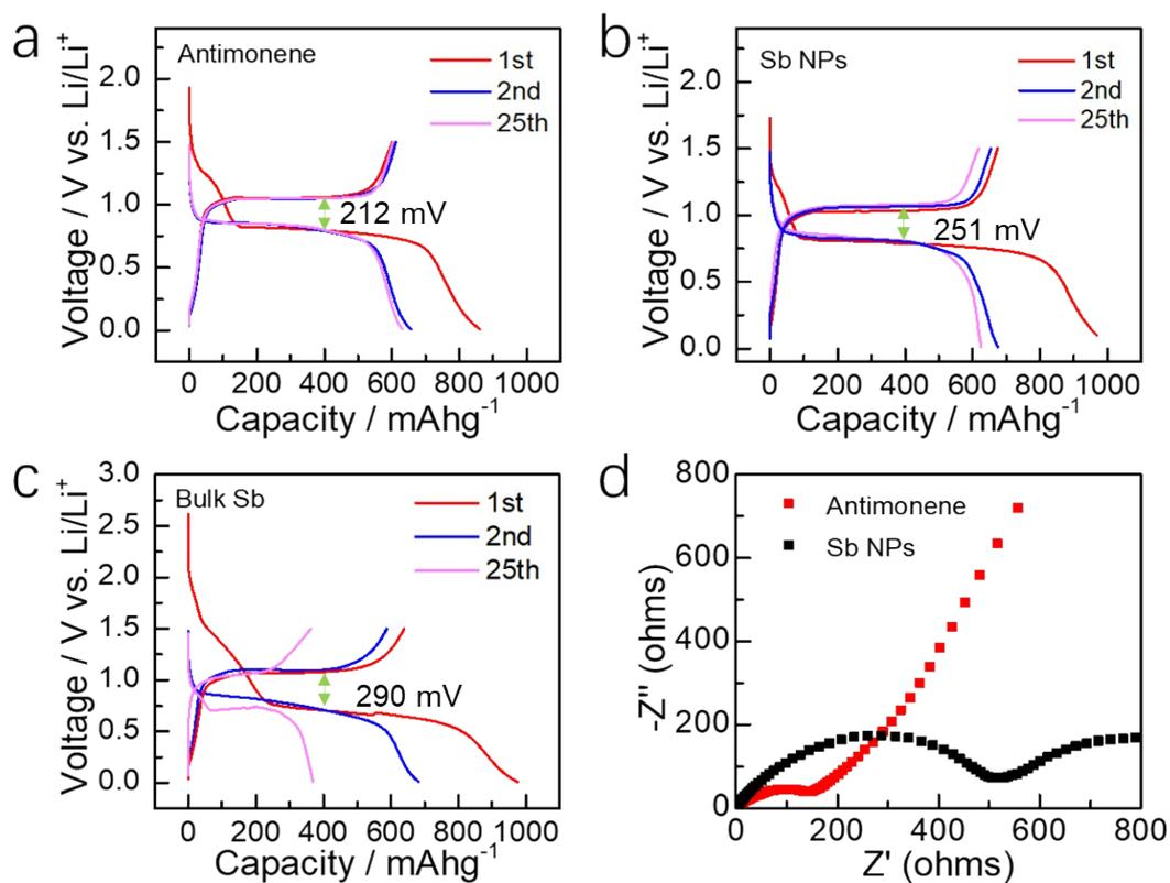
Figure S6. The charge-discharge profiles of antimonene (a), Sb nanoparticle (b) and bulk Sb (c), respectively. (d) The electrochemical impedance spectroscopy (EIS) of both antimonene and Sb NPs.
