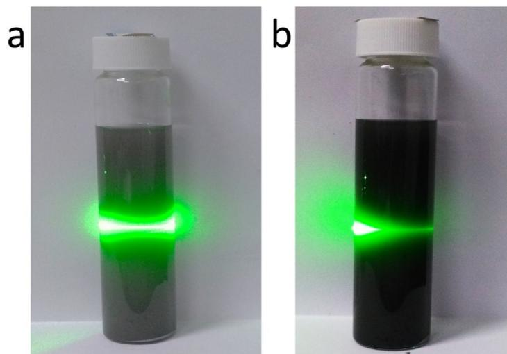
Figure S1. Photographs of antimonene colloid (a) and Sb QDs colloid (b) with Tyndall effect.
