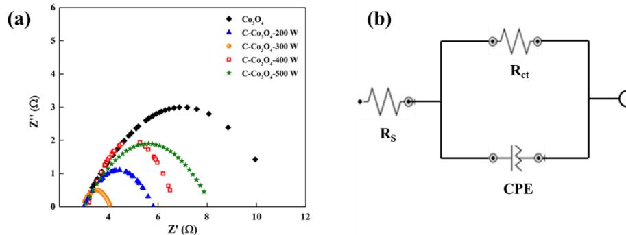
Fig. S5 (a) EIS plots for various kinds of Co<sub>3</sub>O<sub>4</sub>; (b) equivalent circuit diagram for fitting EIS.
