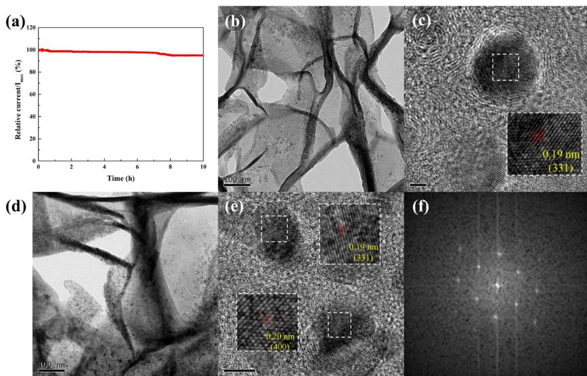
Fig. S6 (a) Chronoamperometry curve of C-Co<sub>3</sub>O<sub>4</sub> sample treated at 300 W; (b) (d) FESEM, (c) (d) HRTEM and (f) Live Fast Fourier Transform (FFT) images of C-Co<sub>3</sub>O<sub>4</sub> after stability tests.
