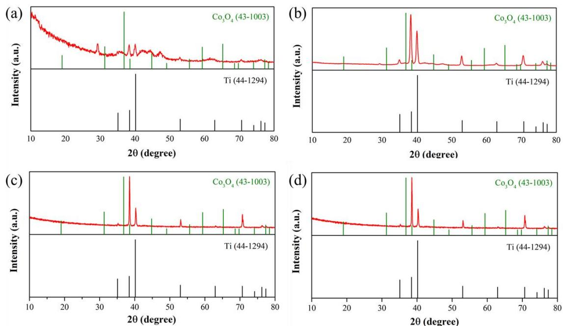
Fig. S3 GIXRD patterns of C-doped  $\text{Co}_3\text{O}_4$  sample under 300 W with (a) 1°; (b) 5°; (c) 10° input angle and (d) XRD pattern.
