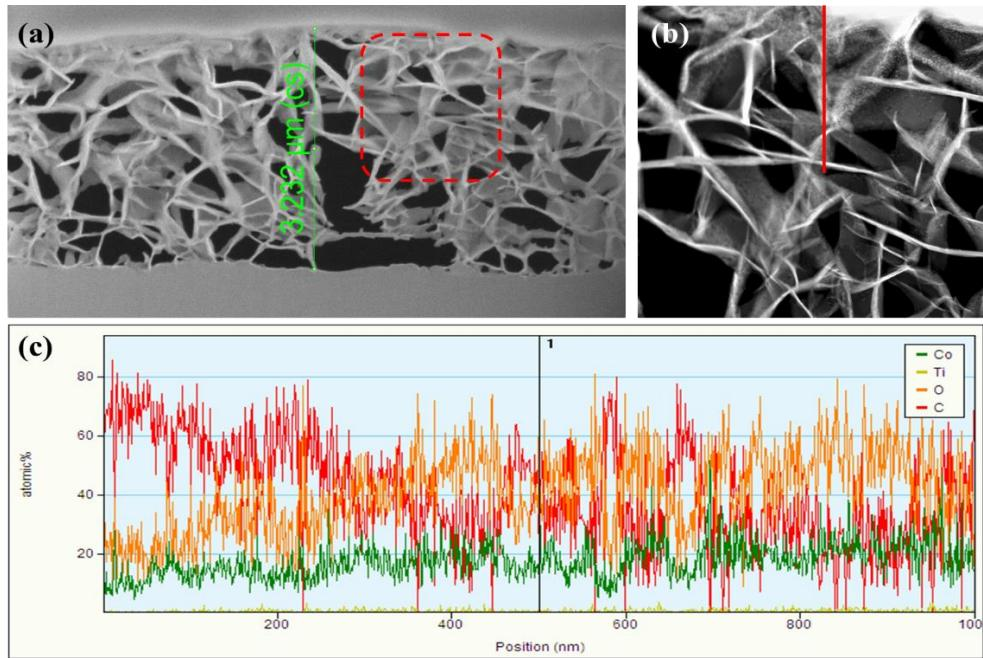
Fig. S2 SEM and EDS results for the section of C-doped  $\text{Co}_3\text{O}_4$  under 300 W treatment
