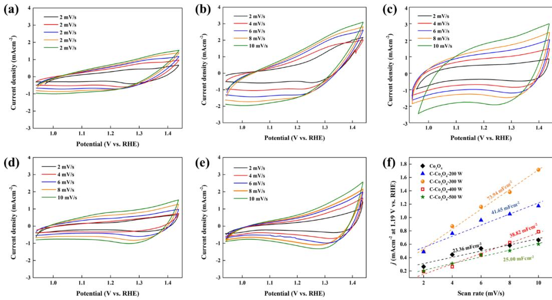
Fig. S4 CV plots for (a) pristine Co<sub>3</sub>O<sub>4</sub>; (b) treated under 200 W; (c) 300 W; (d) 400 W; (e) 500 W; (f) ECSA determined by the capacitive currents at 1.19 V vs. RHE
