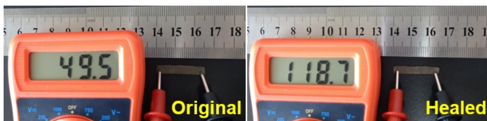
Fig. S10. Resistance change before and after self-healing of electric device taking TCR-20 sample as substrate.
