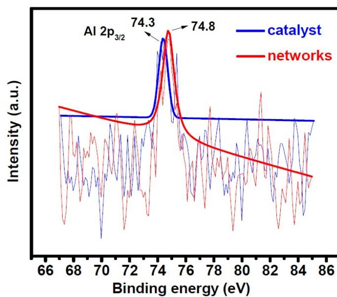
Fig. S9 Al ( $2p_{3/2}$ ) electron binding energy of the network 2 and catalyst 3.
