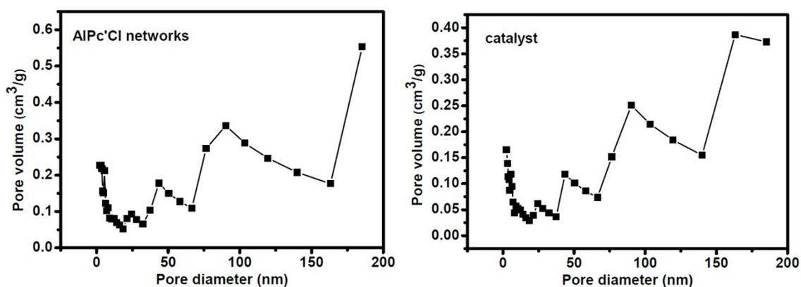
**Fig. S11** BJH pore-size distribution for the network **2** and catalyst **3**.
