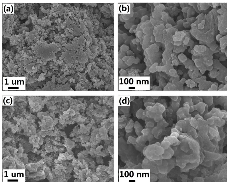
**Fig. S22** SEM images of catalyst **3** before (a, b) and after (c, d) 3 catalytic cycles.
