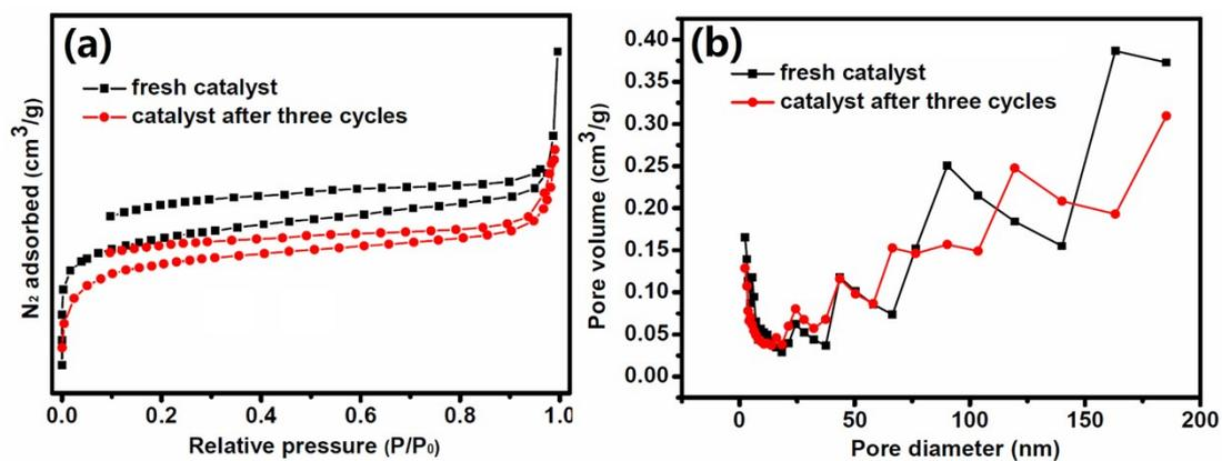
**Fig. S23** The BET surface areas (a) of catalyst before and after three catalytic cycles, with corresponding BJH pore-size distributions (b).
