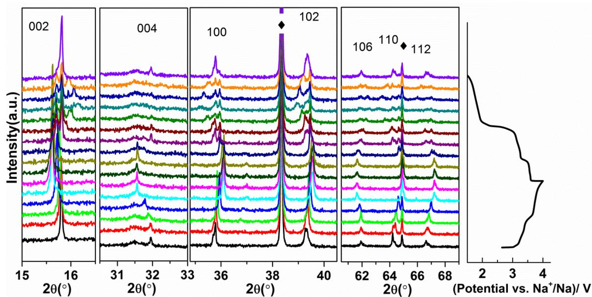
**Figure S5.** *In-situ* synchrotron XRD patterns of NNMO cycling between 4.0 and 1.5 V, the  $2\theta$  has been converted based on the Cu wavelength for convenience.
