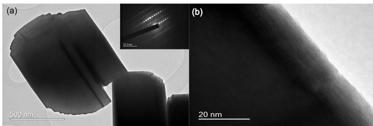
**Figure S3.** (a) TEM image and (b) high resolution TEM image showing lattice fringes of NNMO prepared at 850°C (inset: SADE pattern).
