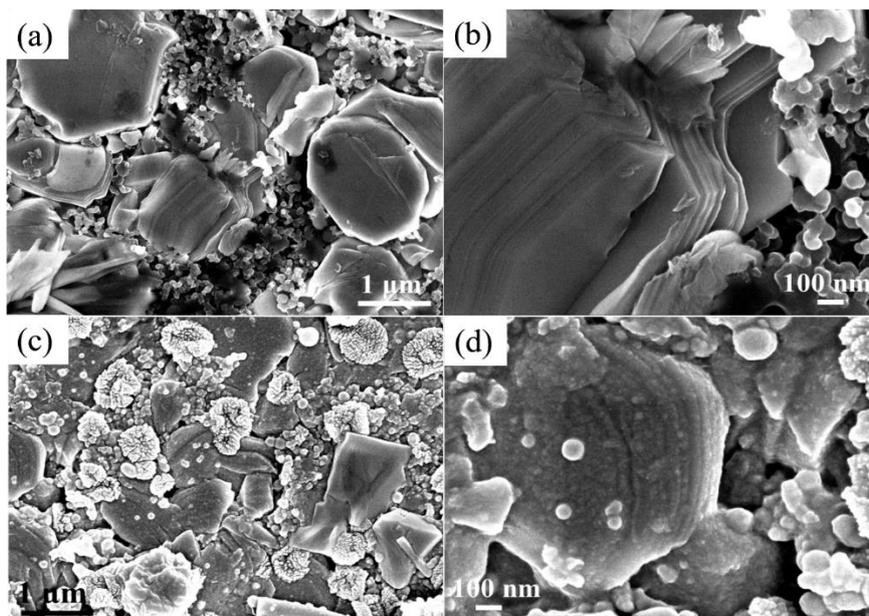
**Figure S7.** Electrodes before (a, b) and after (c, d) 1000 cycles at 1 C with super P and PVDF binder around.
