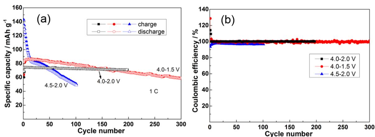
**Figure S4.** (a) Cycling performance and (b) corresponding CE of prepared NNMO with different cut-off voltages at 1 C.
