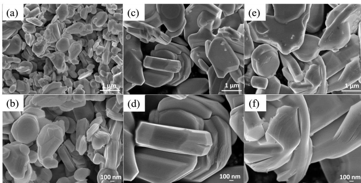
**Figure S2.** SEM morphologies of NNMO powders calcined at different temperatures: (a, b) 800; (c, d) 850; and (e, f) 900°C.
