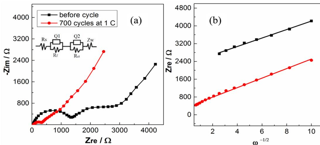
**Figure S6.** (a) Nyquist plots of prepared NNMO at 850°C before and after 700 cycles at 1 C (inset: equivalent circuit); and (b) corresponding  $Z_{re}$  vs.  $\omega^{-1/2}$  plots in the low frequency region.
