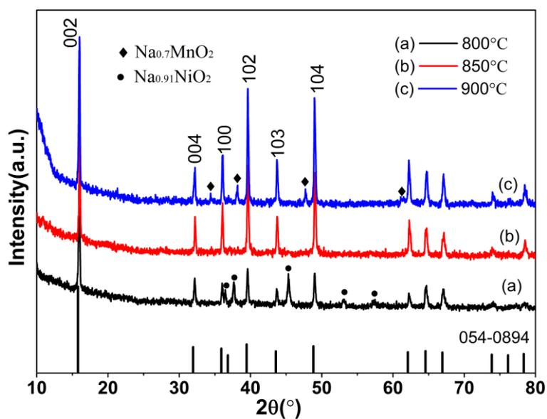
**Figure S1.** XRD patterns of NNMO prepared at different temperatures.
