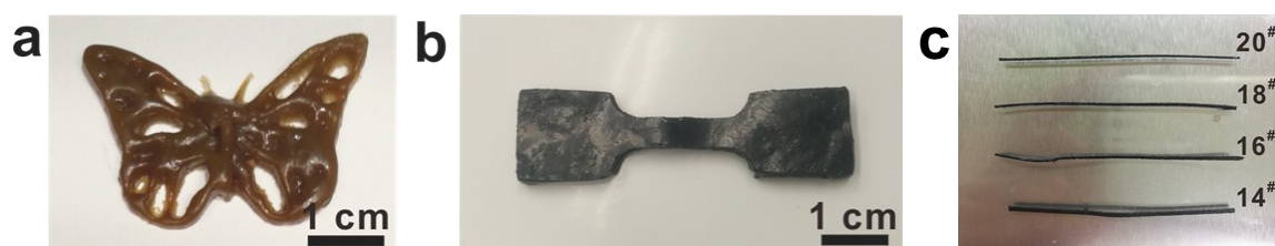
Fig. S5. Photographs of samples printed from (a) DAPU and (b) PDAPU10. (c) The ink filaments extruded from DIW printer with different nozzle diameters. The inner diameter of 14#, 16#, 18# and 20# nozzles is 1.6 mm, 1.2 mm, 0.84 mm and 0.64 mm, respectively. The ink filament diameter is approximately equal to the nozzle size.
