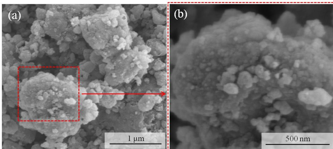
Figure S5. Typical SEM images of as-milled  $\text{MgH}_2$  after ten cycles.
