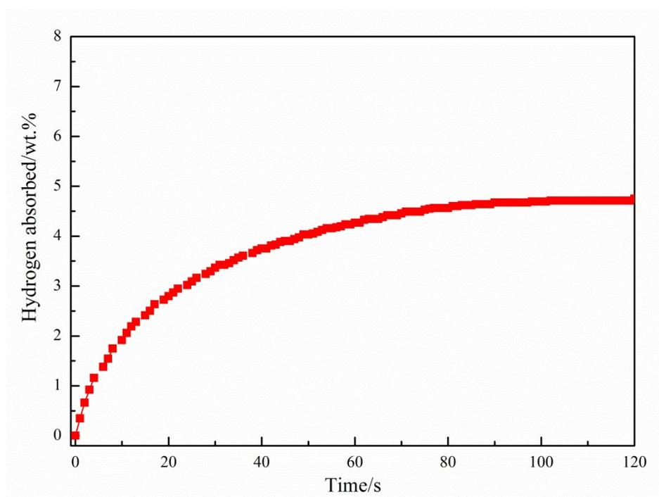
Figure S3. Isothermal rehydrogenation curve of as-milled MgH<sub>2</sub> at 250 °C under 80 bar hydrogen back pressure.
