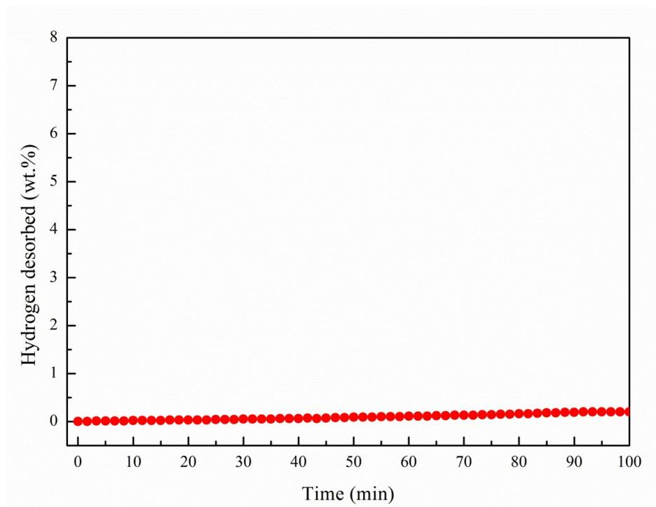
Figure S4. Isothermal dehydrogenation curve of as-milled  $\text{MgH}_2$  at  $275\text{ }^\circ\text{C}$  under 0.02 bar hydrogen back pressure.
