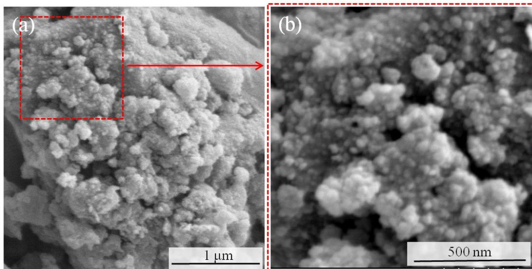
Figure S6. Typical SEM images of MgH<sub>2</sub>-10 wt.% Co/Pd@B-CNTs after ten cycles.
