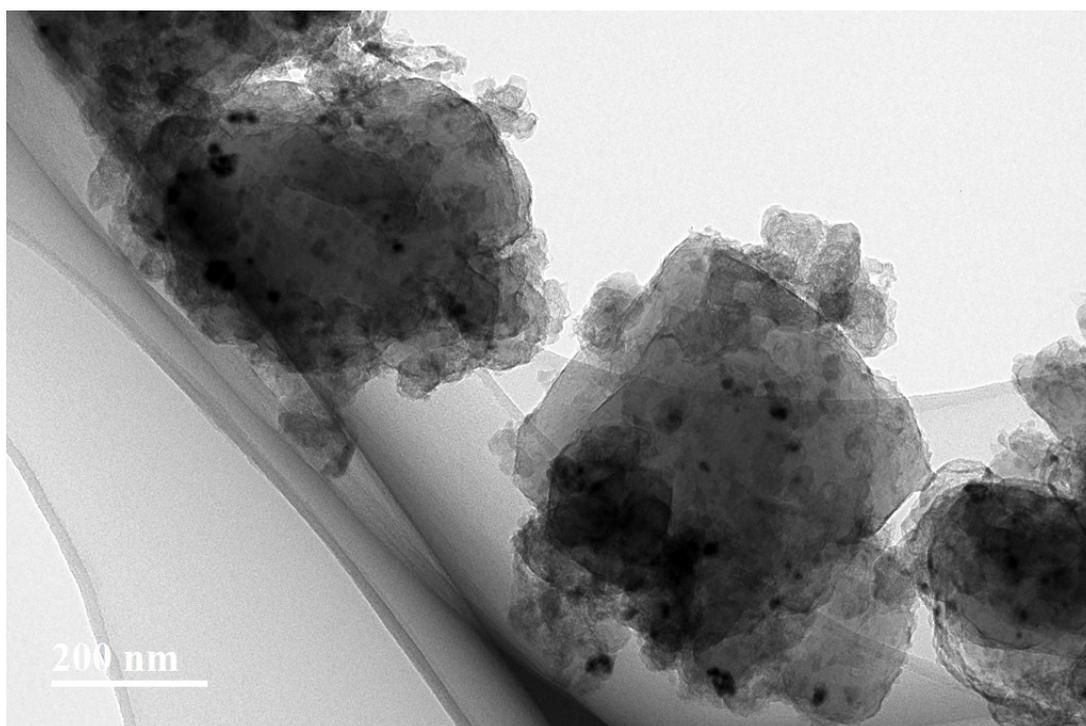
Figure S7. Typical TEM image of as-milled MgH<sub>2</sub> after ten cycles.
