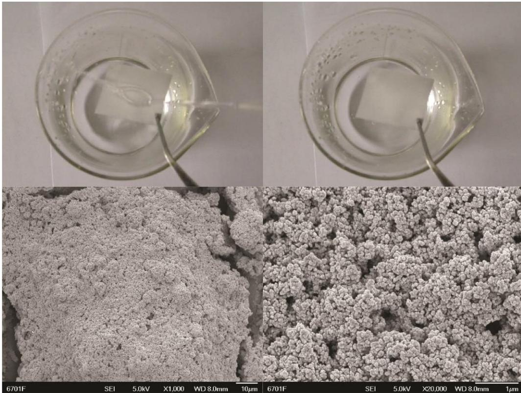
**Fig. S33** The process of the water impact test and SEM images of the TiO<sub>2</sub>-AP-FOTS coated SSM after the water impact test for 10 cycles. Water droplets randomly impact the SSM surface and promptly bounce without any residual small water droplets.
