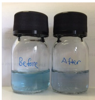
Figure S8. Titrating samples before and after the equivalent point.
