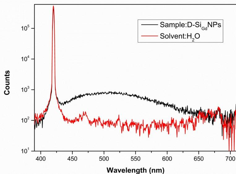
**Fig. S6.** APLQY spectra of the as-prepared D-Si<sub>Gd</sub>NPs. The APLQY value was measured by FLS-920 instrument equipped with an integrating sphere.
