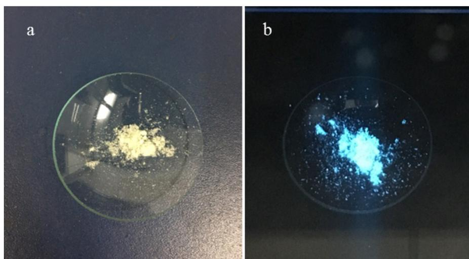
**Fig. S1.** The photographs of the D-Si<sub>Gd</sub>NPs powder via lyophilization after dialysis under ambient light (a) and 365 nm UV irradiation (b).
