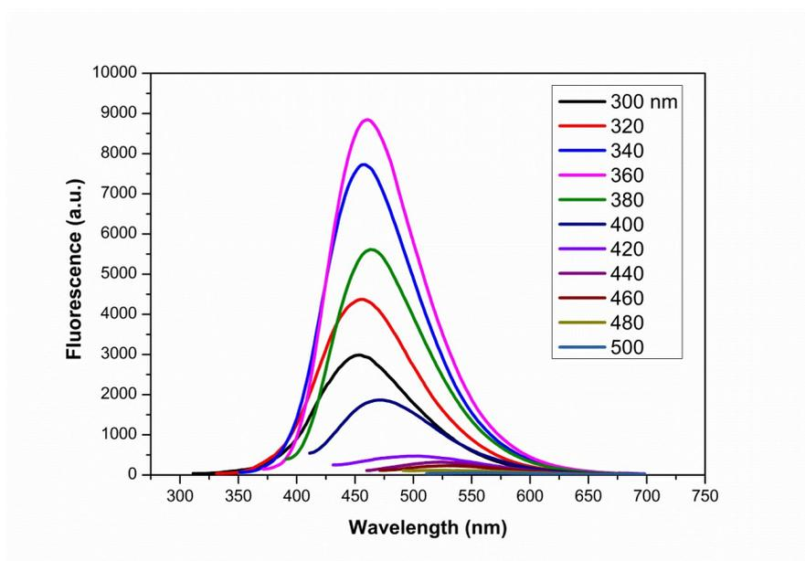
**Fig. S5.** PL spectra of SiNPs at different excitation wavelength from 300 nm to 500 nm.
