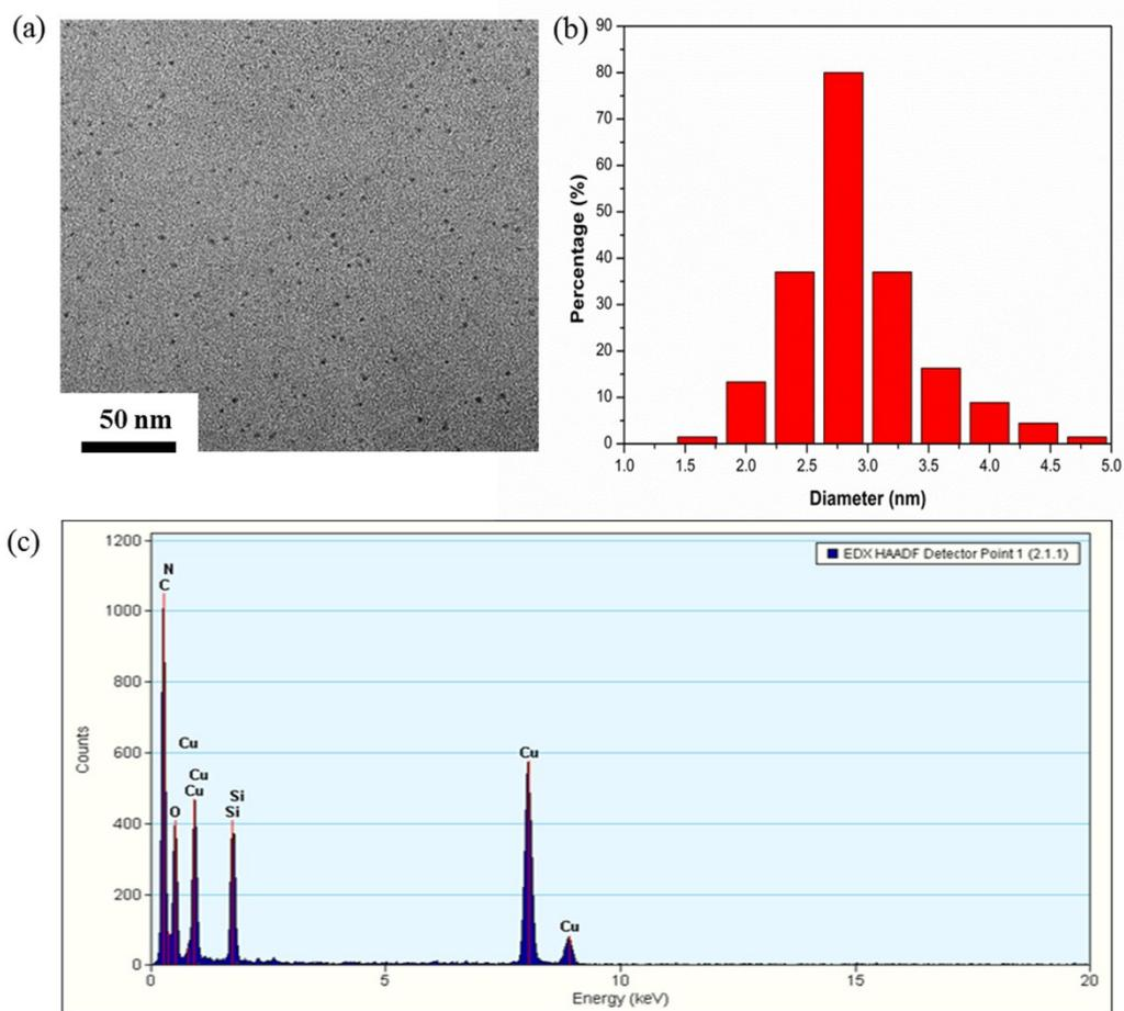
**Fig. S3.** (a) TEM image, (b) corresponding size distribution histogram and (c) EDX pattern of the D-Si<sub>Gd</sub>NPs prepared at reaction time of 1 h.
