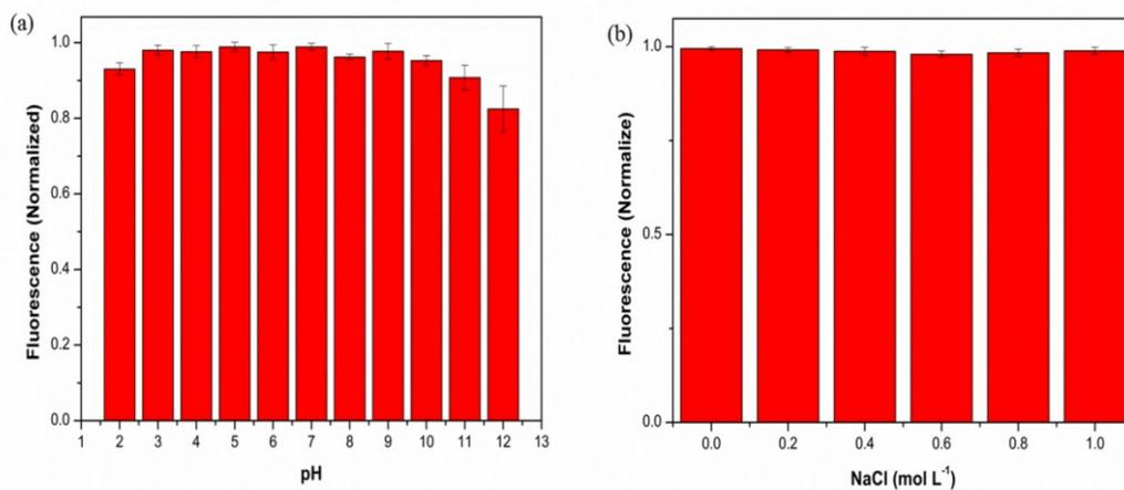
**Fig. S7.** The stability of the as-prepared D-Si<sub>Gd</sub>NPs. (a) pH stability in water; (b) Salt effect.
