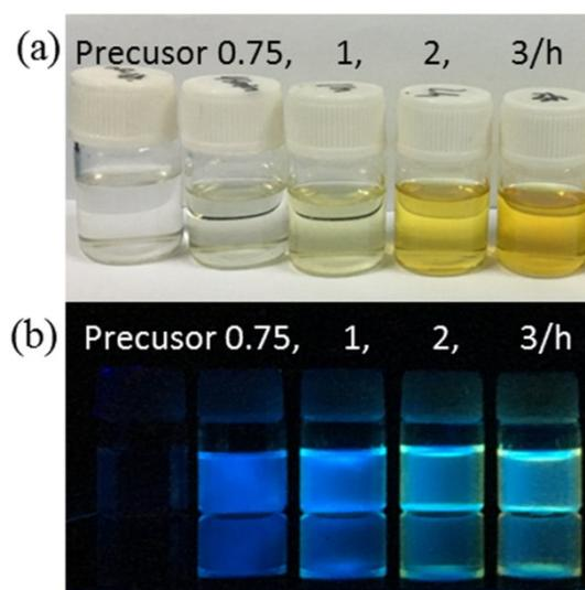
**Fig. S2.** The photographs of the D-Si<sub>Gd</sub>NPs prepared at different reaction times (precursor, 0.75, 1, 2, 3 h) under ambient light (a) and 365 nm UV irradiation (b).
