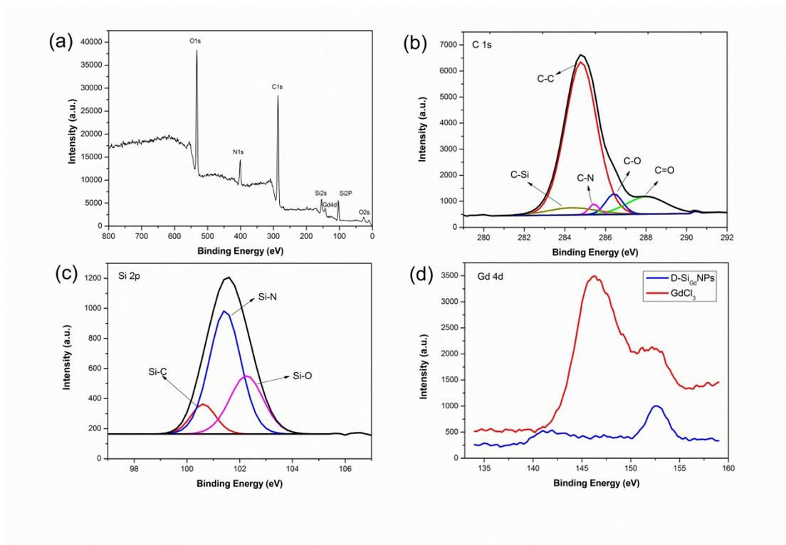
**Fig. S4.** The XPS spectra of the D-Si<sub>Gd</sub>NPs: (a) full range, (b) C 1s, (c) Si 2p, (d) Gd 4d.
