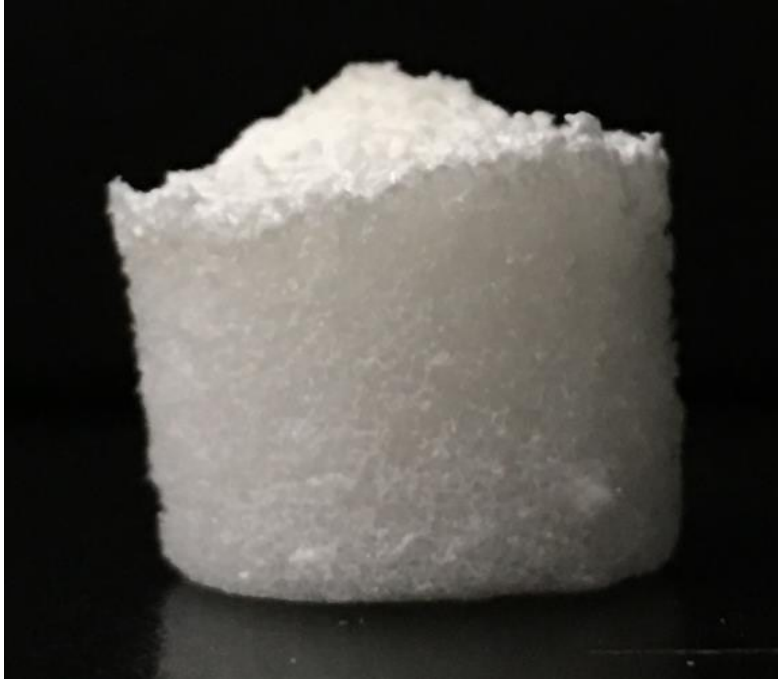
Figure S2 Typical optical image of the salt-leached scaffolds
