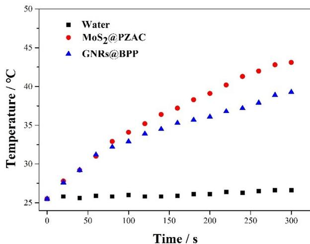
Figure S11. The temperature variations of MoS<sub>2</sub>@PZAC and GNRs@BPP with the same concentration under laser irradiation (808 nm, power density of 1 W/cm<sup>2</sup>).
