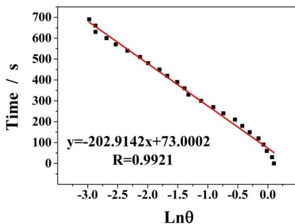
Figure S8. Linear time versus  $\text{Ln}\theta$  obtained from the cooling period in Figure S7.
