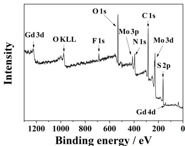
Figure S2. XPS survey spectrum of MoS<sub>2</sub>@PZAC.
