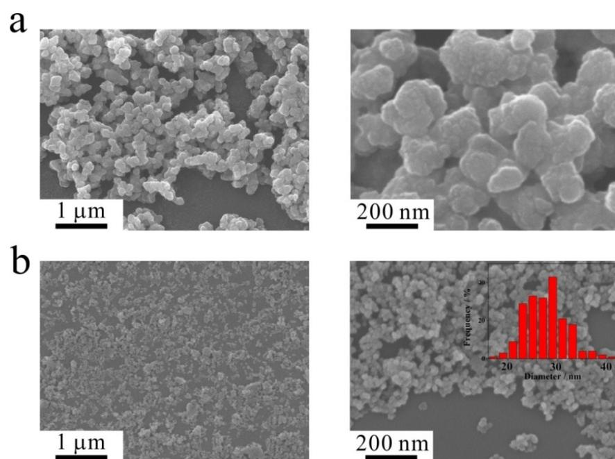
Figure S3. SEM images of (a) MoS<sub>2</sub> and (b) MoS<sub>2</sub>@PZAC.
