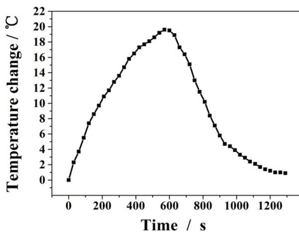
Figure S7. The PTT temperature change of MoS<sub>2</sub>@PZAC aqueous dispersion with a NIR laser irradiation on-off.
