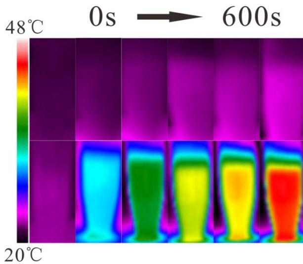
Figure S5. Infrared thermal images of water (top) and MoS<sub>2</sub>@PZAC dispersion (bottom) at different time points under NIR laser irradiation (1 W/cm<sup>2</sup>).
