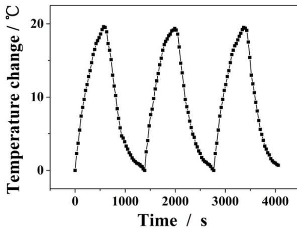
Figure S6. The temperature variations of MoS<sub>2</sub>@PZAC dispersion at 100 µg/mL under irradiation with an 808 nm laser at a power density of 1 W/cm<sup>2</sup> for three on-off cycles
