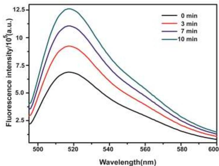
**Fig.S4.** Fluorescence recovery of substrate mRNA by the released DNAzyme after light irradiation.
