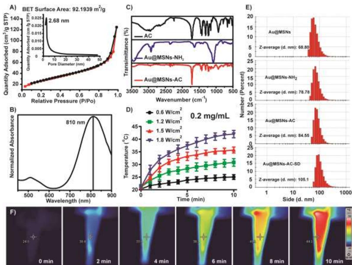
**Fig. S1.** (A)  $N_2$  sorption isotherms of Au@MSNs. (B) UV-Visible spectra of the Au@MSNs. (C) FT-IR spectra of AC, Au@MSNs-NH<sub>2</sub>, and Au@MSNs-AC. (D) Temperature changes of 0.2 mg/mL nanocarriers at different power densities. (E) DLS of Au@MSNs, Au@MSNs-NH<sub>2</sub>, Au@MSNs-AC, and Au@MSNs-AC-SD. (F) Thermographic images of Au@MSNs-AC aqueous soli
