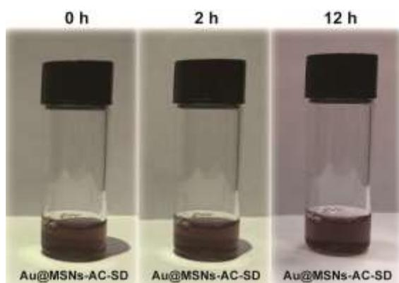
**Fig. S5.** Photographs indicating the stability of Au@MSNs-AC-SD in PBS at 0, 2, 12 h.
