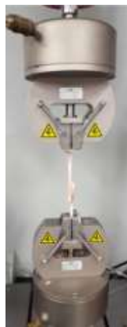
Figure S20. Representative image of lap shear test.
