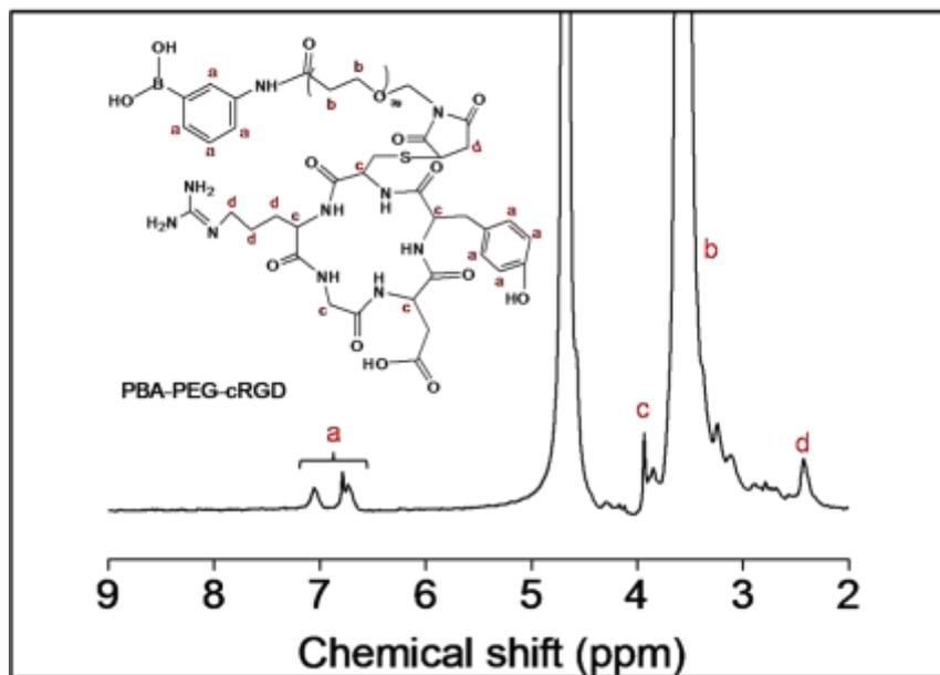
Figure S5.  $^1\text{H-NMR}$  spectrum of PBA-PEG-cRGD measured in  $\text{D}_2\text{O}$  at  $25^\circ\text{C}$ .
