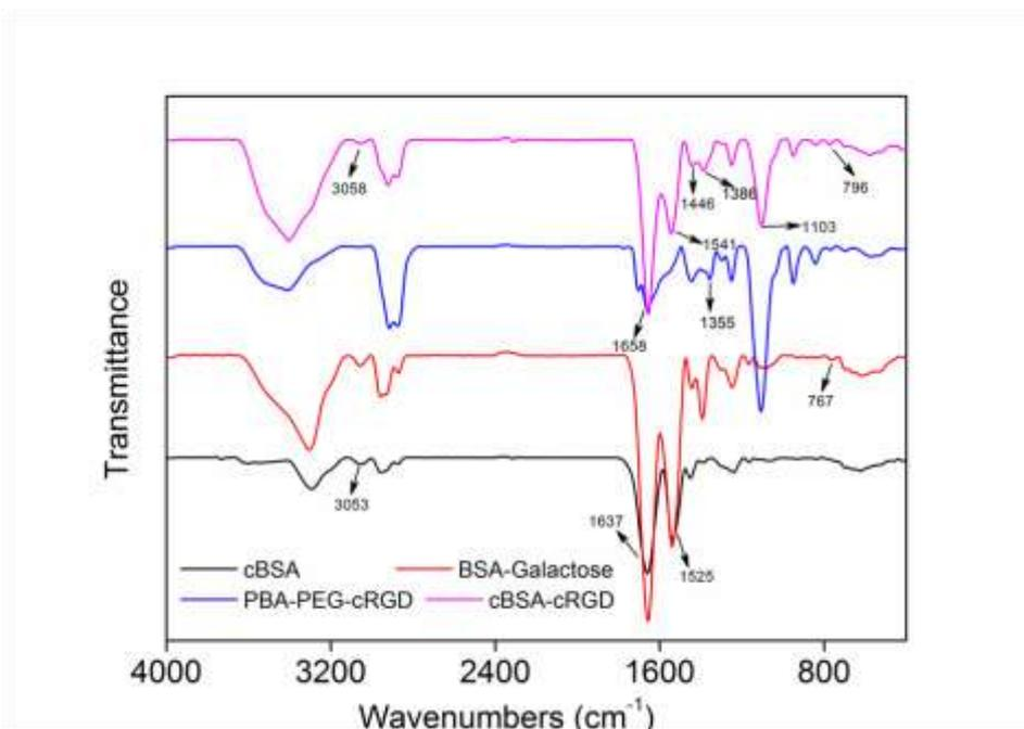
Figure S6. FTIR spectra of cBSA, cBSA with Galactose, PBA-PEG-cRGD, and cBSA-cRGD.
