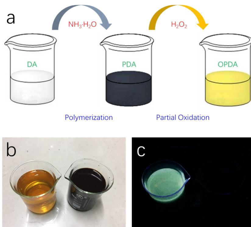
**Fig. S2** a, Schematic of PDA and OPDA synthesis process, the beaker model is from ChemBioOffice 14.0.; b, digital picture of mass production PDA and OPDA under nature light; c, digital picture of mass production PDA and OPDA under UV light.
