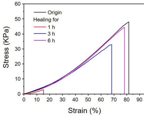
**Figure S11.** Tensile test of the PLGA based self-healing hydrogel after different healing period.
