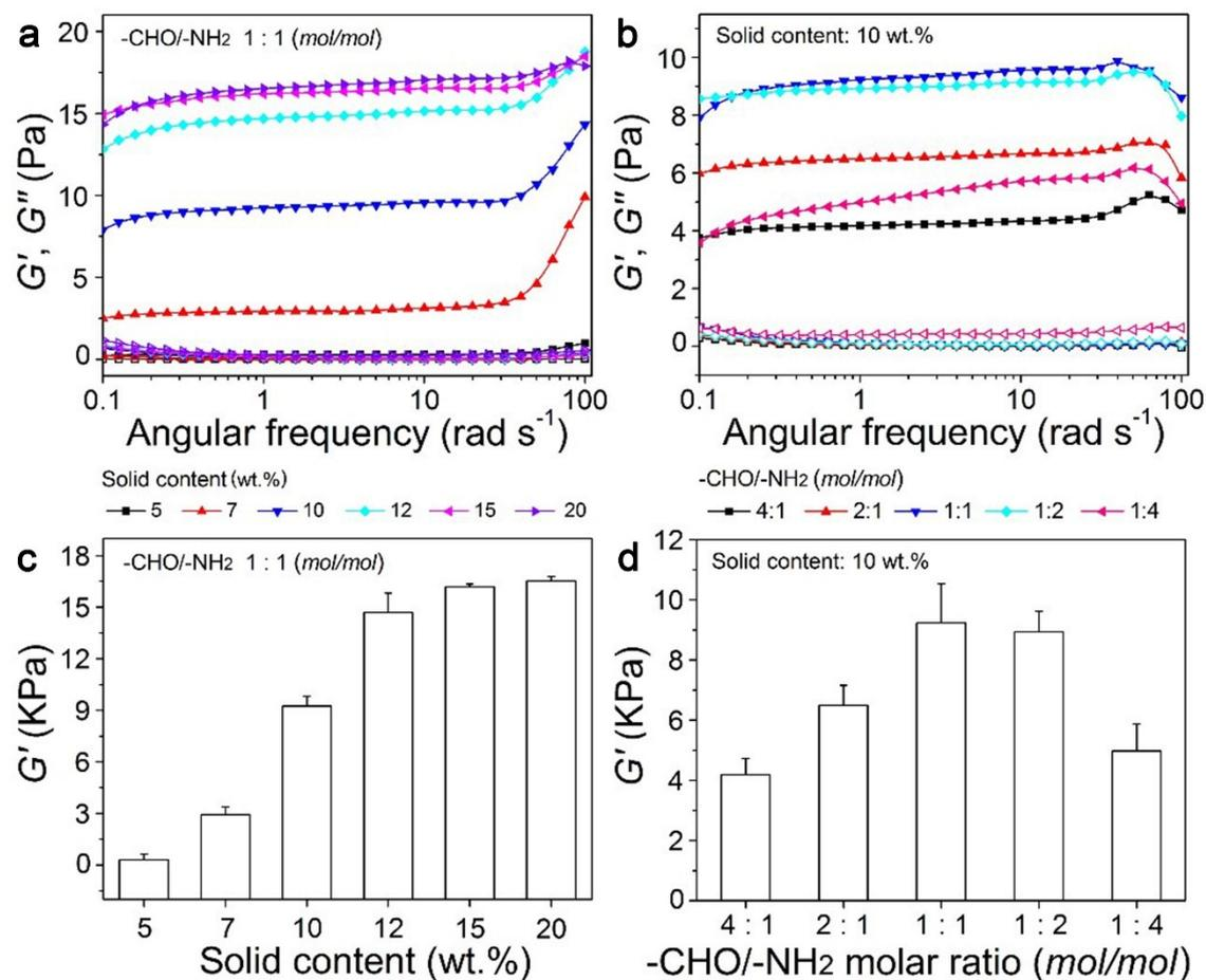
**Figure S10.** Rheological characterization of self-healing hydrogel with (a, c) different solid content and (b, d) different -CHO/-NH<sub>2</sub> molar ratio. The experiment was carried out under 1% strain and values in (c, d) represent  $G'$  at  $\omega = 1 \text{ rad s}^{-1}$ .
