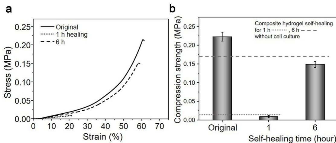
**Figure S14.** Self-healing of the composite hydrogel after cell seeding. (a) Compressive stress-strain curves.
