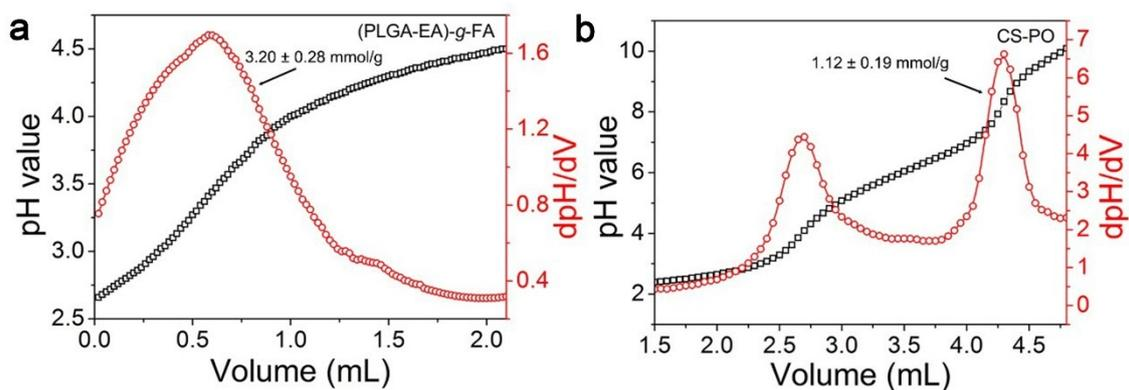
**Figure S7.** (a) Hydroxylamine hydrochloride titration curve and differential curve of (PLGA-EA)-g-FA. (b) Polymer potentiometric titration curve and differential curve of CS-PO.
