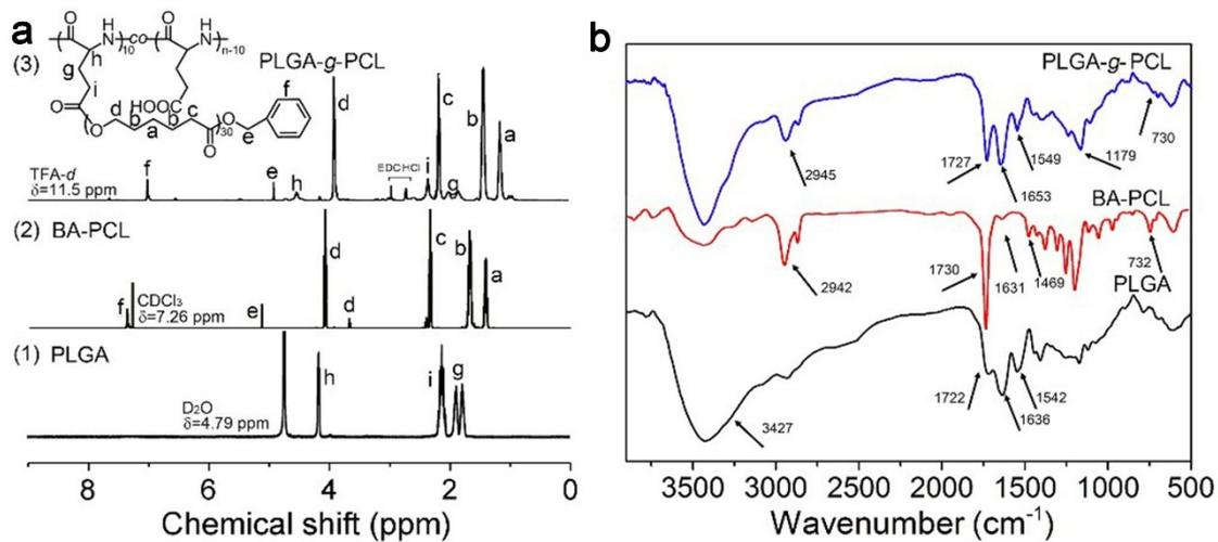
**Figure S1.** Characterization of PLGA-g-PCL. (a) <sup>1</sup>H NMR spectra, (b) FTIR spectra.
