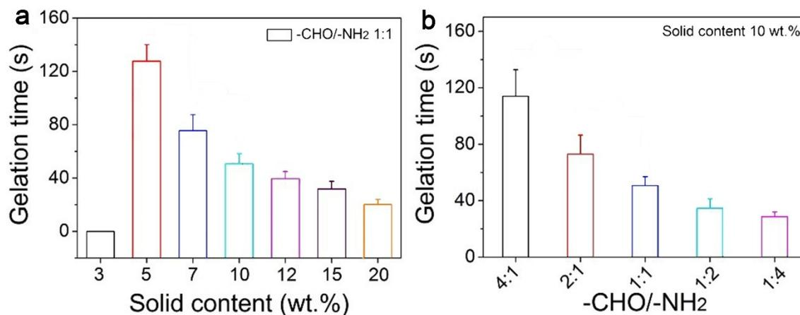
**Figure S9.** Gelation time of self-healing hydrogel with (a) different solid content and (b) different -CHO/-NH<sub>2</sub> molar ratio.
