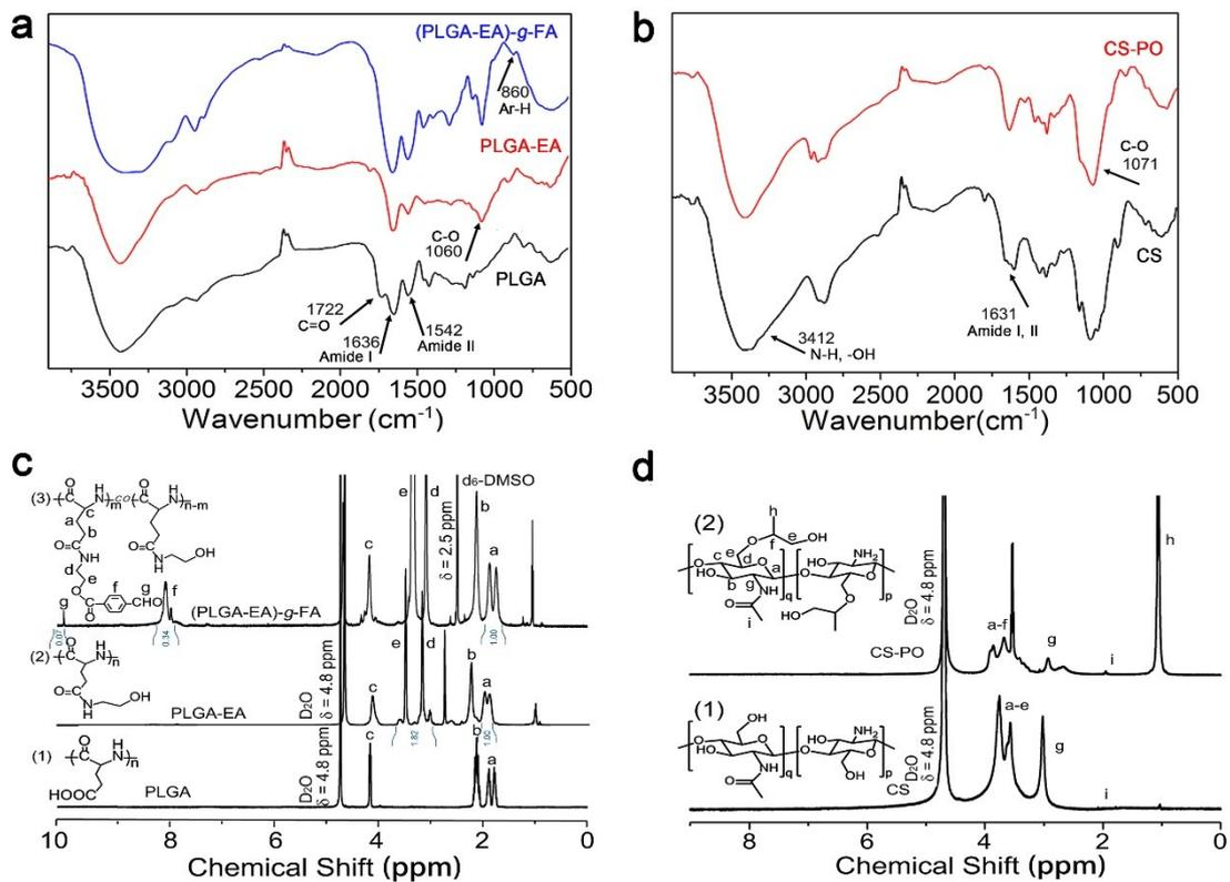
**Figure S6.** FT-IR spectra of (a) (PLGA-EA)-g-FA and (b) CS-PO.  $^1\text{H}$  NMR spectra of (c) (PLGA-EA)-g-FA and (d) CS-PO.
