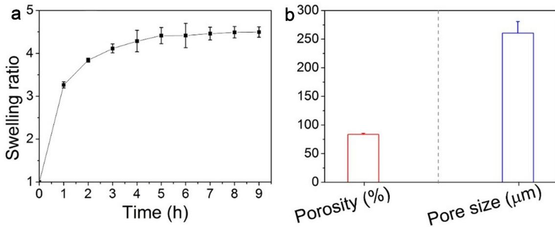
**Figure S4.** (a) Swelling kinetics, (b) porosity and average pore diameter of the PLGA based tough porous hydrogel skeleton.
