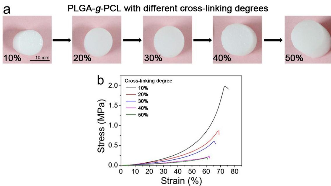
**Figure S2.** PLGA-g-PCL hydrogels with different cross-linking degrees after dialysis in water. (a)
