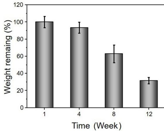
**Figure S5.** In vivo degradation of the PLGA based tough porous hydrogel skeleton. The data was calculated according to the thickness of the remaining skeleton from H&E staining images.
