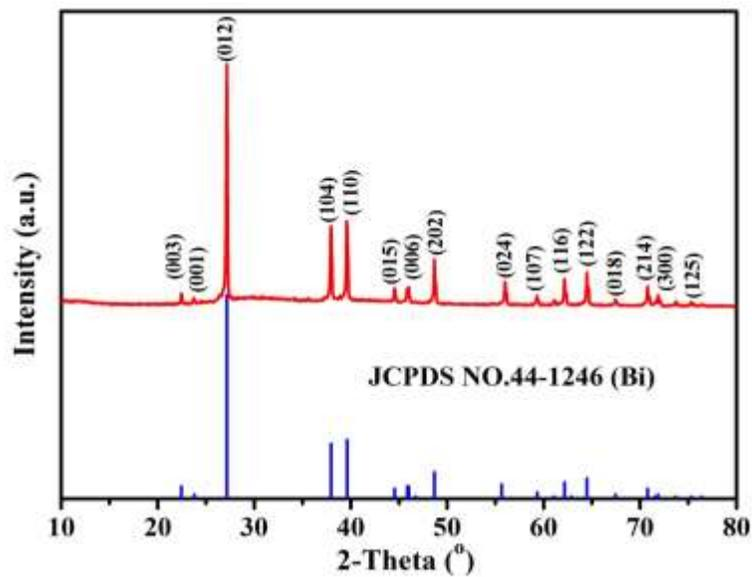
Fig. S4 Powder XRD patterns of pBi nanospheres.
