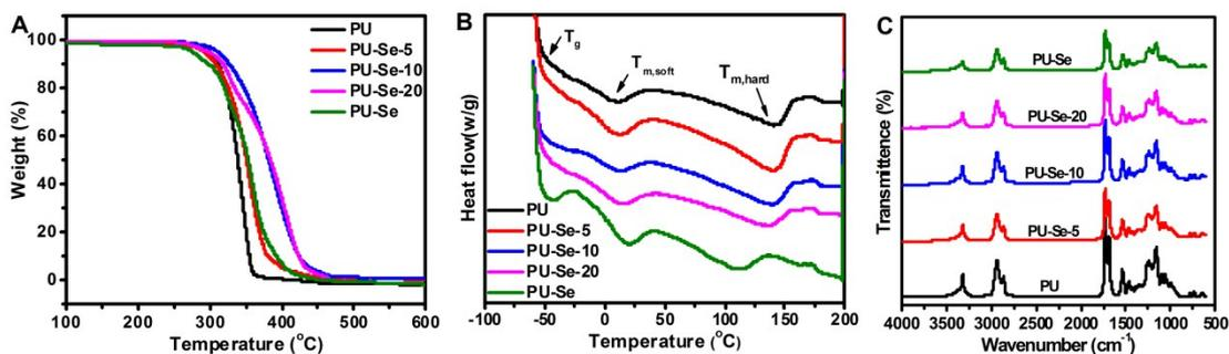
Fig. S6. (A) TGA and (B) DSC curves of different films under nitrogen atmosphere at the heating rate of 10 °C min<sup>-1</sup>. (C) FT-IR spectra of different films.
