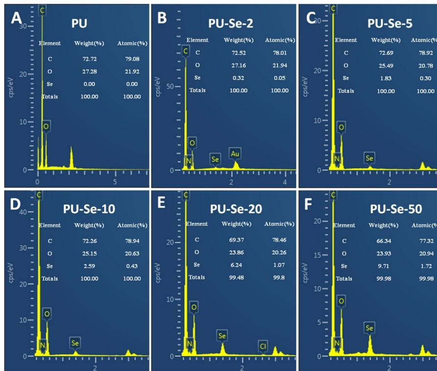
Fig. S2. EDS spectrograms of PU and PU/PU-Se blend films.
