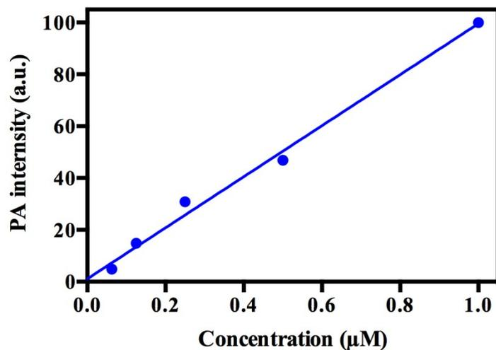
Figure S6. PA intensity-concentration plot shows the relationship between concentration of WSCP dots and PA intensity.
