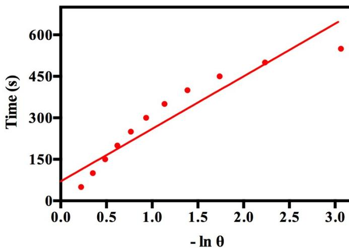
Figure S3. Linear time versus  $-\ln \theta$  obtained from the cooling period of Figure 2d.
