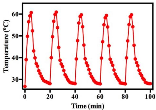
Figure S4. Photothermal profiles of WSCP dots aqueous solution for five ON/OFF cycles (730 nm, 1.0 W/cm<sup>2</sup>, 1 μM).
