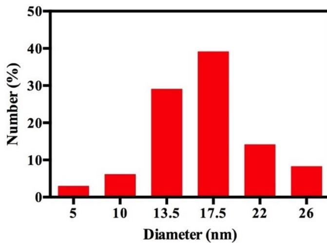
Figure S5. DLS size distribution histogram of WSCP dots after five ON/OFF cycles irradiation (730 nm laser).
