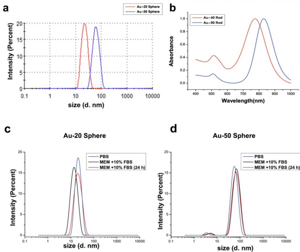
**Figure S1.** (a) Hydrodynamic diameters of Au-20 Sphere and Au-50 Sphere. (b) UV-vis-NIR spectra of Au-40 Rod and Au-90 Rod. (c) Stability of Au-20 Sphere in 10% serum-containing MEM. (d) Stability of Au-50 Sphere in 10% serum-containing medium.
