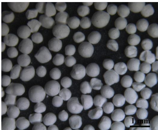
Fig.S3. Photograph containing a few spheres for 2.5 wt% PS/nCaCO 3 by an optical microscope.
