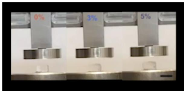
**Supplementary Video 1 Compressive failure of GH-DN hydrogels.**
