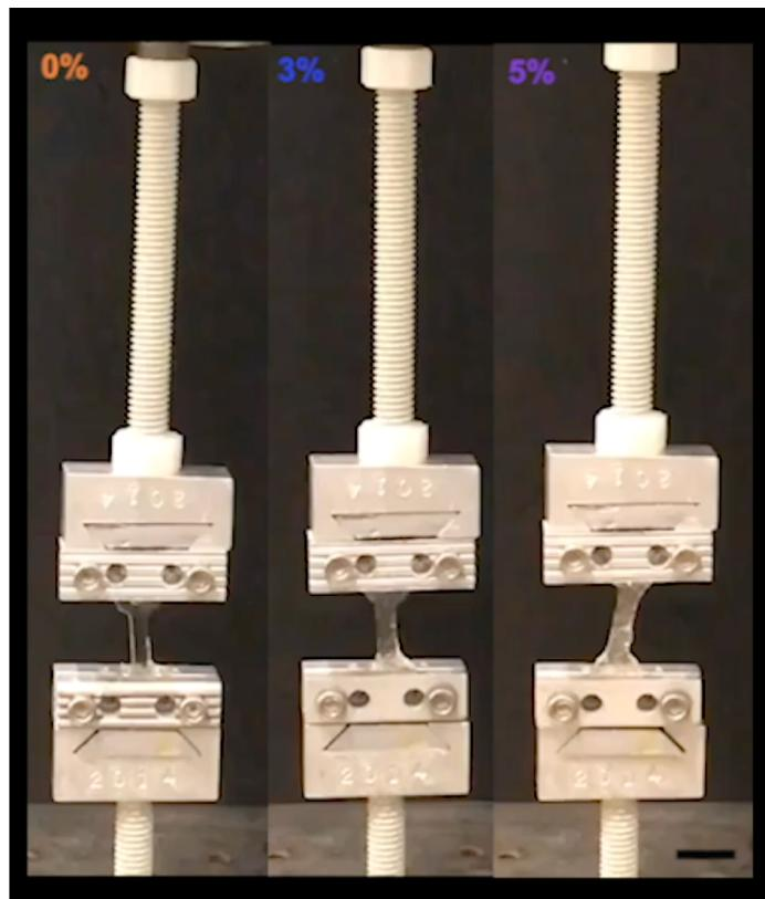
**Supplementary Video 2 Tensile failure of GH-DN hydrogels.**
