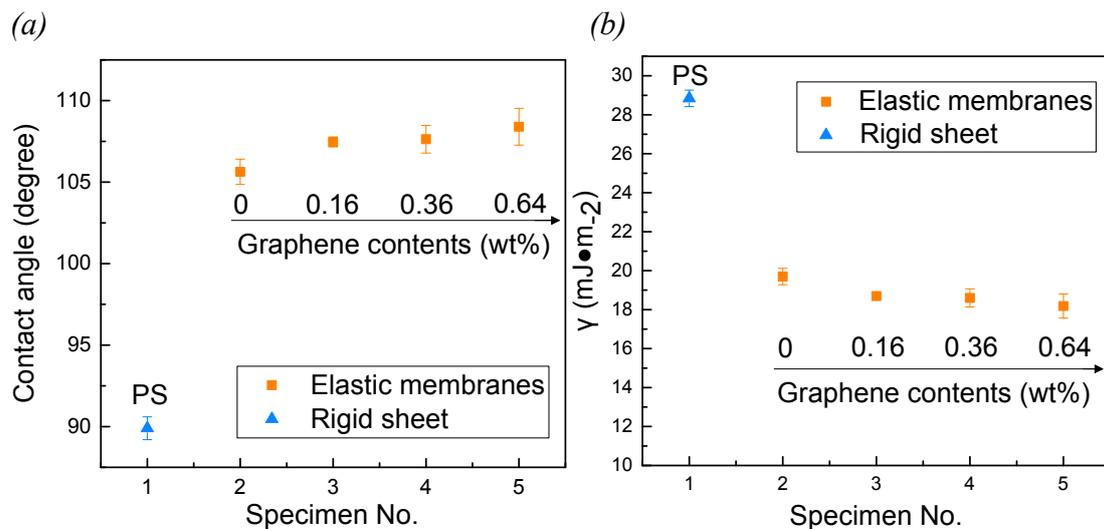
**Fig. S3** (a) Water contact angle of the rigid PS sheet and PSR/GSR membranes for various graphene contents at 20°C. (b) Surface energy of the rigid PS sheet and
