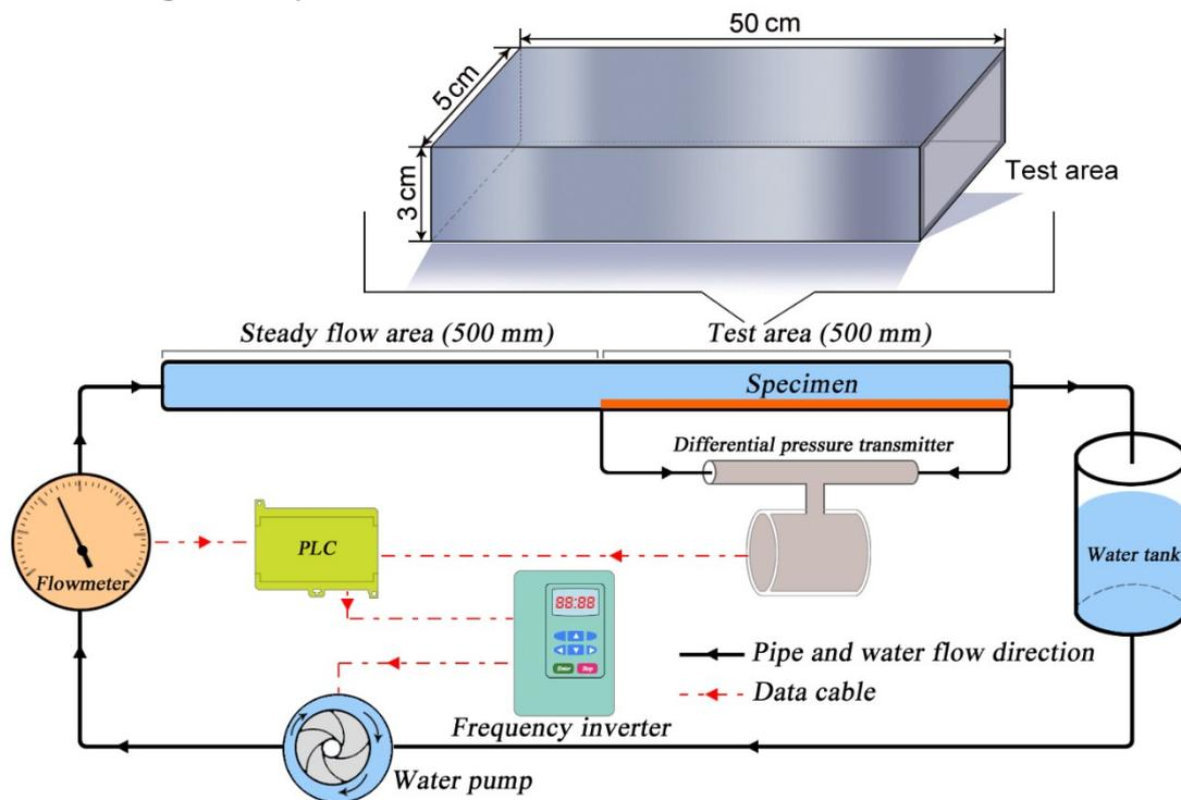
**Fig. S2** Schematic diagram of the flowing water system.
