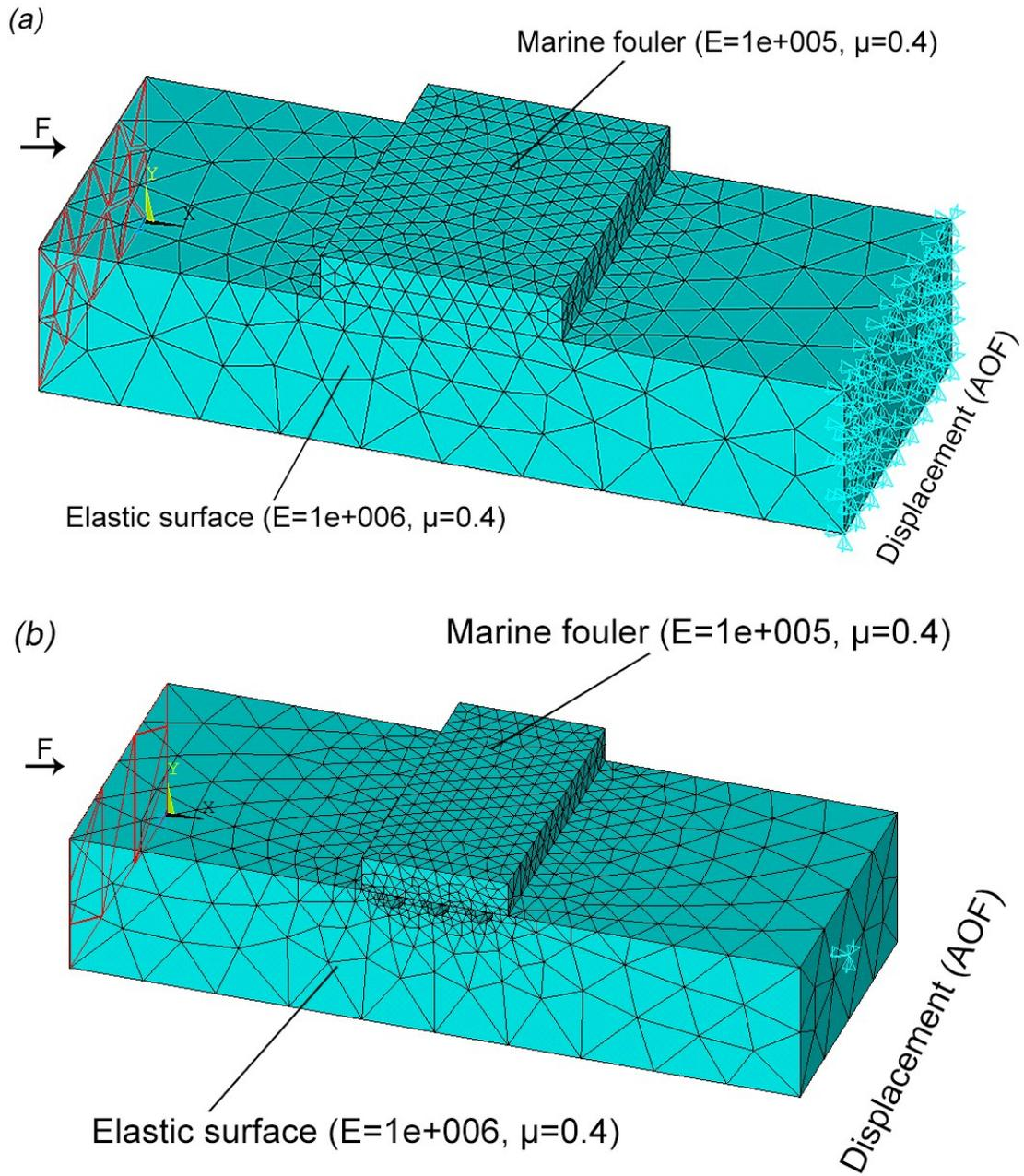
**Fig. S5** (a) A fouler was glued on the elastic surface. (b) A fouler was glued on the elastic surface with some flaws in attachment area.
