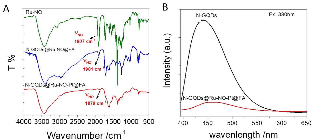
**Figure S1** FTIR spectra of {Ru-NO} (green), {N-GQDs@Ru-NO@FA} (blue), and {N-GQDs@Ru-NO-Pt@FA} (red). (H) Fluorescence spectra of N-GQDs (black line) and nanoplatfrom **1** (red line) in water. Ex: 380 nm.
