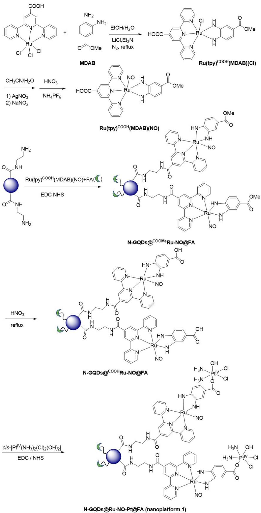
**Scheme S1** Chemical structures and preparation route for the nanoplatform **1**.
