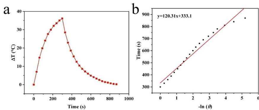
**Figure S3.** (a) Difference in temperature change between BGSs suspension ( $30 \mu\text{g mL}^{-1}$ ) and water irradiated by 808 nm laser at the power density of  $1.5 \text{ W cm}^{-2}$  for 5 min and then the laser was shut off. (b) Linear relationship between  $-\ln(\theta)$  and time.
