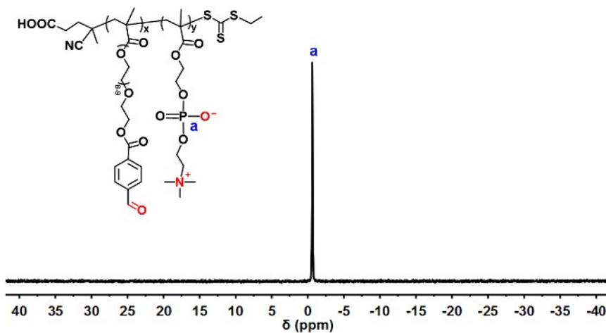
**Figure S4.**  $^{31}\text{P}$  NMR spectrum of P(MPC-co-PEGMA-BZ) random copolymer.
