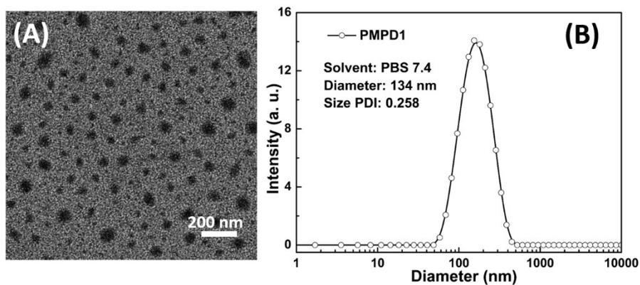
**Figure S9.** TEM image of PMPD1 prodrug nanoparticles (A) and the particle size distribution curve (B) corresponding to the TEM sample (scale bar 200 nm). The concentration was  $0.5 \text{ mg mL}^{-1}$ .
