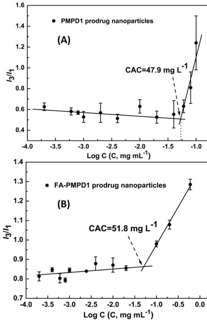
**Figure S8.** Intensity ratios ( $I_3/I_1$ ) as a function of  $\text{Log } C$  for (A) PMPD1 and (B) FA-PMPD1 prodrug nanoparticles in pH 7.4 buffer solution.
