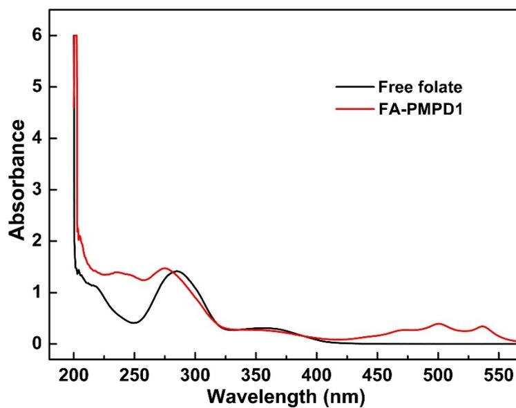
**Figure S7.** UV-vis spectra of free folate and FA-PMPD1 in ethanol.
