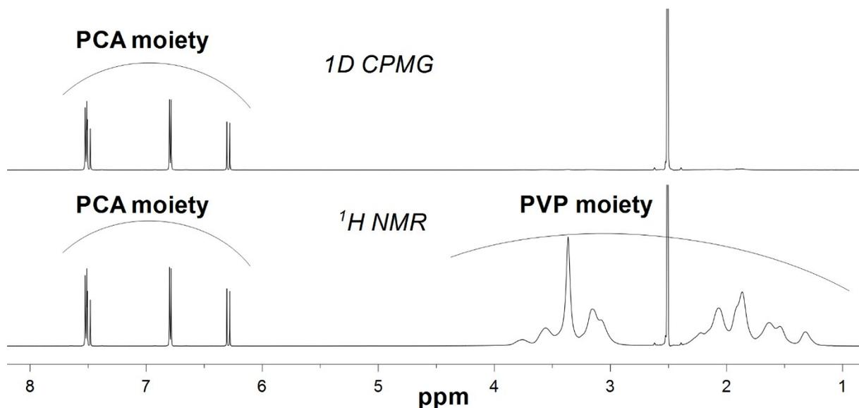
**Figure S4.** <sup>1</sup>H NMR and 1D-CPMG of the PVP/PCA 10:1 sample in DMSO-d<sub>6</sub>. The PVP signals are suppressed after the application of a 1D CPMG acquisition scheme, while the signals of PCA are only slightly decrease in intensity (due to their intrinsic T<sub>2</sub> resonance decay). Analogous results were obtained with all the samples.
