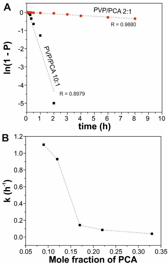
**Figure S5.** **A**, first-order fitting of drug release experiments for PVP/PCA 10:1 and 2:1. The correlation factor  $R$  is included. **B**, calculated kinetic constants as a function of the mole fraction of PCA.
