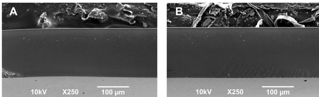
**Figure S2. A, B**, Cross-section SEM images of the PVP/PCA 10:1 and 2:1 samples, respectively.
