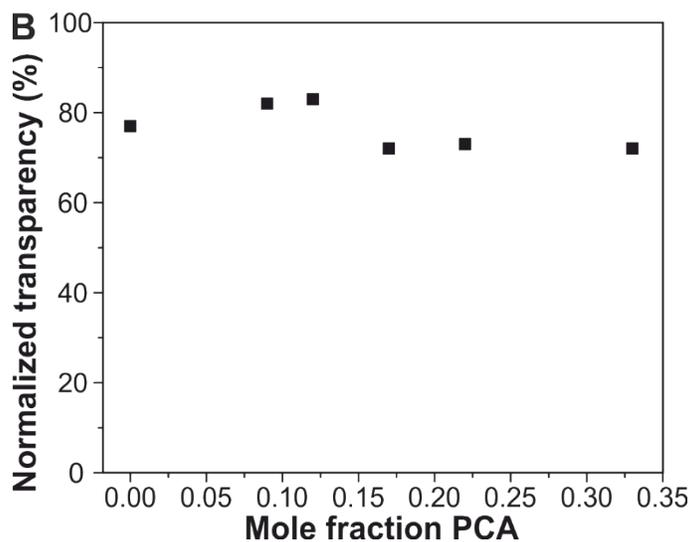
**Figure S1. A**, UV-VIS- spectra in the range 400-800 nm for PVP/PCA 1:0, 2:1, 5:1 and 10:1 samples. **B**, normalized transmittance as a function of the mole fraction of PCA.
