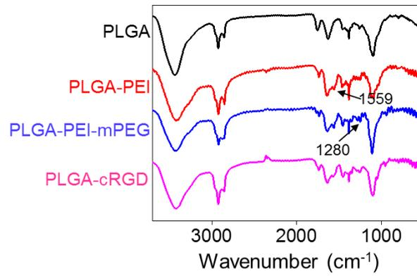
**Figure S2.** The FT-IR spectra of the PLGA, PLGA-PEI, PLGA-PEI-mPEG, and PLGA-cRGD copolymers. The black arrows indicate the amine group (1559 cm<sup>-1</sup>) and the amide group (1280 cm<sup>-1</sup>).
