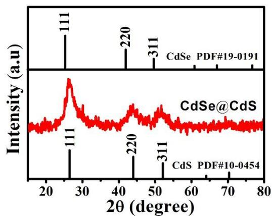
**Figure S1.** The XRD patterns of CdSe@CdS core@shell QDs
