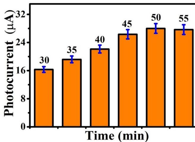
**Figure S10** Photocurrent responses of the PEC biosensor at different incubation time of A $\beta$ -Ab<sub>2</sub> at 0 V (orange columns, 0.1 ng mL<sup>-1</sup> A $\beta$ , error bars=SD (n=5)).
