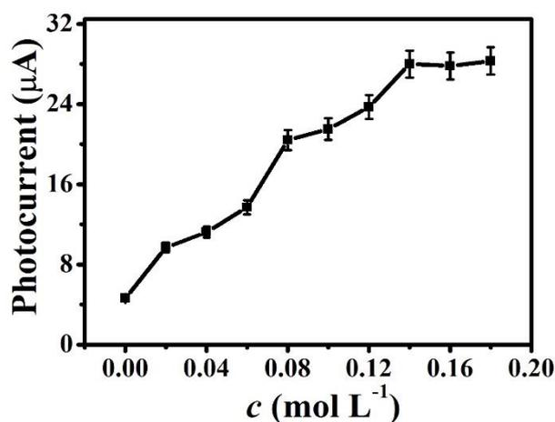
**Figure S3.** Photocurrent responses of the PEC biosensor at different concentration of AA ( $0.1 \text{ ng mL}^{-1} \text{ A}\beta$ , error bars=SD ( $n=5$ )).
