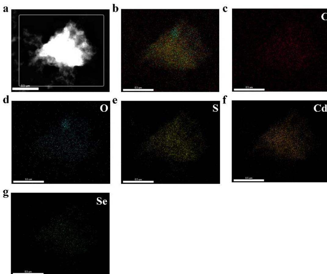
**Figure S2** (a) high-angle annular dark-field scanning TEM; corresponding Energy-dispersive X-ray mapping: (b) merged imagine, (c) C, (d) O, (e) S, (f) Cd and (g) Se
