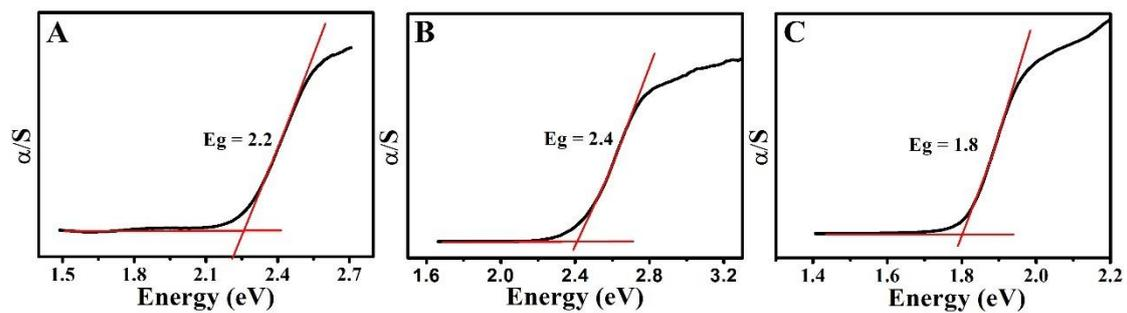
**Figure S5** UV-vis diffuse reflectance spectroscopy of (A)  $\alpha$ - $\text{Fe}_2\text{O}_3$ , (B) CdS and (C) CdSe
