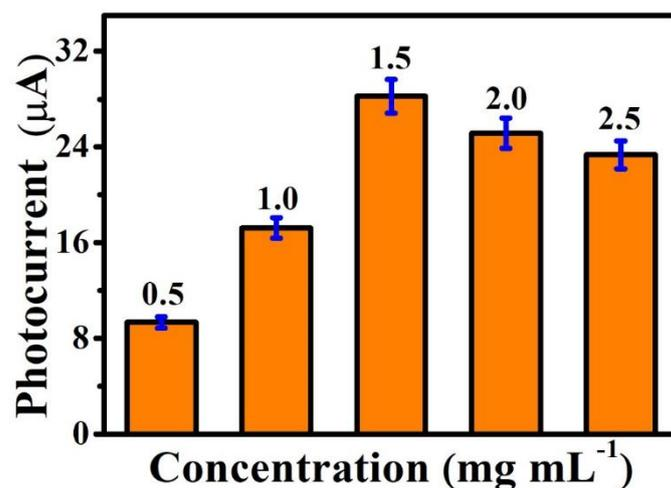
**Figure S8** Photocurrent responses of the PEC biosensor at different concentration of GO/CdSe@CdS QDs at 0 V (orange columns, 0.1 ng mL<sup>-1</sup> A $\beta$ , error bars=SD (n=5)).
