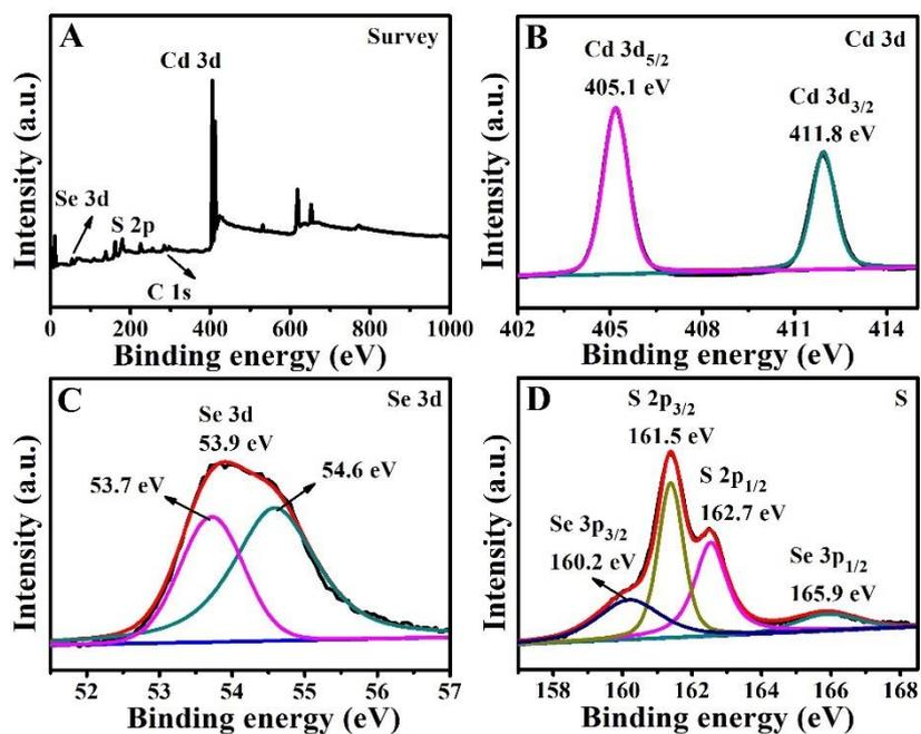
**Figure S4.** XPS survey spectrum of CdSe@CdS QDs composite: (A) survey spectrum; (B) Cd 3d; (C) Se 3d; (D) S 2p.
