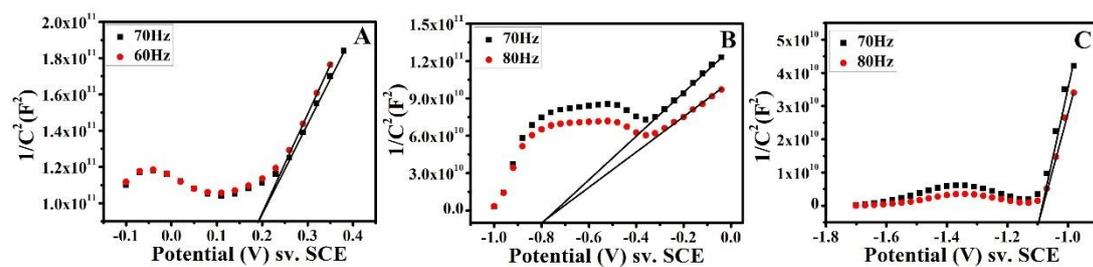
**Figure S6** (A)-(C) Mott-Schottky curves of  $\alpha$ - $\text{Fe}_2\text{O}_3$ , CdS and CdSe in a 0.2 mol/L  $\text{Na}_2\text{SO}_4$  aqueous solution
