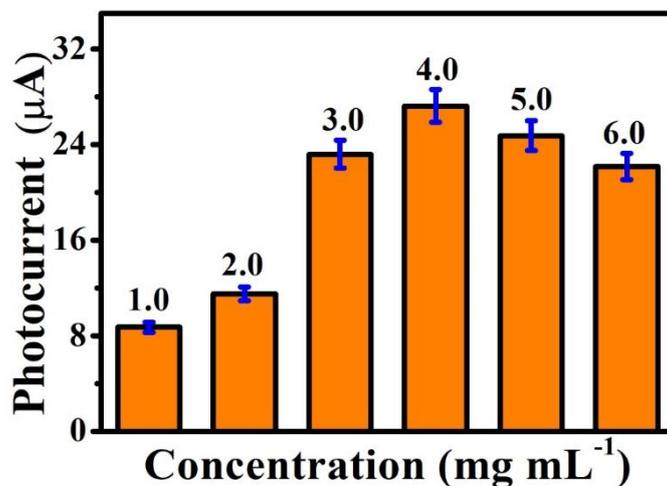
**Figure S7** Photocurrent responses of the PEC biosensor at different concentration of Au NPs/ $\alpha$ -Fe<sub>2</sub>O<sub>3</sub> at 0 V (orange columns, 0.1 ng mL<sup>-1</sup> A $\beta$ , error bars=SD (n=5)).
