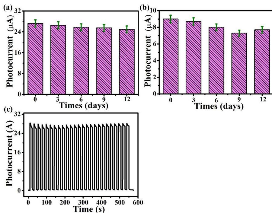
**Figure. S11** (a)  $c_{A\beta} = 0.1 \text{ ng mL}^{-1}$  and (b)  $c_{A\beta} = 0 \text{ ng mL}^{-1}$  the storage stability study of the  $A\beta$  immunosensor, respectively, (c) photocurrent stability evaluation of the PEC immunosensor under several on/off irradiation cycles for 600 s,  $c_{A\beta} = 0.1 \text{ ng mL}^{-1}$
