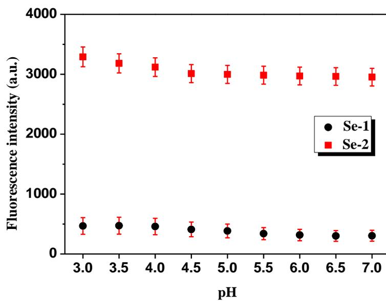
**Figure S7.** Effects of pH on relative fluorescence of Se-1 (10  $\mu\text{M}$ ) and Se-2 (10  $\mu\text{M}$ ) in acetic acid/sodium acetate buffer (20 mM),  $\lambda_{\text{ex}} = 435$  nm.
