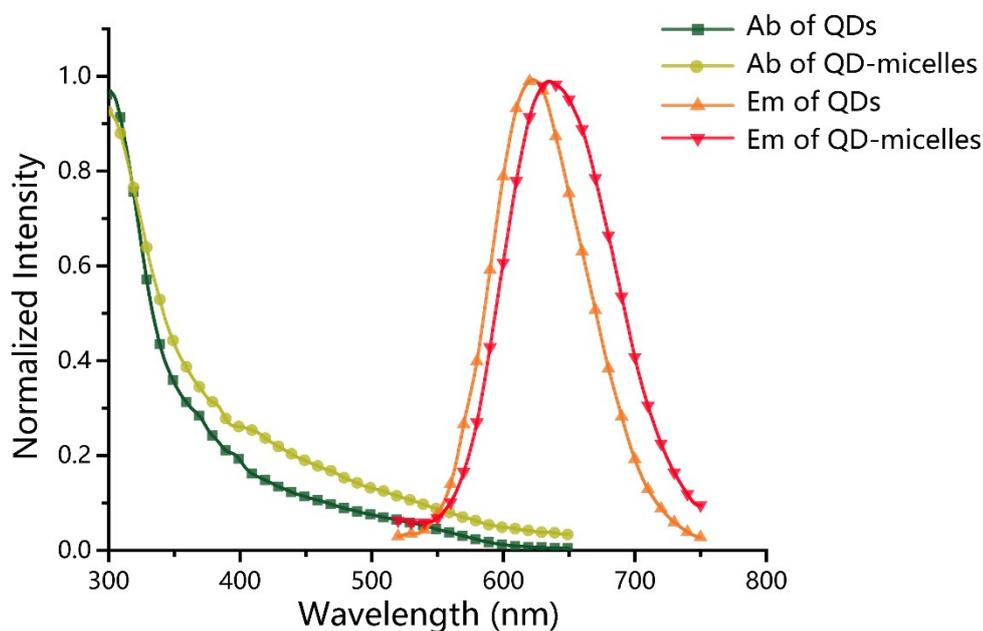
**Figure S1** Absorption (Ab) and emission (Em) spectra of CuInS<sub>2</sub> QDs dispersed in n-hexane (as synthesized) or water (after PS micelle-encapsulation). Both of QDs and QD-micelles were excited at 488nm.
