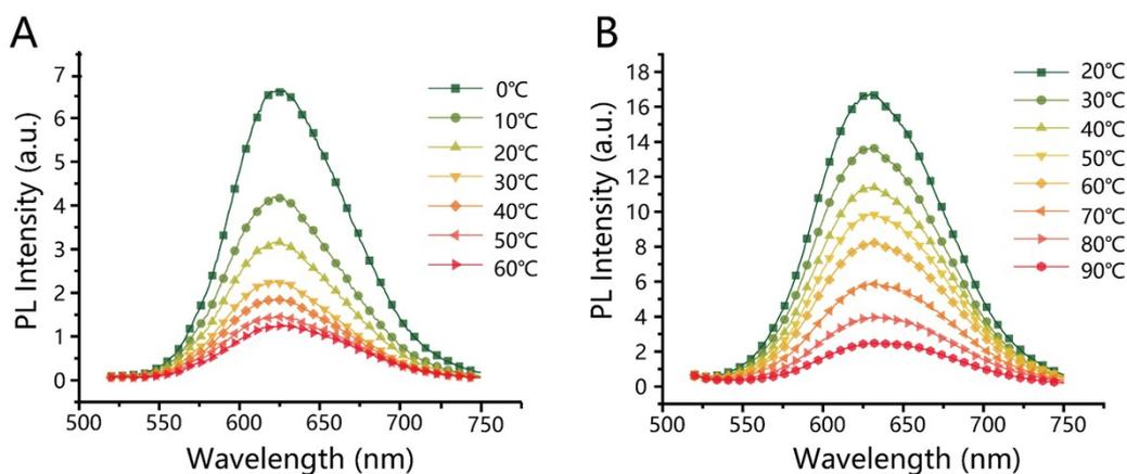
**Figure S4** Temperature-dependent PL emission spectra of CuInS<sub>2</sub>/ZnS QDs in hexane (A) and in octadecene (B).
