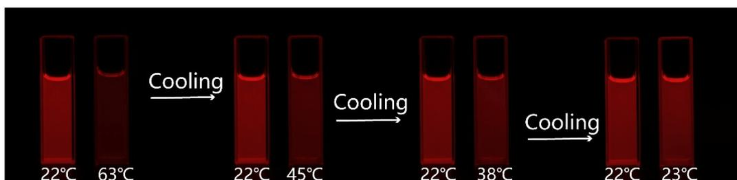
**Figure S3** Fluorescence differences of the heated QD-micelles solution sample (right) and the control (left) as it cooled from 63 °C to 23 °C, under 365 nm UV illumination.
