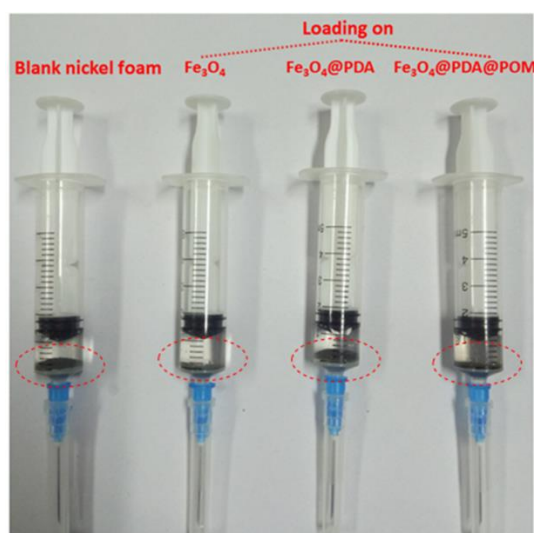
Fig. S6. Nickel foam as the schematic diagram of filter membrane, with asepsis injector as reaction vessel.
