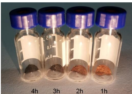
Figure S1. Digital photo of the reduced products of sample S4 at 300 °C for different periods.
