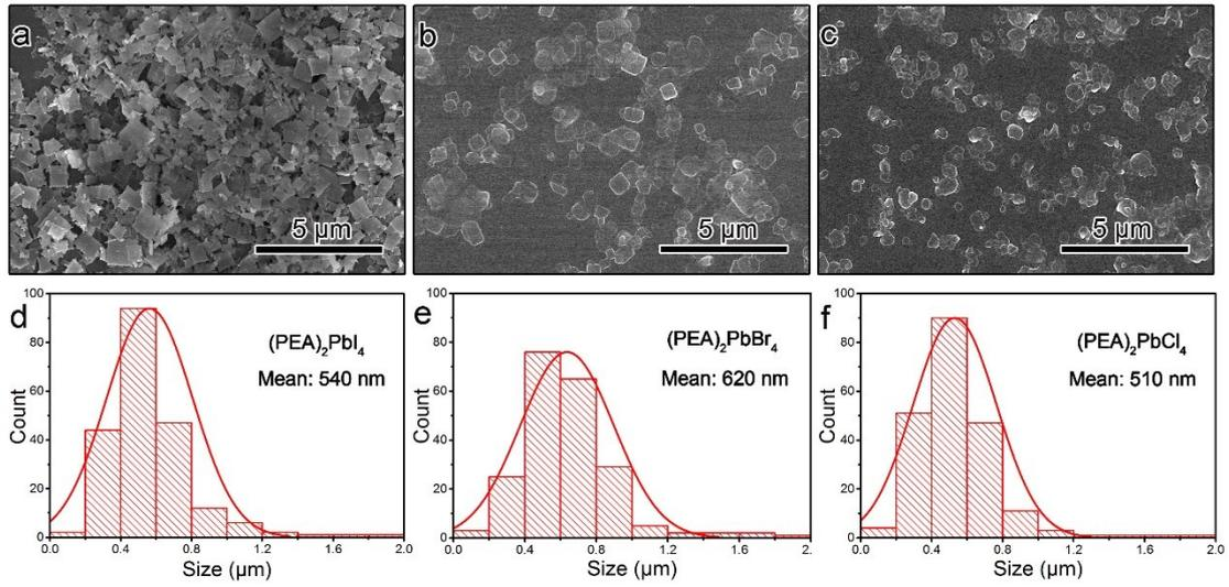
Figure S1. (a) SEM images and (d) the corresponding lateral size distribution of  $(\text{PEA})_2\text{PbI}_4$  NSs. (b) SEM images and (e) the corresponding lateral size distribution of  $(\text{PEA})_2\text{PbBr}_4$  NSs. (c) SEM images and (f) the corresponding lateral size distribution of  $(\text{PEA})_2\text{PbCl}_4$  NSs.
