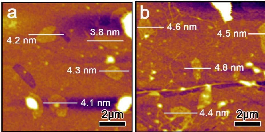
Figure S3. AFM height images and the corresponding thickness of the (a) (PEA)<sub>2</sub>PbBr<sub>4</sub> NSs and (b) (PEA)<sub>2</sub>PbCl<sub>4</sub> NSs.
