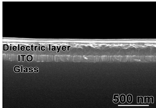
Figure S5. The cross-sectional SEM image of dielectric layer on ITO substrate.
