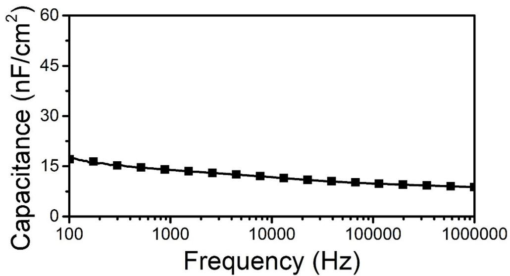
Figure S6. Capacitance vs frequency for characteristic with a capacitor area of 0.00125
