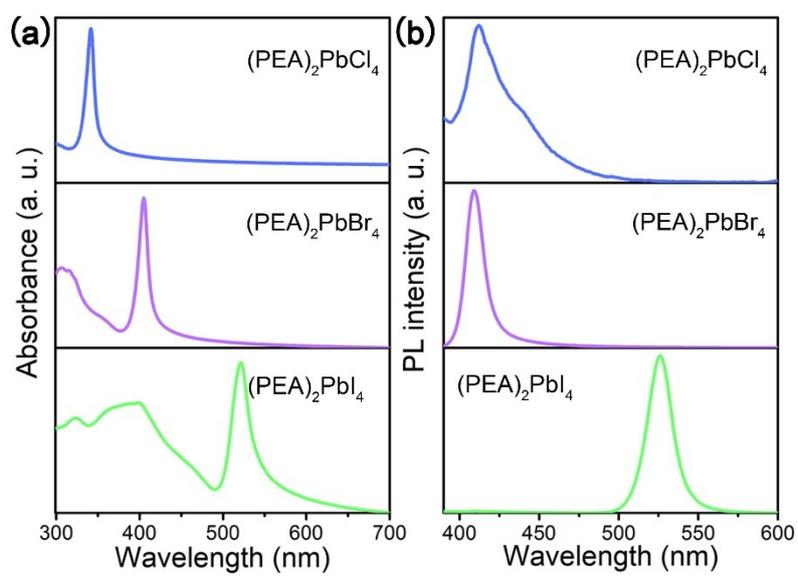
Figure S2. (a) UV/Vis absorption and (b) photoluminescence (PL) spectra of  $(\text{PEA})_2\text{PbX}_4$  NSs (X= Cl, Br, I).
