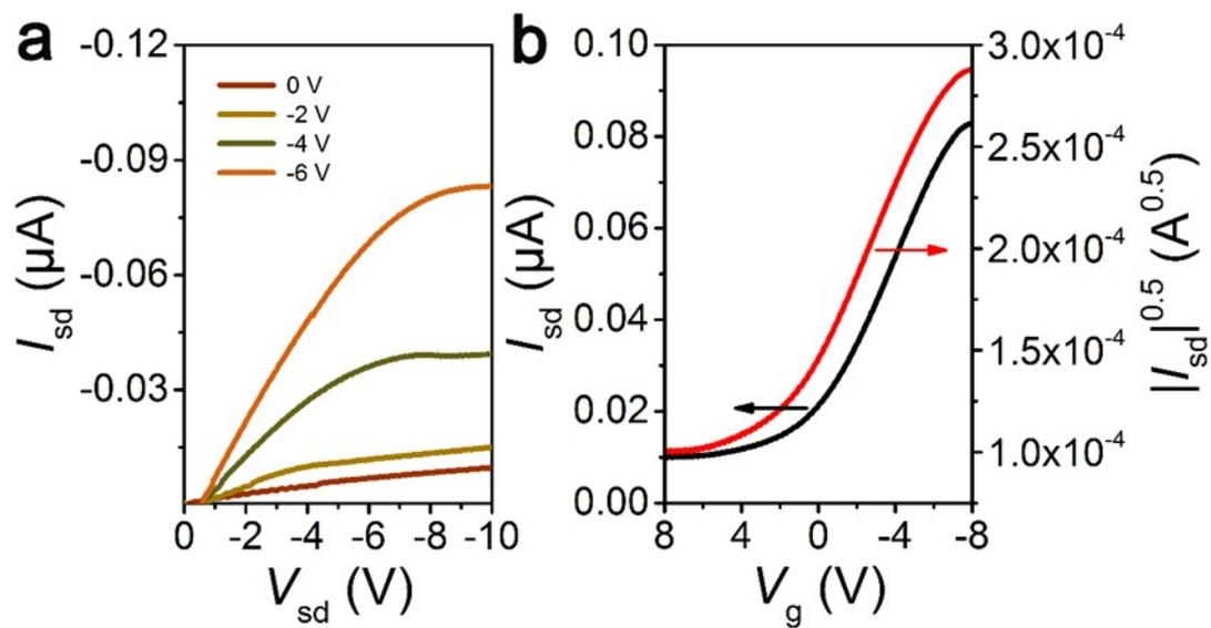
Figure S7. (a) Output and (b) transfer characteristics of a representative *p*-channel FET with P3HT.
