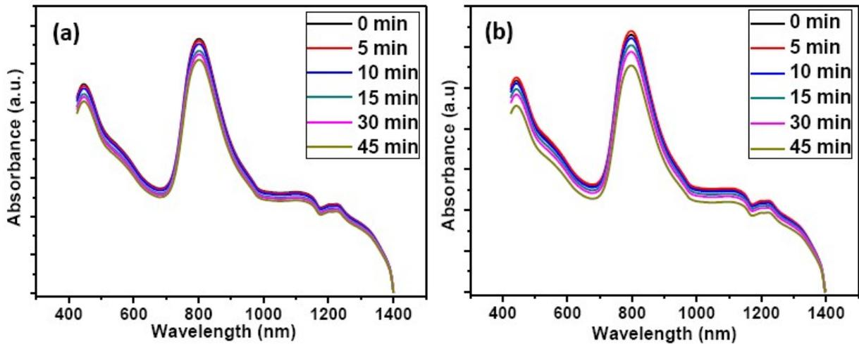
**Fig. S23.** Absorption spectra of (a) water-dispersible IR-1061 dye alone and (b) water-dispersible IR-1061 dye +  $\text{NaYF}_4:\text{Tm}^{3+}(0.5)/\text{Yb}^{3+}(30)@\text{NaYF}_4:\text{Yb}^{3+}(10)$  UCNPs at different time intervals. ( $\lambda_{\text{ex}} = 980 \text{ nm}$  laser,  $7 \text{ W}/\text{cm}^2$ ).
