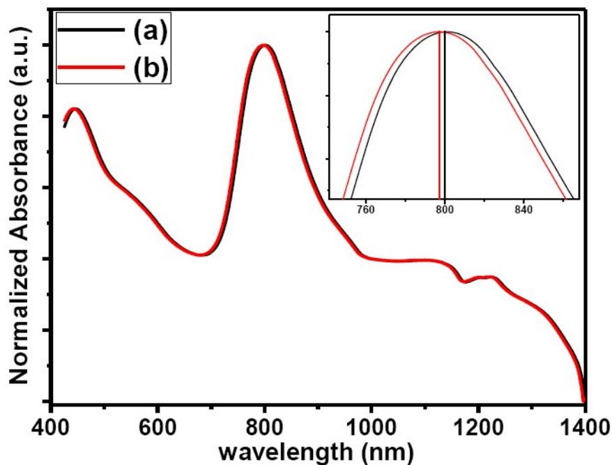
**Fig. S19.** Absorption spectra of (a) water-dispersible IR-1061 dye alone and (b) dye attached to core/active shell UCNP.
