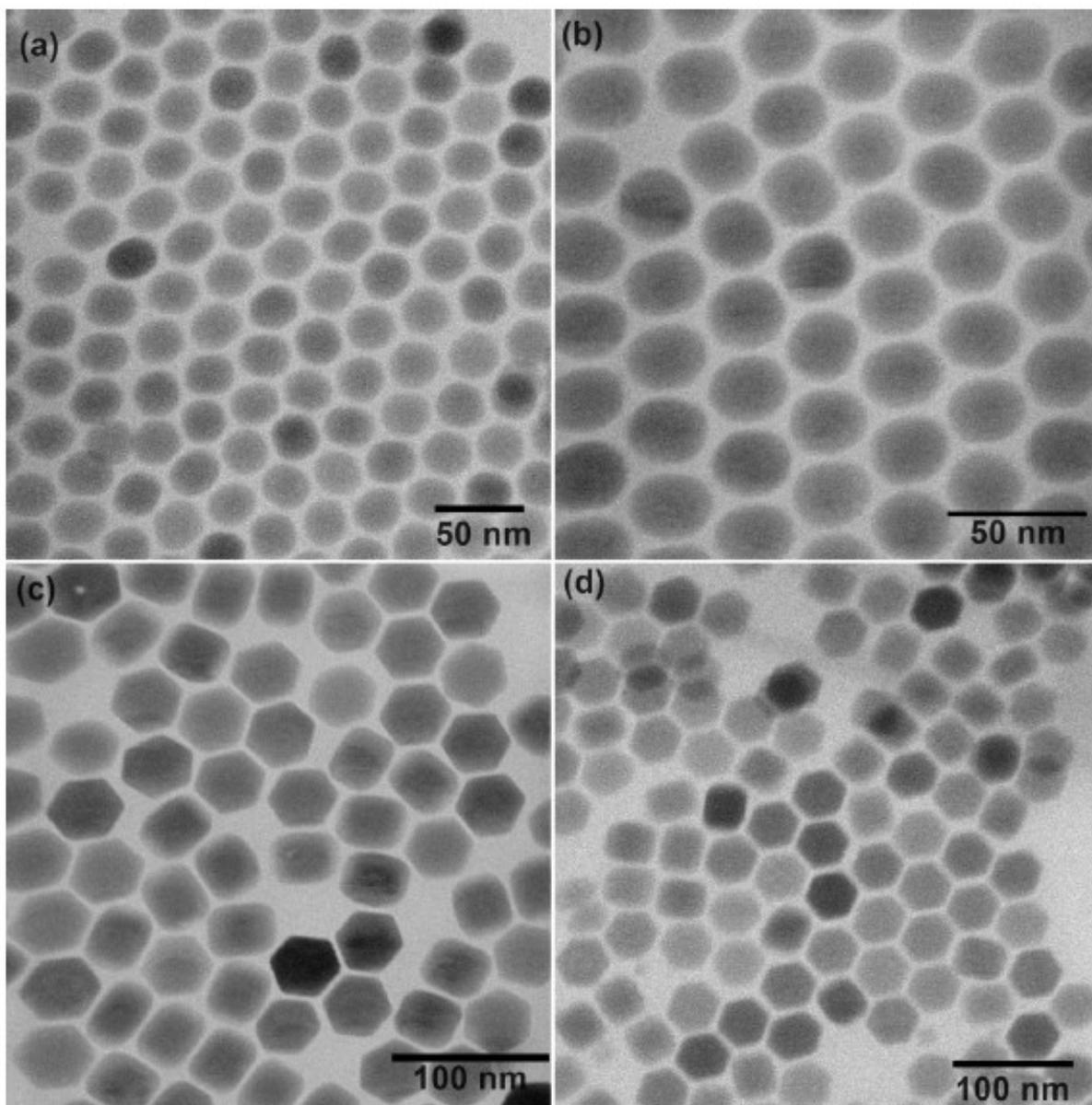
**Fig. S2.** TEM images of oleic acid capped (a) core and (c) corresponding  $\text{NaYF}_4:\text{Tm}^{3+}(0.5)/\text{Yb}^{3+}(30)@\text{NaYF}_4:\text{Yb}^{3+}(2)$  UCNPs; (b) core and (d) corresponding  $\text{NaYF}_4:\text{Tm}^{3+}(0.5)/\text{Yb}^{3+}(30)@\text{NaYF}_4:\text{Yb}^{3+}(20)$  UCNPs.
