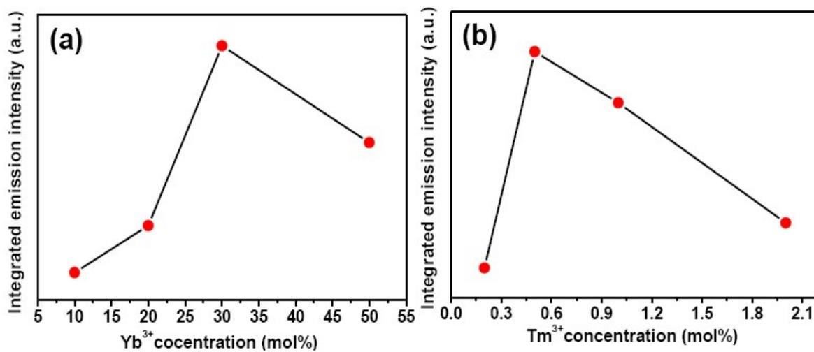
**Fig. S5.** Plot of Integrated upconversion emission intensity against (a)  $\text{Yb}^{3+}$  and (b)  $\text{Tm}^{3+}$  concentration (in mol %) in oleic acid capped core UCNPs.
