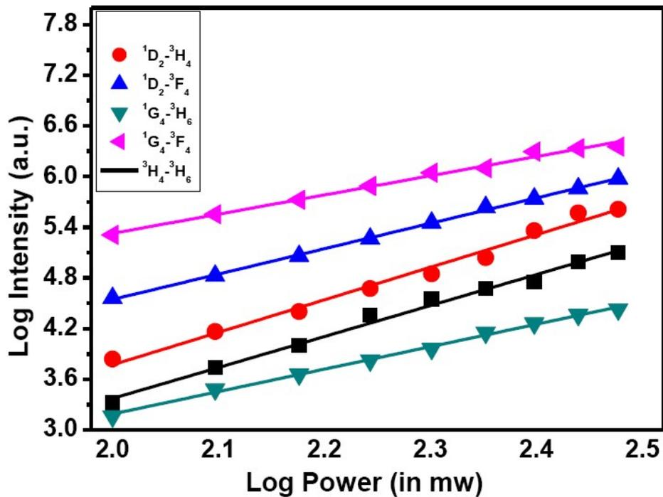
**Fig. S7.** Power dependence graph of the different transitions of Tm<sup>3+</sup> ion in NaYF<sub>4</sub>:Tm<sup>3+</sup>(0.5)/Yb<sup>3+</sup>(30)@NaYF<sub>4</sub>:Yb<sup>3+</sup>(10) UCNPs excited at 980 nm.
