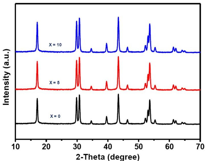
**Fig. S13.** PXRD of PEI capped NaYF<sub>4</sub>:Tm<sup>3+</sup>(0.5)/Yb<sup>3+</sup>(30)@NaYF<sub>4</sub>:Yb<sup>3+</sup>(X) (X= 0, 5, 10) UCNPs. All peaks are well matched with standard hexagonal NaYF<sub>4</sub> crystals (JCPDS No: 28-1192).
