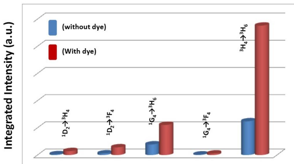
**Fig. S20.** Bar diagram indicating enhancement in upconversion emission from different states of  $Tm^{3+}$  ions of  $NaYF_4:Tm^{3+}(0.5)/Yb^{3+}(30)@NaYF_4:Yb^{3+}(10)$  UCNPs in the presence and absence of dye sensitization.
