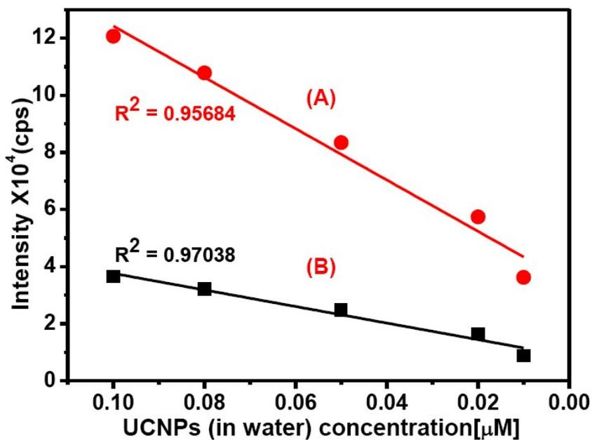
**Fig. S25.** Linear plots between UC emission spectra of water-dispersible IR-1061 dye-sensitized (A) NaYF<sub>4</sub>:Yb<sup>3+</sup>(30)/Tm<sup>3+</sup>(0.5%)@NaYF<sub>4</sub>:Yb<sup>3+</sup>(0) and (B) NaYF<sub>4</sub>:Yb<sup>3+</sup>(30)/Tm<sup>3+</sup>(0.5%)@NaYF<sub>4</sub>:Yb<sup>3+</sup>(10) core/active shell UCNPs against dilution of the same.
