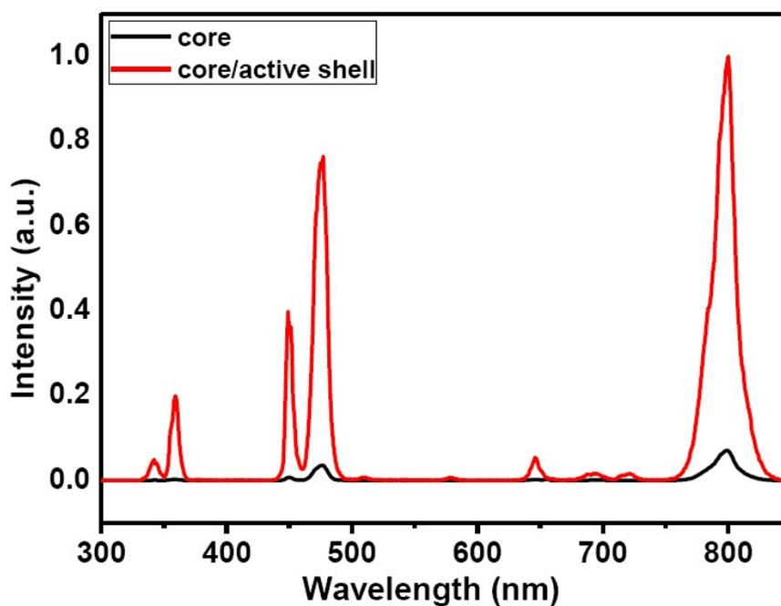
**Fig. S9.** Upconversion emission comparison between  $\text{NaYF}_4:\text{Tm}^{3+}(0.5)/\text{Yb}^{3+}(40)$  core and  $\text{NaYF}_4:\text{Tm}^{3+}(0.5)/\text{Yb}^{3+}(30)@\text{NaYF}_4:\text{Yb}^{3+}(10)$  core/active shell UCNPs.
