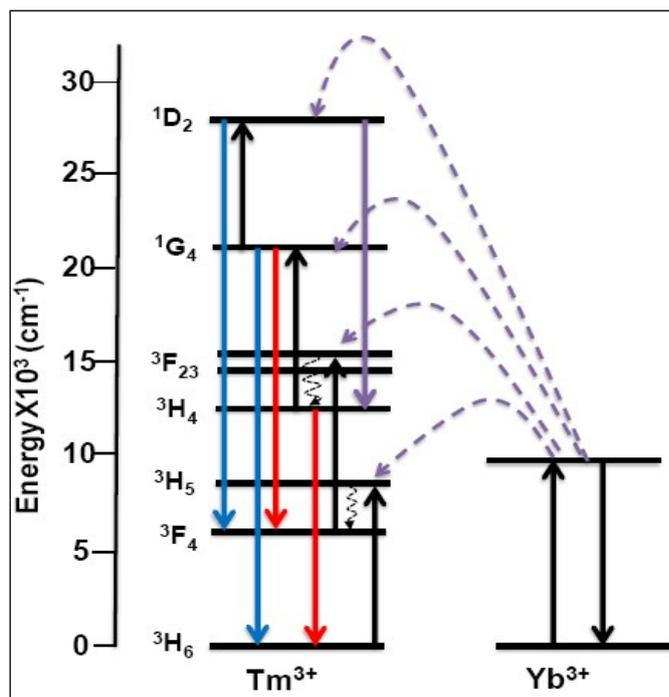
**Fig. S8.** Energy transfer mechanism occurring in between  $\text{Tm}^{3+}$  ion and  $\text{Yb}^{3+}$  ion in  $\text{NaYF}_4:\text{Tm}^{3+}(0.5)/\text{Yb}^{3+}(30)@\text{NaYF}_4:\text{Yb}^{3+}(10)$  UCNPs.
