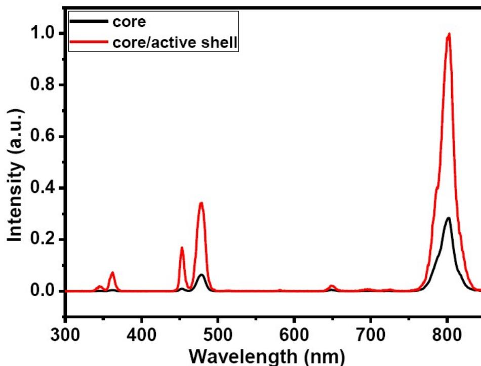
**Fig. S21.** Upconversion emission comparison between water-dispersible IR-1061 dye-sensitized  $NaYF_4:Tm^{3+}(0.5)/Yb^{3+}(40)$  core and  $NaYF_4:Tm^{3+}(0.5)/Yb^{3+}(30)@NaYF_4:Yb^{3+}(10)$  core/active shell UCNPs.
