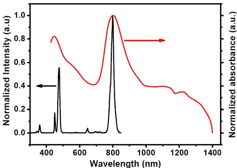
**Fig. S16.** Overlap between absorption of water dispersible IR-1061 dye (red) and upconversion emission of water-dispersible  $\text{NaYF}_4:\text{Tm}^{3+}(0.5)/\text{Yb}^{3+}(30)@\text{NaYF}_4:\text{Yb}^{3+}(10)$  UCNPs (black).
