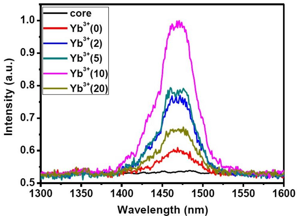
**Fig. S11.** Downshifting emission spectra of oleic acid capped  $\text{NaYF}_4:\text{Tm}^{3+}(0.5)\text{Yb}^{3+}(30)$  core and  $\text{NaYF}_4:\text{Tm}^{3+}(0.5)\text{Yb}^{3+}(30)@\text{NaYF}_4:\text{Yb}^{3+}(X)$  ( $X = 0, 2, 5, 10, 20$ ) core/active shell UCNPs in cyclohexane under 980 nm laser excitation at  $7\text{W}/\text{cm}^2$ .
