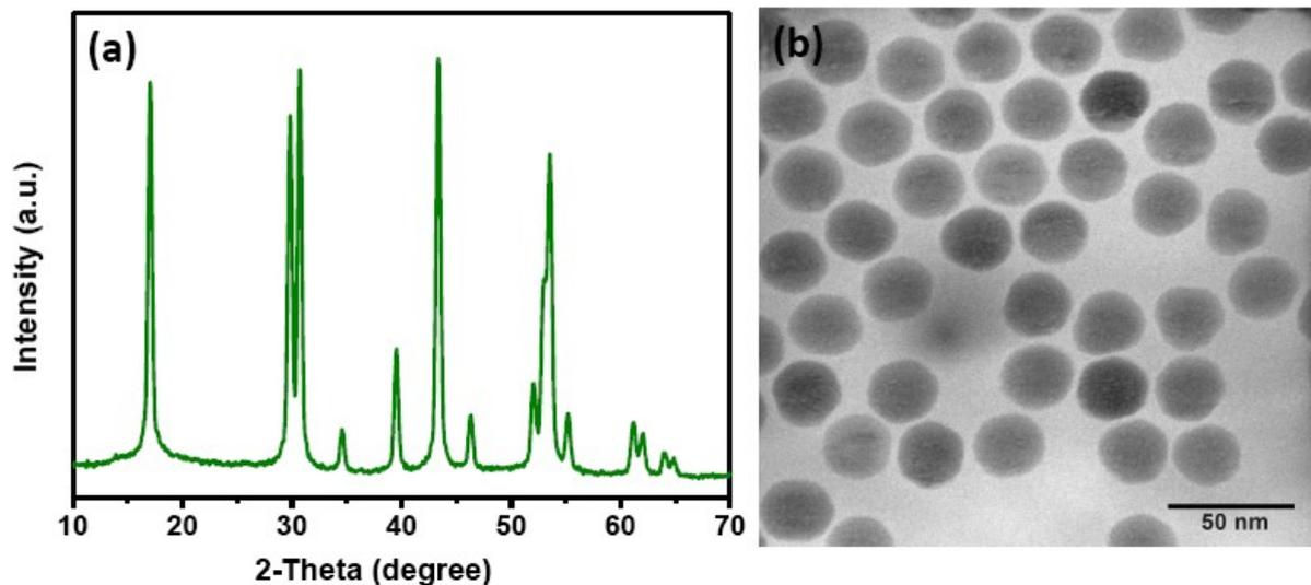
**Fig. S10.** (a) PXRD and (b) TEM image of  $\text{NaYF}_4:\text{Yb}^{3+}(40)/\text{Tm}^{3+}(0.5)$  core UCNPs.
