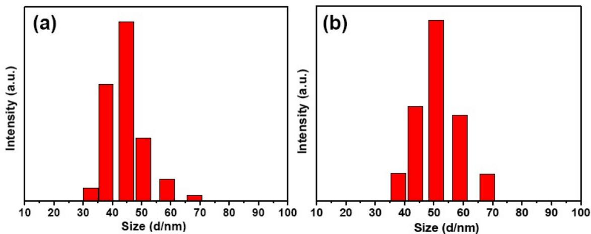
**Fig. S18.** Size distribution (by DLS) of water-dispersible  $\text{NaYF}_4:\text{Tm}^{3+}(0.5)/\text{Yb}^{3+}(30)@\text{NaYF}_4:\text{Yb}^{3+}(10)$  UCNP in (a) absence and (b) presence of water dispersible IR-1061 dye.
