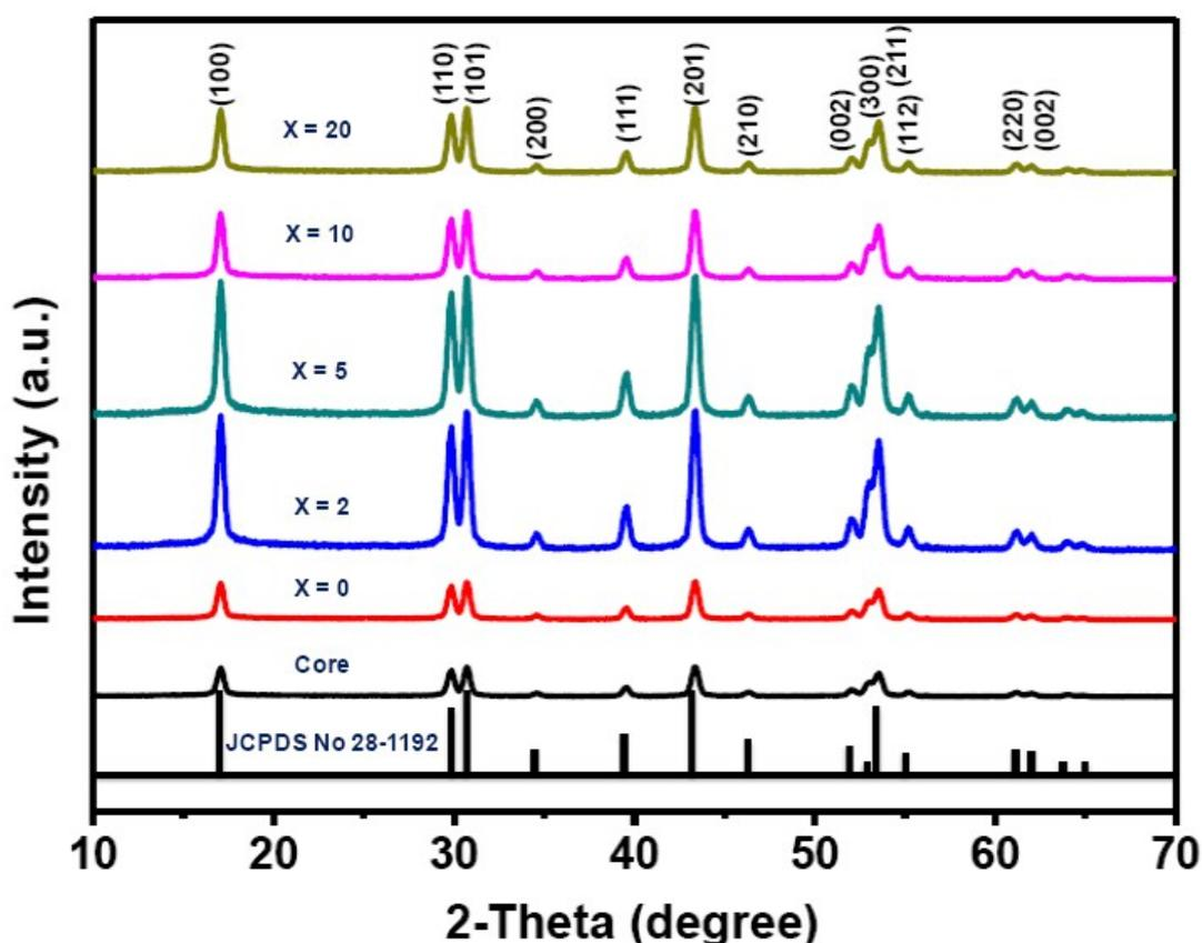
**Fig. S1.** PXRD of oleic acid capped  $\text{NaYF}_4:\text{Tm}^{3+}(0.5)/\text{Yb}^{3+}(30)$  core and  $\text{NaYF}_4:\text{Tm}^{3+}(0.5)/\text{Yb}^{3+}(30)@\text{NaYF}_4:\text{Yb}^{3+}$  ( $X=0, 2, 5, 10, 20$ ) core/active shell UCNPs. All peaks match well with the diffraction peaks of standard hexagonal  $\text{NaYF}_4$  crystals (JCPDS No: 28-1192).
