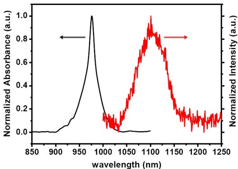
**Fig. S17.** Overlap spectra between PL emission of water-dispersible IR-1061 dye (red) and absorption of water-dispersible  $\text{NaYF}_4:\text{Tm}^{3+}(0.5)/\text{Yb}^{3+}(30)@\text{NaYF}_4:\text{Yb}^{3+}(10)$  UCNPs (black) ( $\lambda_{\text{ex}} = 980 \text{ nm}$  laser,  $7 \text{ W/cm}^2$ ).
