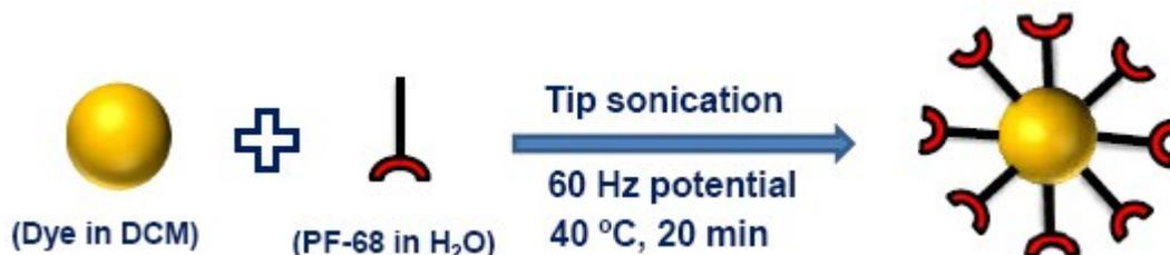
**Scheme:** Scheme illustrating the preparation of water dispersible IR-1061 dye. We synthesized water-dispersible IR-1061 dye using tip sonication via phase transfer process.
