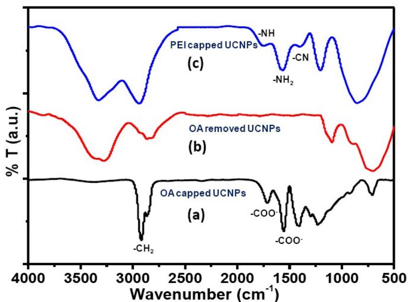
**Fig. S12.** FTIR spectra of (a) oleic acid (OA) capped NaYF<sub>4</sub>:Tm<sup>3+</sup>(0.5)Yb<sup>3+</sup>(30)@NaYF<sub>4</sub>:Yb<sup>3+</sup>(10) (b) oleic acid (OA) removed NaYF<sub>4</sub>:Tm<sup>3+</sup>(0.5)Yb<sup>3+</sup>(30)@NaYF<sub>4</sub>:Yb<sup>3+</sup>(10) (core/active shell UCNPs and (c) PEI capped NaYF<sub>4</sub>:Tm<sup>3+</sup>(0.5)Yb<sup>3+</sup>(30)@NaYF<sub>4</sub>:Yb<sup>3+</sup>(10).
