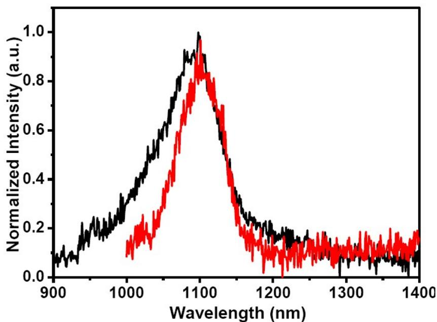
**Fig. S15.** PL emission spectra of water-dispersible IR-1061 dye using 980 nm (red) and 808 nm (black) laser excitation at  $7 \text{ W/cm}^2$ .
