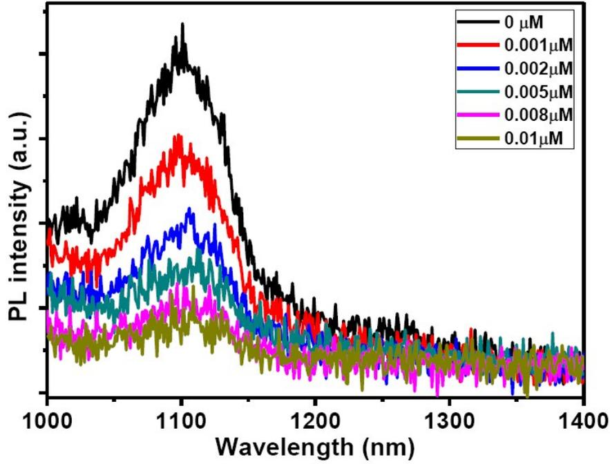
**Fig. S22.** PL emission of IR-1061 dye in water against different concentration of water-dispersible  $\text{NaYF}_4:\text{Tm}^{3+}(0.5)/\text{Yb}^{3+}(30)@\text{NaYF}_4:\text{Yb}^{3+}(10)$  UCNPs. ( $\lambda_{\text{ex}} = 980 \text{ nm}$  laser,  $7\text{W}/\text{cm}^2$ ,  $[\text{IR-1061 dye}] = 0.6 \mu\text{M}$ .)
