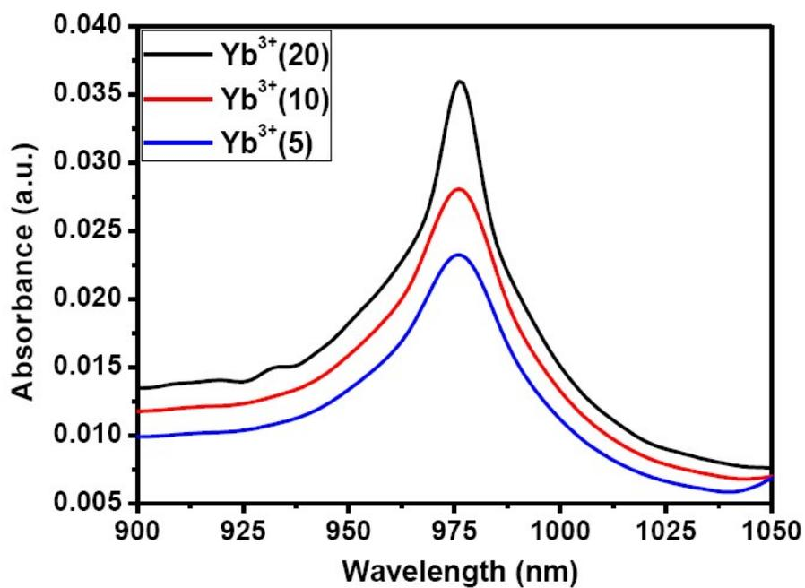
**Fig. S4.** Absorption spectra of  $\text{NaYF}_4:\text{Tm}^{3+}(0.5)/\text{Yb}^{3+}(30)@\text{NaYF}_4:\text{Yb}^{3+}(\text{X})$  ( $\text{X}= 5, 10, 20$ ) UCNPs.
