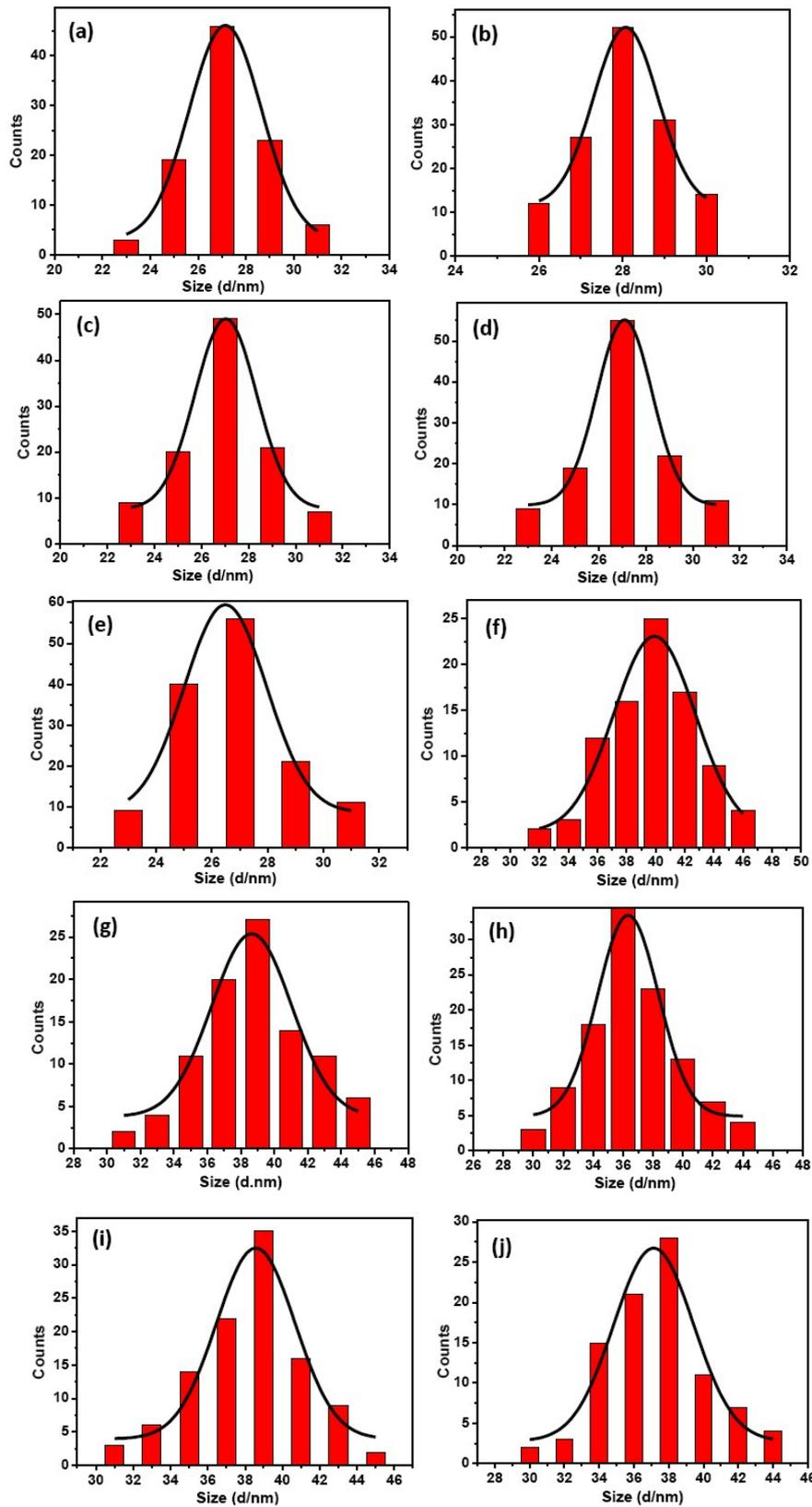
**Fig. S3.** The size distribution of  $\text{NaYF}_4:\text{TM}^{3+}(0.5)/\text{Yb}^{3+}(30)$  core and  $\text{NaYF}_4:\text{TM}^{3+}(0.5)/\text{Yb}^{3+}(30)@\text{NaYF}_4:\text{Yb}^{3+}(X)$  ( $X = 0, 2, 5, 10, 20$ ) core/shell UCNPs. [a-core, f-core/shell ( $X = 0$ ); b-core, g- core/shell ( $X = 2$ ); c-core, h- core/shell ( $X = 5$ ); d-core, i- core/shell ( $X = 10$ ); e-core, j- core/shell ( $X = 20$ )];
