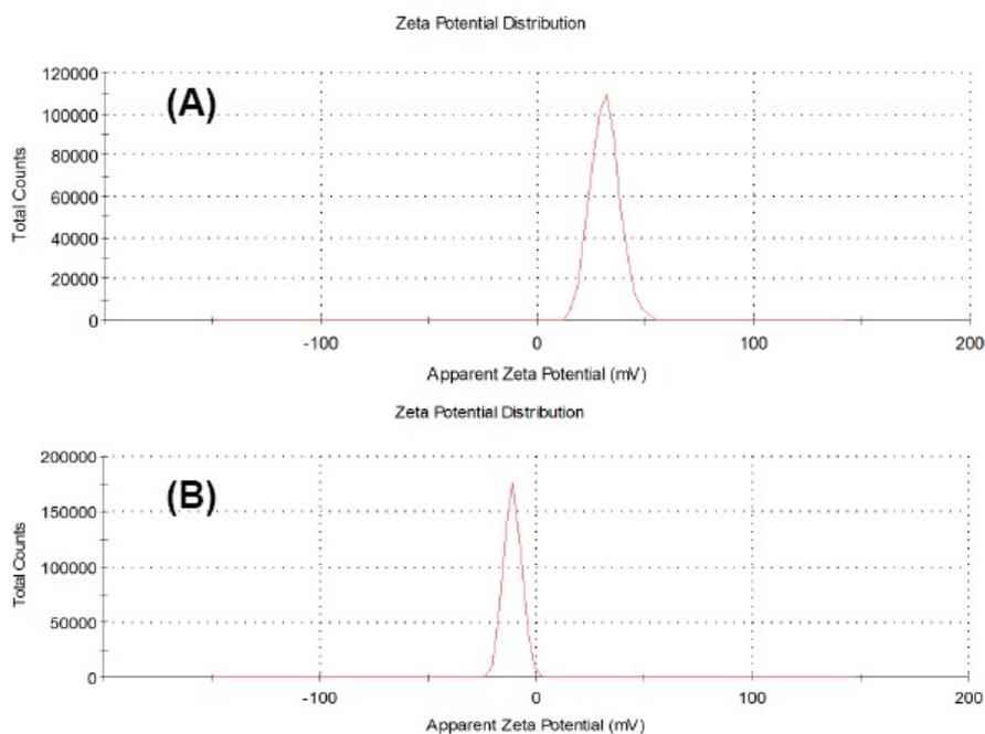
**Fig. S14.** Zeta potential graphs of (A) PEI capped  $\text{NaYF}_4:\text{Tm}^{3+}(0.5)/\text{Yb}^{3+}(30)@\text{NaYF}_4:\text{Yb}^{3+}(10)$  UCNP and (B) Pluronic F68 encapsulated IR-1061 dye.
