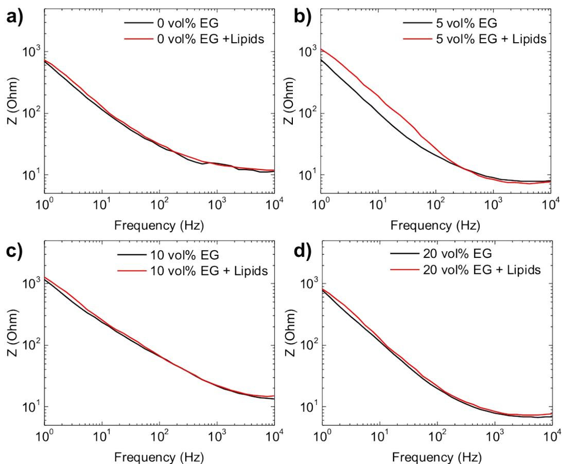
**Figure S3.** Electrochemical impedance spectra recorded in PBS at  $V = -0.05V$  vs.  $V_{oc}$  for PEDOT:PSS coated  $SiO_2$  sensors with (red lines) and without lipid layers (black lines). From a to d, PEDOT:PSS films were cast from dispersions containing 0, 5, 10 and 20 vol% EG, respectively.
