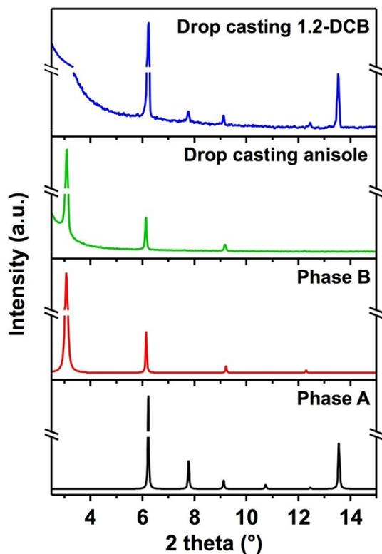
**Figure S4.** XRD patterns of the C<sub>6</sub>-NT4N thin films deposited on Cytop by drop casting from 1,2-DCB (blue line) and anisole (green line) solution, and calculated diffractograms of A (black line) and B (red line) phases.
