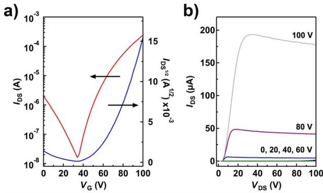
**Figure S3.** (a) Transfer and (b) output characteristics measured at positive source-drain bias of a representative field-effect transistor based on  $C_6$ -NT4N film deposited by thermal sublimation (bottom gate/top contact configuration, drain voltage  $V_{SD} = 100$  V).
