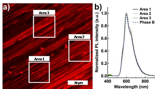
**Figure S5.** (a) Confocal fluorescence image and (b) localized emission spectra ( $\lambda_{\text{ex}} = 405 \text{ nm}$ ) of C<sub>6</sub>-NT4N microstripes deposited on Cytop by LCW from 1,2-DCB solution. PL spectrum of C<sub>6</sub>-NT4N thin film deposited by thermal sublimation (phase B) is reported as comparison (blue dashed line).
