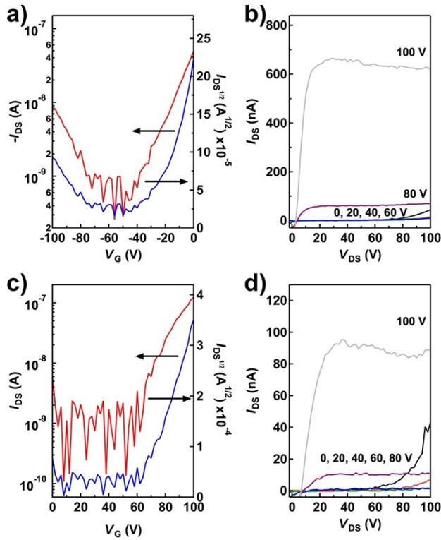
**Figure S2.** Transfer and output characteristics of representative field-effect transistors based on  $C_6$ -NT4N films deposited by LCW from (a, b) anisole and (c, d) 1,2-DCB solution (drain voltage  $V_{SD} = \pm 100$  V).
