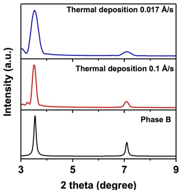
**Figure S1.** XRD patterns of C<sub>4</sub>-NT4N thin film on HMDS-treated Si/SiO<sub>2</sub> deposited by thermal sublimation at 0.1 Å/s (red line) and 0.017 Å/s (blue line) and theoretical X-ray diffractogram of C<sub>4</sub>-NT4N phase B (black line).
