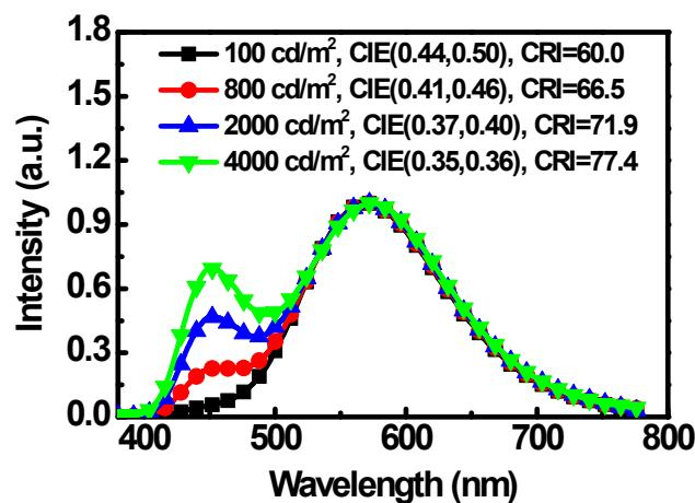
**Figure S6.** EL spectra of WOLED without the TSPO1 buffer layer at different luminance.
