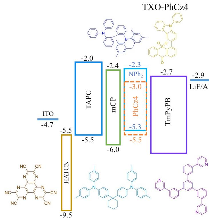
**Figure S5.** Molecular structures and energy levels of WOLEDs based on bi-component TADF EML with simple structure.
