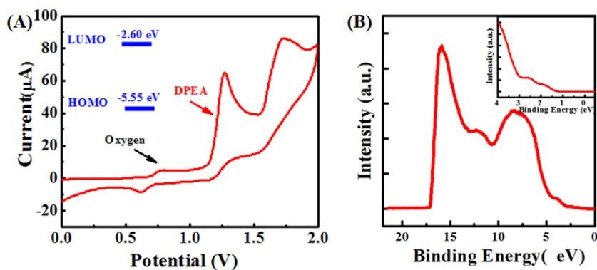
**Figure S1.** (A) Cyclic voltammogram measurement of DPEA in the acetonitrile solution. (B) UPS Energy distribution curve of DPEA thin films.  $\text{HOMO} = h\nu + E_{\text{cutoff}} - E_{\text{F}}$ ,  $h\nu = 21.22 \text{ eV}$ .
