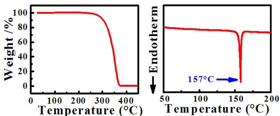
**Figure S2.** Thermal gravimetric analysis and differential scanning calorimetry of DPEA.
