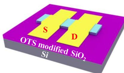
**Figure S5.** Schematic of the DPEA single-crystal-based transistor with bottom-gate top-contact configuration.
