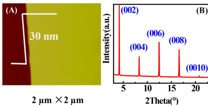
**Figure S6.** (A) AFM image of DPEA crystal prepared by physical vapor transport. (B) XRD diffractions of DPEA crystals on OTS-modified Si/SiO<sub>2</sub> substrate.
