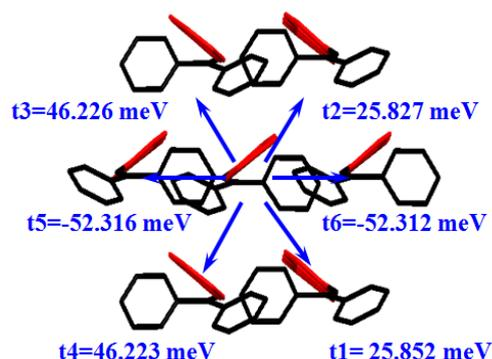
**Figure S3.** Illustrations of transfer integrals for the nearest neighboring molecular pairs considered in the calculations for the DPEA crystal based on the direct integration with site-energy correction.
