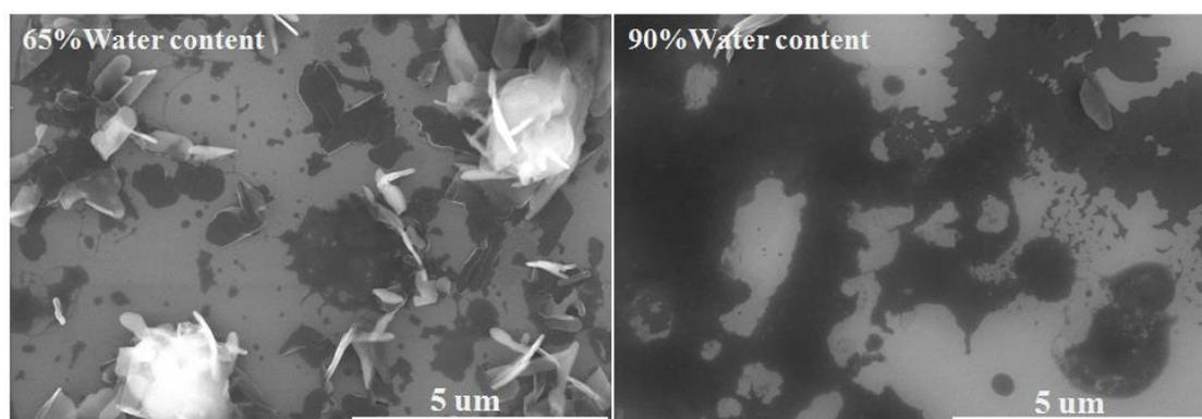
**Figure S4.** SEM images of DPEA aggregations in the mixture solutions with water contents of 65% and 90%, respectively.
