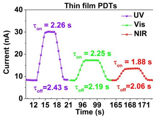
**Figure S13** Enlarged portions of one response and reset process of [60]PCBM thin film devices under dark and illuminated by UV, Vis and NIR lasers.
