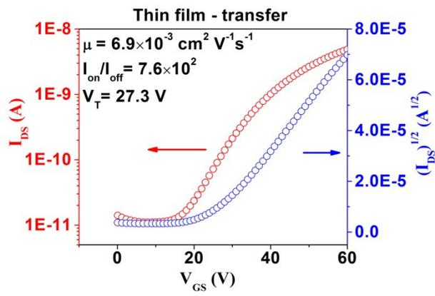
**Figure S5** Typical transfer characteristics of thin film device in n-channel operation mode under positive drain bias.
