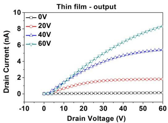
**Figure S6** Typical output characteristics of thin-film device in n-channel operation mode under positive drain bias.
