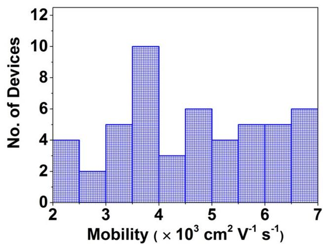
**Figure S7** Histogram of electron mobility calculated from 50 OFETs based on PCBM thin films.
