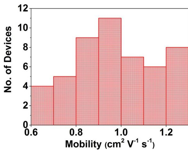
**Figure S2** Histogram of electron mobility calculated from 50 OFETs based on [60]PCBM single crystals.
