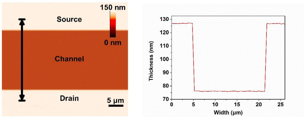
**Figure S4** AFM image and selected area roughness analysis of OFET device based on [60]PCBM thin films.
