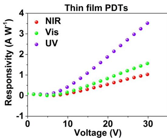
**Figure S11** Responsivity of [60]PCBM thin film devices under dark and illuminated by UV, Vis and NIR lasers.
