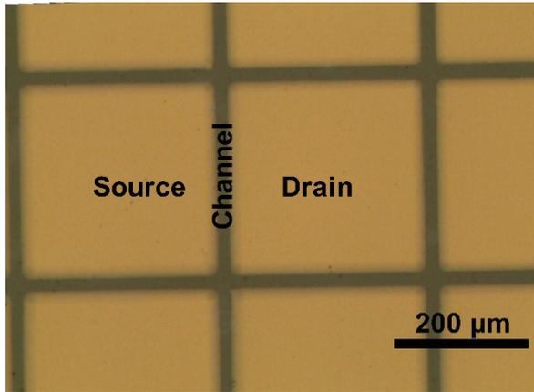
**Figure S3** OM image of OFET device based on [60]PCBM thin films.
