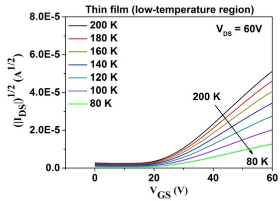
**Figure S9** Transfer characteristics of thin film devices in n-channel operation mode at the temperature from 200K to 80K.
