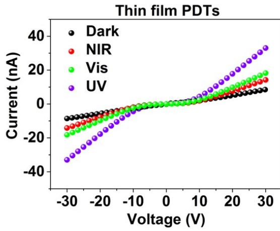
**Figure S10** I–V curves of [60]PCBM thin film devices under dark and illuminated by UV, Vis and NIR lasers.
