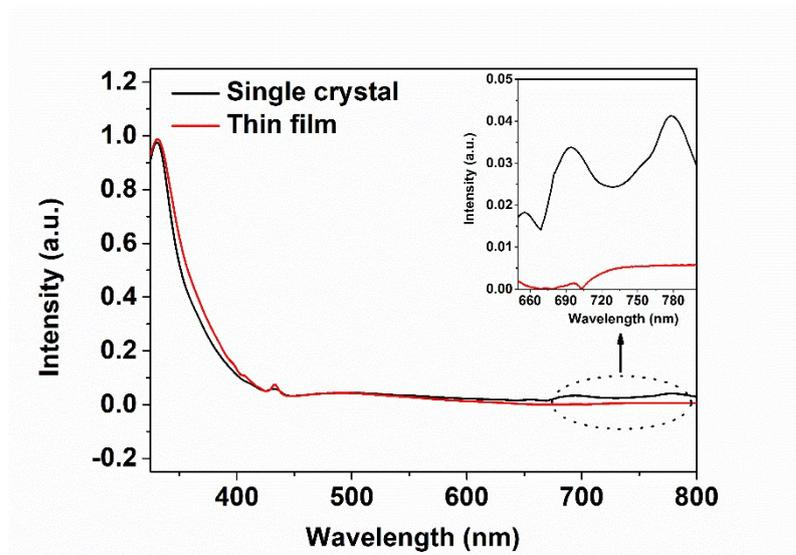
**Figure S14** UV-Vis spectra of [60]PCBM single crystals and thin films.
