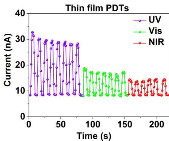
**Figure S12** Time-resolved photocurrent response of [60]PCBM thin film devices under dark and illuminated by UV, Vis and NIR lasers.
