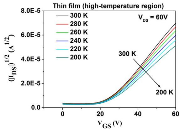
**Figure S8** Transfer characteristics of thin film devices in n-channel operation mode at the temperature from 300K to 200K.
